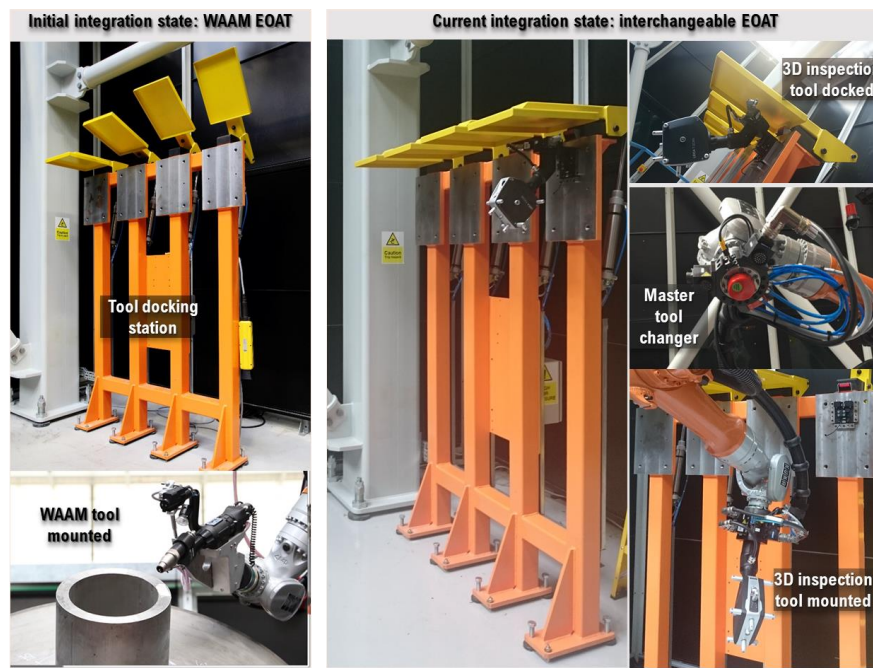
Figure 4-15: Implementation of tool docking station to support multi-EOAT concept for BAM applications.
