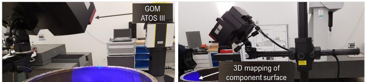
Figure 5-28: 3D geometric inspection and DAQ procedures.
