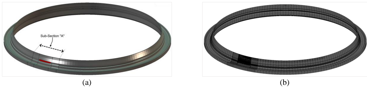
Figure 6-24. (a) Defeatured artefact model section with representative groove, showing sub-section “A”, and (b) artefact model section mesh.
