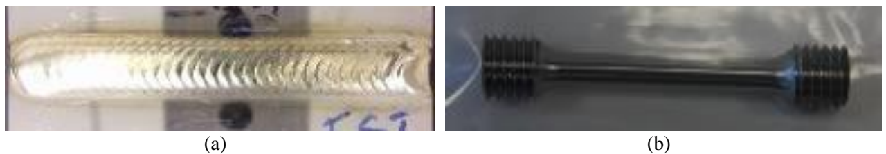
Figure 5-20: (a) Material extracted from restored BAM sample for (b) uniaxial tensile specimen
