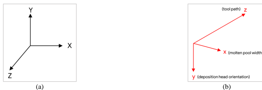
Figure 6-5. (a) Global coordinate system and (b) local coordinate system for the moving heat source by transformation of the global coordinate system [403].
