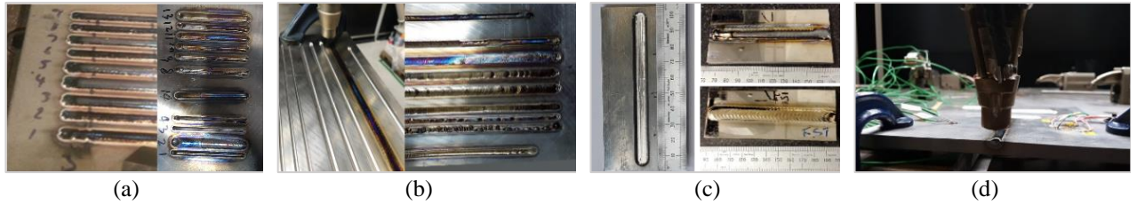
Figure 5-4: Reprocessing strategy involving (a) characterisation of single beads (b) evaluation of different types of features (c) specification of SMRM task inputs and (d) development of in-process monitoring technique.
