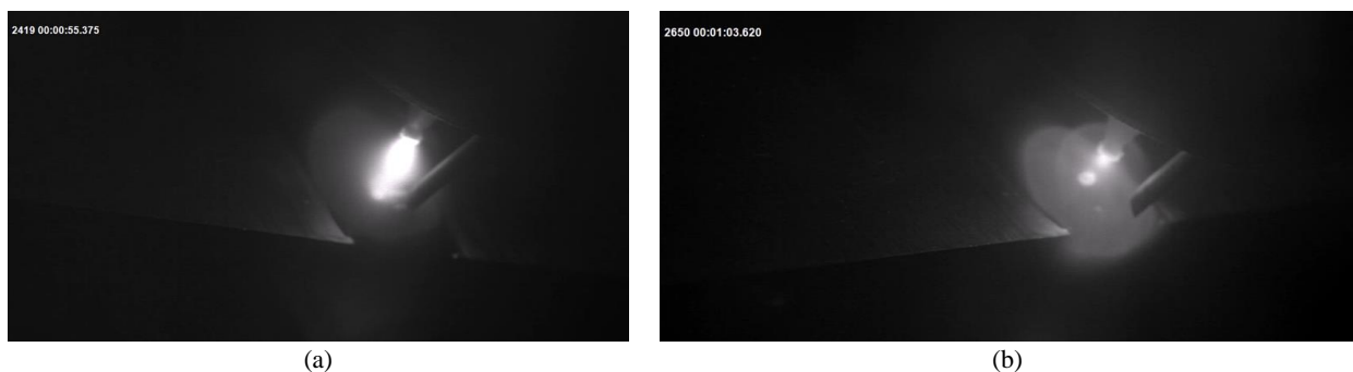
Figure 6-9. Time coded images used for the estimation of molten pool dimensions: (a) arc extinguishing point and (b) estimated molten pool dimensions as the arc is extinguished. Arc properties 130A, 13V, 3 mm arc gap
