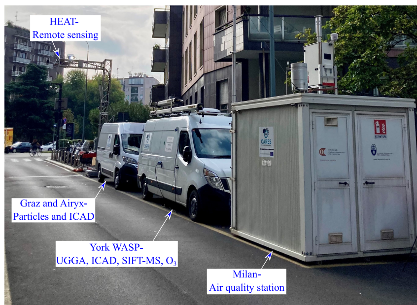
Figure 2.11: Set-up of the vehicle point sampling measurements in Milan.
