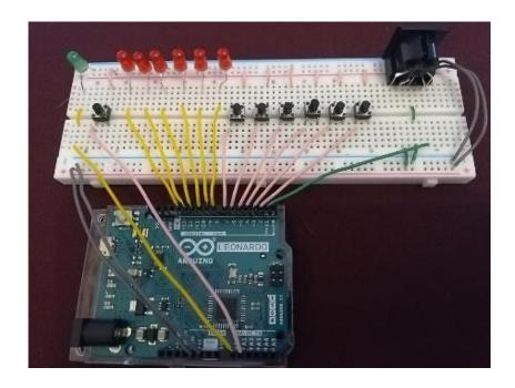
Figure 7.9. The Prototype: a simplified, colour-coded breadboard circuit.
