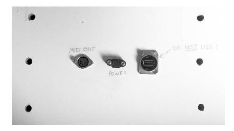
Figure 7.11. The MIDI and USB power sockets fixed to the chassis at the back of the interface, providing better modularity between the interface and the cabinet.
