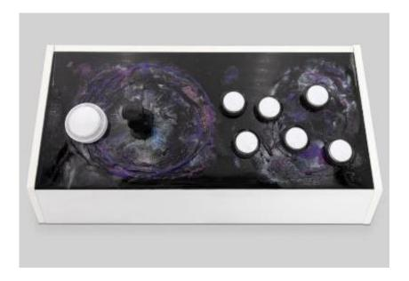
Figure 7.10. The final interface. The black 'space' background was created using a resin pour process.
