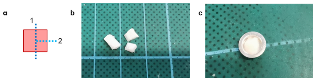
Figure 2.6: Sample preparation for differential scanning calorimetry.
