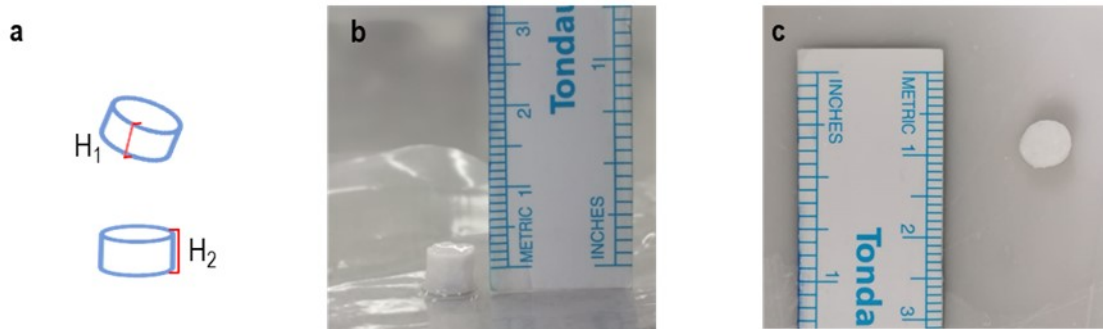
Figure 4.2: Cylindrical 6 mm diameter pSFT plugs for compression characterisation
