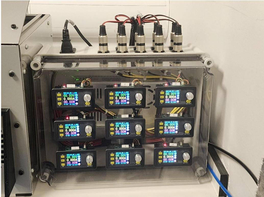
**Figure 3.15: The laser power supply used to control each laser module individually.**
