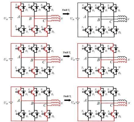
Fig. 3-1. Current loop in healthy and fault conditions.
