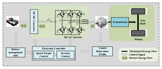
Fig. 2-1. The basic structure of the motor drive system.
