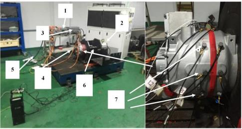
1. Inverter of prototype2. Dyno3. Controller of Dyno4. Prototype5. Water cooling system6. Speed and torque sensor7. B&K 4520 type 3D acceleration sensor
