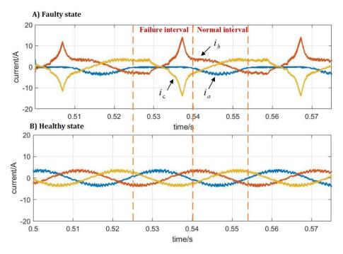
Fig. 3-2. Responses in the faulty half of a fundamental period.
