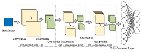
Fig. 2-9. The basic structure diagram of CNN.
