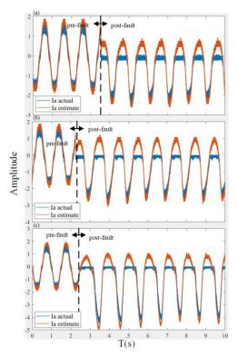
Fig. 3-8. Phase A estimate and actual current under different fault states (a) fault T1 state. (b) fault T1&T4 state. (c) fault T1&T3 state.
