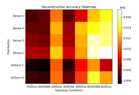
Fig. 5-13. Heatmap for different sensor distribution and operating conditions.
