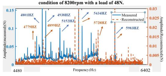
Fig. 4-12. Measured and reconstructed value of OCF under the condition of 8200rpm with a load of 48N.
