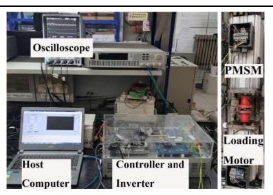
Fig. 3-5. The experimental platform.
