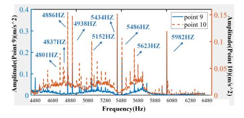
Fig. 5-11. Spectrum of acceleration response under the condition of 8200rpm without load for sensor point 9 and point 10.
