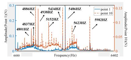
Fig. 4-14. Spectrum of OCF under the condition of 8200rpm without load for sensor point 9 and point 10.
