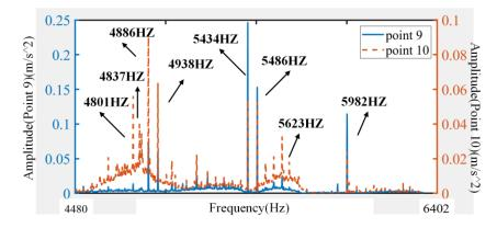
Fig. 4-13. Spectrum of OCF under the condition of 6000rpm without load for sensor point 1 and point 10.
