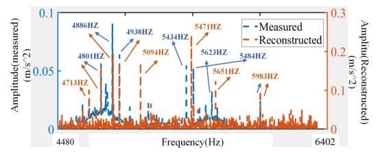
Fig. 4-10. Measured and reconstructed value of acceleration response under the condition of 6000rpm without load.
