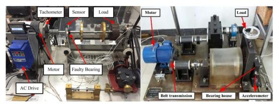
Fig. 2-2. The example of experimental rigs [42][106].
