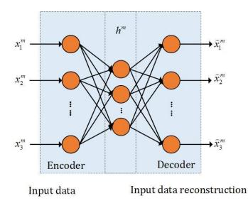
Fig. 2-3. The basic structure diagram of AE.
