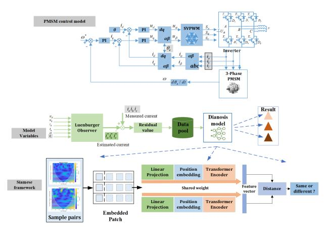
Fig. 3-4. Flowchart of model-data-hybrid-driven diagnosis method.
