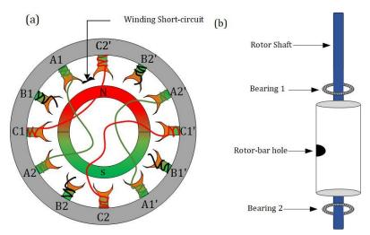
Fig. 2-4. Typical faults: (a) Stator winding short-circuit (WSC). (b) Rotor crack fault (CRF) [226].
