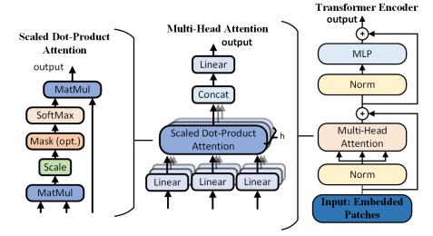
Fig. 3-3. Structure of transformer encoder.
