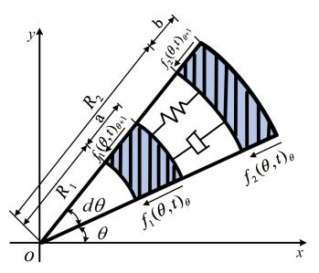
Fig. 4-2. Shell micro-element segment.
