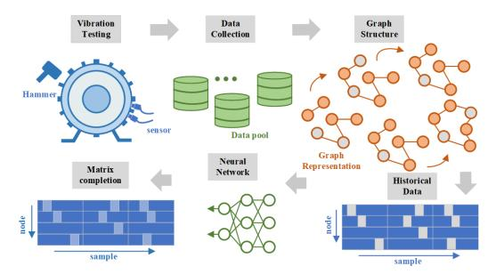
Fig. 5-4. Diagram of data-driven for signal reconstruction in vibration testing.
