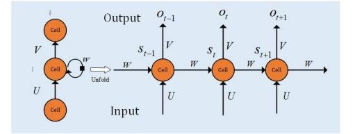
Fig. 2-10. The basic structure diagram of RNN.
