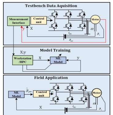
Fig. 2-14. The entire process test bench.
