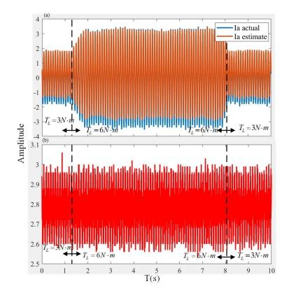
Fig. 3-6. Dynamic responses under load change between 3 N.m and 6 N.m (a) phase A estimate and actual current. (b) phase A residuals.
