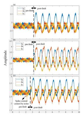
Fig. 3-7. Three phase residuals under different fault states (a) fault T1 state. (b) fault T1&T4 state. (c) fault T1&T3 state.
