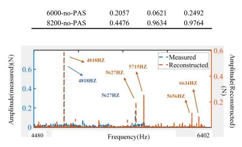
Fig. 4-9. Measured and reconstructed value of OCF under the condition of 6000rpm without load.
