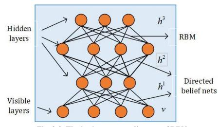
Fig. 2-2. The basic structure diagram of DBN.
