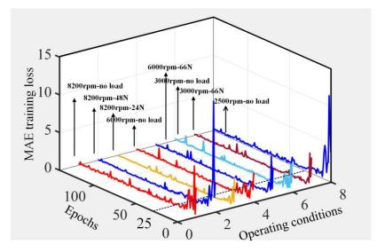
Fig. 4-15. Curve of MAE training loss with different epochs.
