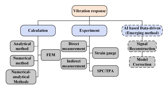
Fig. 4-1. Classification of vibration analysis methods [22].
