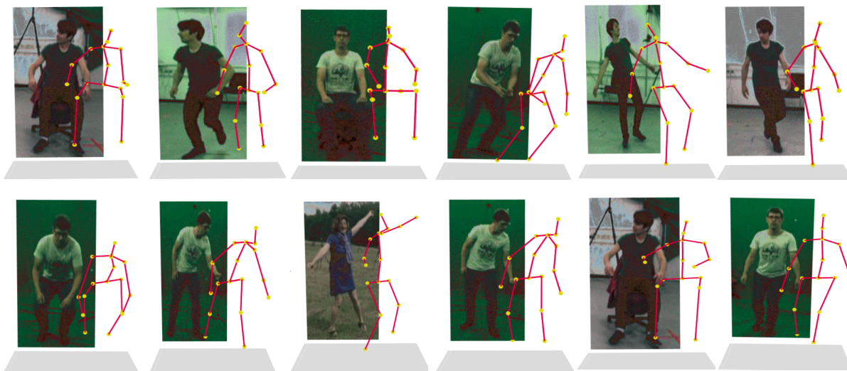
Figure 4.15: Qualitative results on images from MPI-INF-3DHP dataset. Each figure contains the input image and its corresponding estimated 3D pose by our model. An extended version of qualitative results for this dataset is included in Appendix B .
