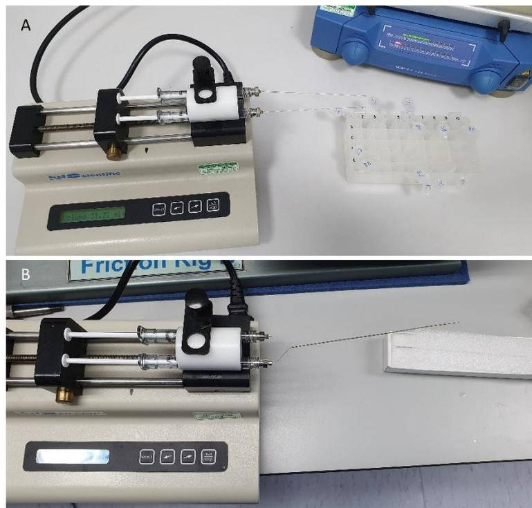
**Figure 4-1 – Syringes placed in the syringe driver with A) two straight needles attached and B) one bespoke needle attached.**
