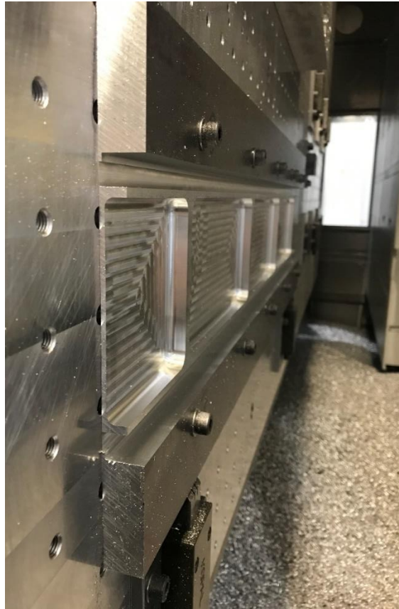
Figure 5-35: End of TPC2 stage 2 machining
