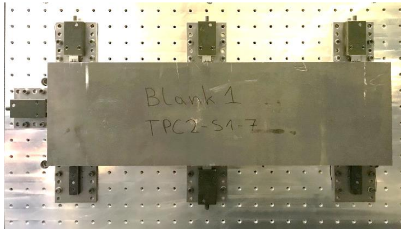
Figure 5-32: TPC2 stage 1 work holding on machine
