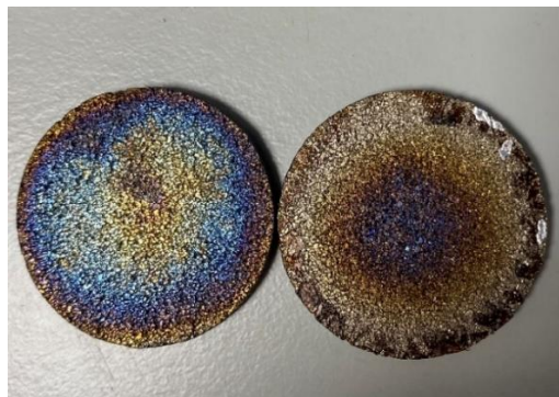
Figure 3.5 Deformed sintered plate after a period of use.
