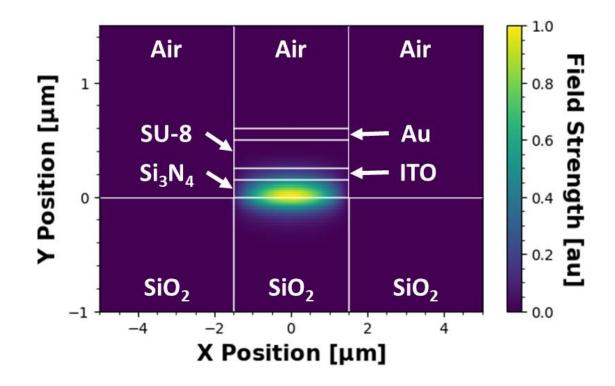
Figure 3.3: Cross-section of slab waveguide with metal-oxide-semiconductor structure surrounded by air.
