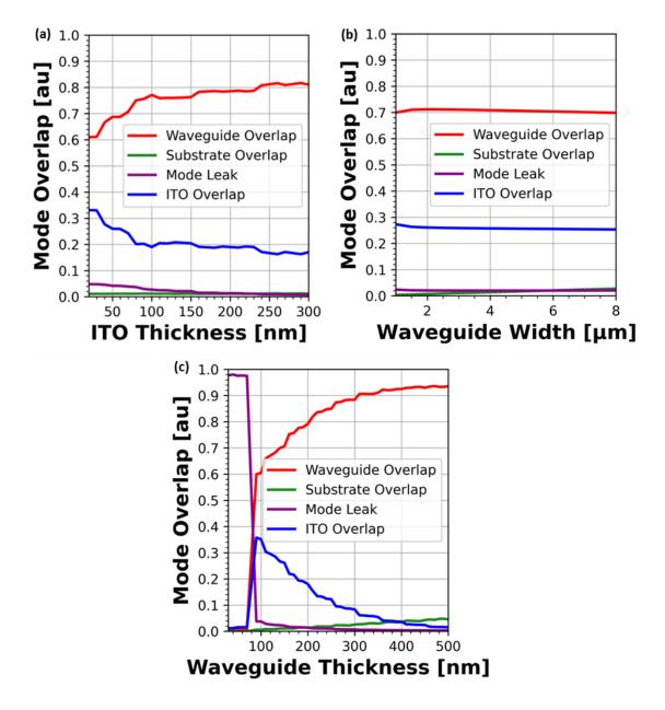
Figure 9.4: Mode overlap as a function of (a) indium tin oxide layer thickness, (b) waveguide width, and (c) waveguide layer thickness for a fully surrounded waveguide structure.
