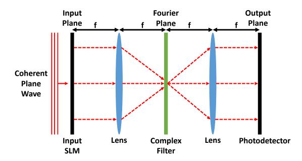
Figure 1.5: 4f coherent optical processor.
