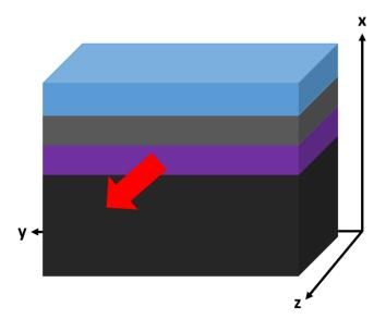
Figure 2.8: Illustration of slab waveguide, layer materials, permittivities, and dimensions are not important, note that the y scale is significantly larger than the wavelength of propagating light to ensure invariance in y. Propagation is in the z-direction, indicated by the red arrow.
