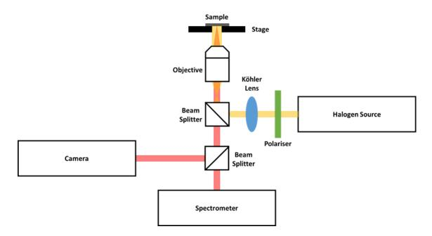
*Figure 4.16: Optical setup for measuring the reflectance of guided mode resonance spectra for 1D periodic structures in ITO.*
