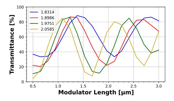
Figure 7.13: Intensity transmitted into the waveguide after passing through the MOS capacitor modulator stack as a function of effective waveguide mode index.
