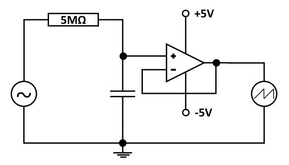
Figure 6.5: Illustration of an RC charging circuit with (from left to right) an input alternating current supply, a 5M $\Omega$  resistor, a capacitor, an operational amplifier, and an oscilloscope.
