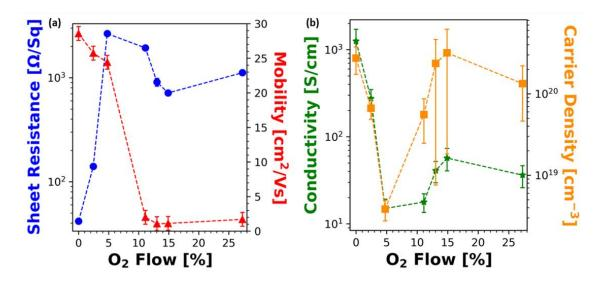
Figure 4.10: (a) Measured sheet resistance and carrier mobility for sputter deposited ITO film and the (b) calculated conductivity and carrier density as a function of oxygen concentration.
