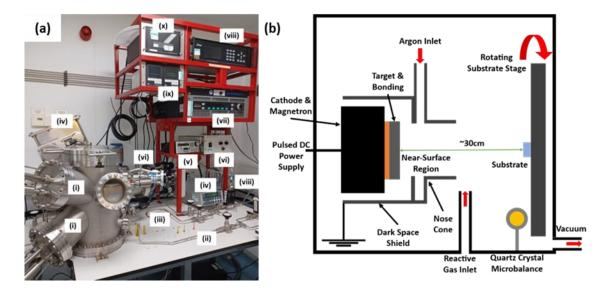
Figure 5.5: (a) Photograph and (b) schematic of the bespoke pulsed DC reactive magnetron sputterer at York, schematic not to scale.
