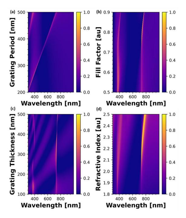
Figure 3.2: Reflectance surface plots with incident wavelength on the x-axis and (a) grating period, (b) fill factor, (c) grating thickness, and (d) grating refractive index on the y-axis. Reflectance is given by the colour bar. Simulations conducted using RCWA ( $S^4$ ) software. The base parameters were a period of 500 nm, grating thickness of 150 nm, fill factor of 0.7, and a refractive index of 2.0 for the grating layer.
