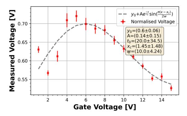
Figure 7.15: Oscilloscope measured voltage as a function of capacitor gate voltage for a 600  $\mu$ m single capacitor, single waveguide, modulator for a 520 nm input.
