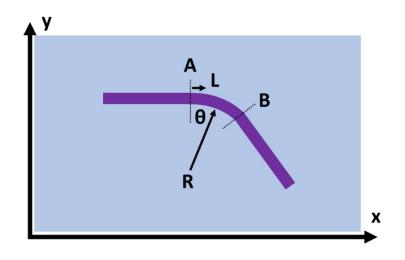
Figure 3.11: Straight waveguide – bend – straight waveguide geometry.
