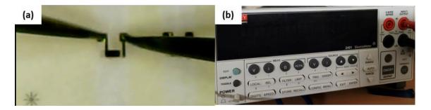
Figure 7.4: (a) Electrical contact made to the metal-oxide-semiconductor capacitor arms with 4-axis probes. (b) Keithley 2440 Bench Top DC Power Supply
