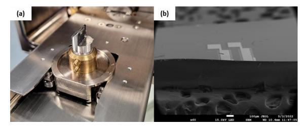
Figure 6.7: (a) Vertical sample mounting in the scanning electron microscope loading stage, (b) cleaved cross-section of the metal-oxide-semiconductor capacitor viewed under the scanning electron microscope at a 20° angle.
