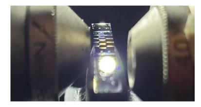
*Figure 7.3: Facet coupled input (left) and output (right) objectives, with magnification and focal lengths 60x and 40x, 2.8mm and 4.5mm, respectively.*
