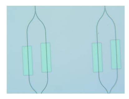
Figure 5.22: Micrograph of phase modulators with double capacitors, showing only the waveguide layer and ITO layer.
