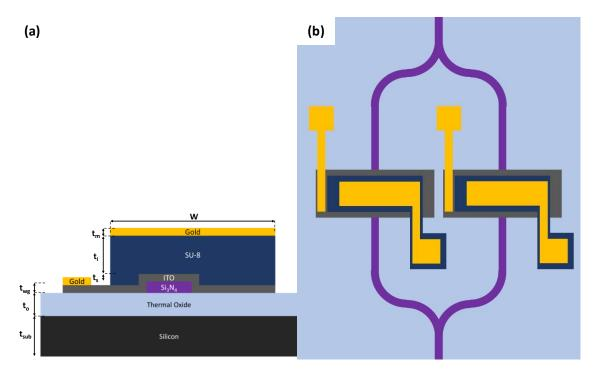
Figure 5.1: (a) Layer structure of the MOS EO modulator with dimensions:  $W \sim 3\mu m$ ,  $t_{sub} \sim 525\mu m$ ,  $t_{wg} \sim 100$ nm,  $t_i \sim 200$ nm, and  $t_m \sim 100$ nm. (b) Device structure of the phase modulator.
