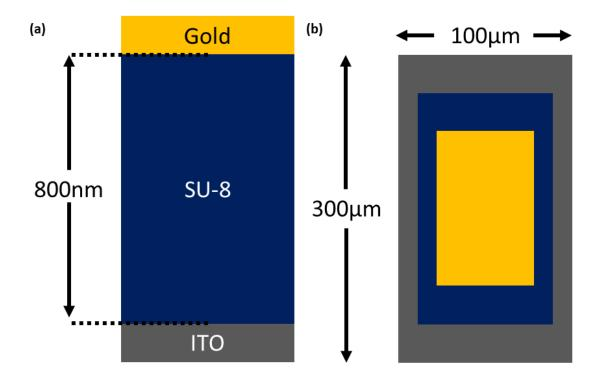
Figure 6.1: Schematic of the (a) cross-section and (b) top-down view of the capacitor with approximate layer thickness and dimensions.
