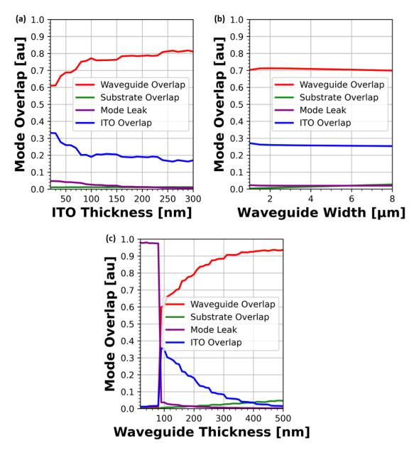
Figure 9.5: Mode overlap as a function of (a) indium tin oxide layer thickness, (b) waveguide width, and (c) waveguide layer thickness for a partially surrounded waveguide structure.
