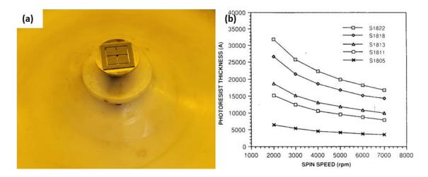
Figure 5.2: (a) Spin coater available at York and (b) photoresist thickness as a function of spin speed for S1800 photoresist series [233].
