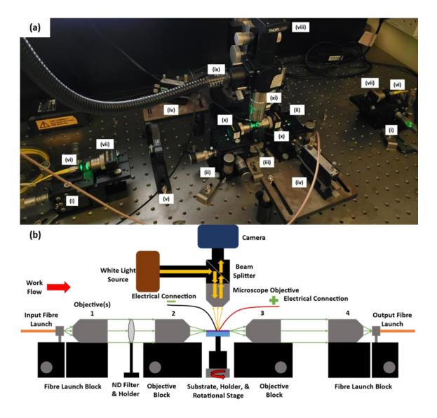
Figure 7.1: (a) Photograph and (b) illustrated schematic of the optical setup used to obtain amplitude and phase modulation results in this research. The individual components are discussed throughout this chapter.
