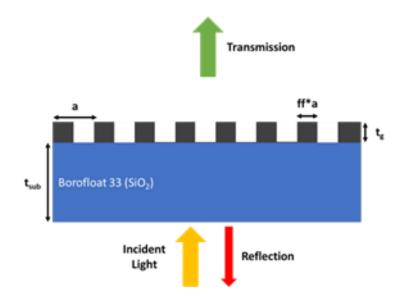
Figure 2.7: Schematic of sub- $\lambda$  operating mode for a resonant structure.
