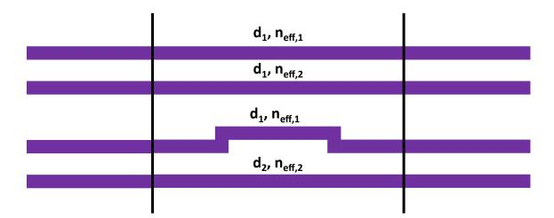
Figure 2.12: Illustration of phase shift methods in Mach-Zehnder modulator.
