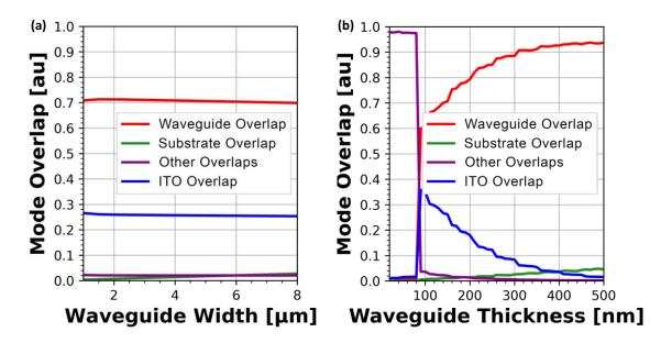
Figure 3.4: (a) Mode overlap as a function of slab waveguide width and (b) mode overlap as a function of waveguide layer thickness.
