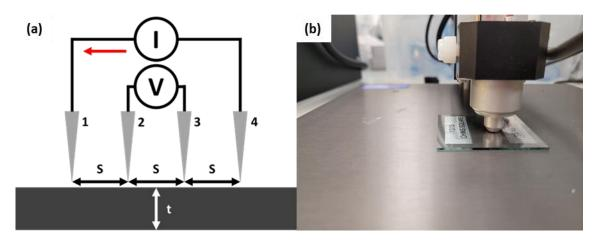
*Figure 4.8: (a) Schematic diagram and (b) picture of the four-point probe system at York. Here the probe is pictured measuring a calibration sample.*
