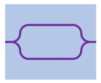
Figure 2.11: Mach-Zehnder interferometer waveguide platform.
