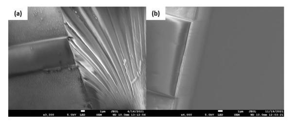
*Figure 5.30: Scanning electron microscope images of cleaved facet from (a) silicon nitride on borofloat 33 substrate and (b) silicon nitride on thermal oxide on silicon substrate.*
