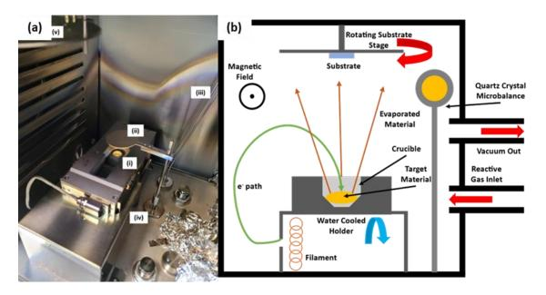
*Figure 5.7: (a) Photograph of material crucible, electron beam filament, and water-cooling stage at York, (b) schematic of electron beam evaporator at York.*
