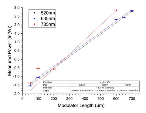
Figure 9.20: Measured incident power on the oscilloscope as a function of modulator length for incident wavelengths of 520nm (black), 635nm (blue), and 785nm (red).
