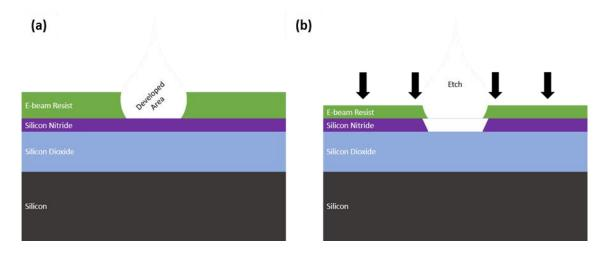
Figure 5.10: (a) Post exposure development and (b) dry etch patterning.
