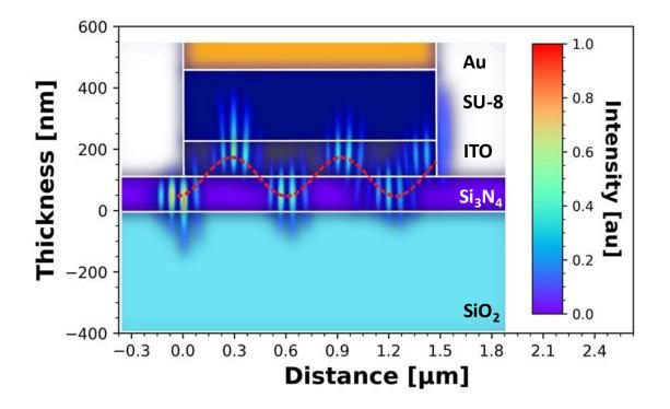
Figure 7.12: Fundamental waveguide mode in a  $1.5\mu$ m gold, SU-8, ITO, silicon nitride on glass modulator side-profile. The waveguide mode profile is imposed onto an illustration of the modulator with thicknesses and lengths shown. Intensity is shown by the colour scale on the right of the figure. The ITO has a refractive index of 2.2.
