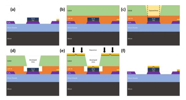
Figure 5.25: UVL and bilayer lift-off for electrical contact patterning.
