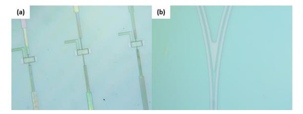
*Figure 5.20: Micrographs of (a) tapered silicon nitride waveguide with SU-8 waveguides and (b) Y-junction splitter fabricated in silicon nitride.*
