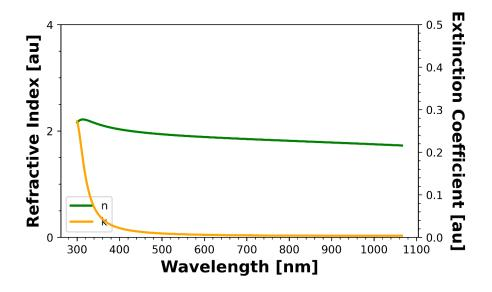
Figure 9.11: Real (green) and imaginary (orange) components of the complex refractive index of a sputter deposited ITO thin film with 1% oxygen flow concentration.
