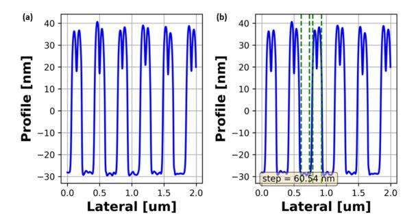
Figure 4.13: Atomic force micrographs of a 1D periodic structure in ITO showing the (a) raw and (b) step height calculated data of 60.54 nm.
