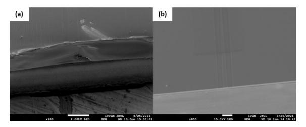
Figure 5.31: Scanning electron microscope images of cleaved facet from (a) silicon nitride on borofloat 33 substrate and (b) silicon nitride on thermal oxide on silicon substrate, captured with a low magnification.
