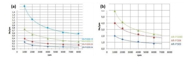
Figure 9.15: Film thickness as a function of spin speed for (a) AR-P 6200 and (b) AR-PC 5000 series [193], [295].
