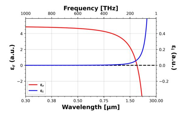
Figure 5.32: Real (red) and imaginary (blue) components of the Drude permittivity for sputter deposited ITO with a 27% oxygen flow concentration during deposition.
