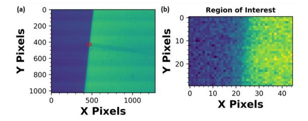
Figure 7.5: (a) Raw image from the camera showing the output waveguide facet from the top-down, the desired region of interest is marked with a red box and shown in (b).
