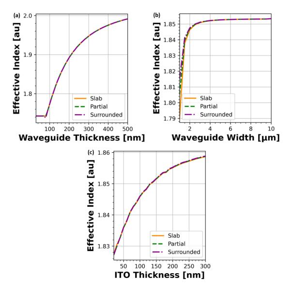
Figure 3.7: Waveguide mode effective index for the slab (orange), partial (green), and surrounded (purple) waveguide designs as a function of (a) waveguide thickness, (b) waveguide width, and (c) indium tin oxide layer thickness measured using the effective index method in finite-difference time-domain simulation in Lumerical.
