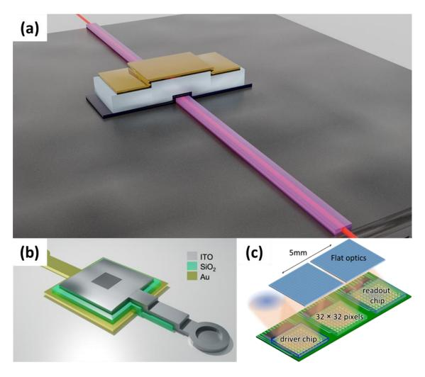
Figure 8.1: Blender designed renders of (a) a planar (waveguide) modulator and (b) an out-of-plane (resonant) modulator. (c) A concept of an out-of-plane 4f coherent optical processor. Credit: (b) & (c) S. Blair 2023.
