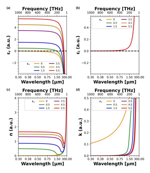
Figure 4.3: (a) Real and (b) imaginary components of the complex Drude permittivity and the corresponding (c) refractive index and (d) extinction coefficient of the complex refractive index as a function of the high frequency permittivity.
