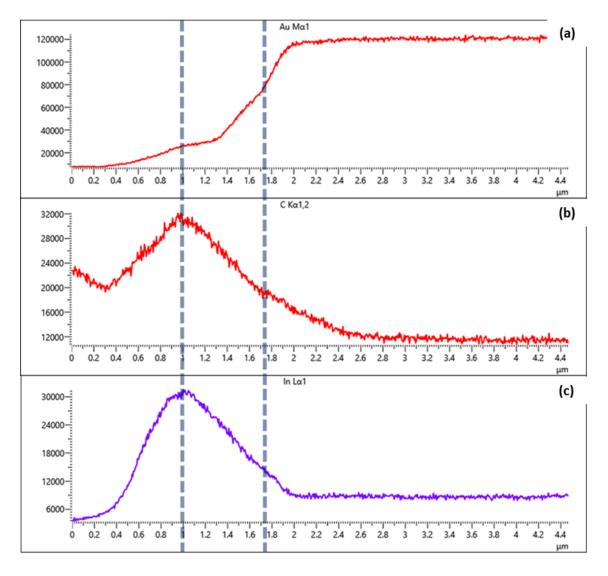
Figure 6.10: Elemental counts per second as a function of the distance across the cross-section of the rgion of interest for (a) gold, (b) carbon, and (c) indium, with the approximate insulator layer thickness marked with blue dotted lines.
