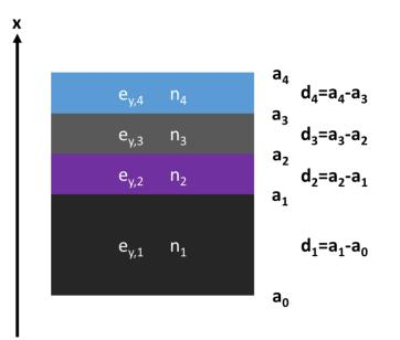
*Figure 2.9: Multilayer slab waveguide with piecewise refractive index (n), electric field (e), and thickness (d).*
