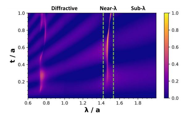
Figure 2.4: Reflectance as a function of wavelength ( $\lambda$ ) and grating thickness (t), both normalised to grating period (a), showing the diffractive, near- $\lambda$ , and sub- $\lambda$  operation modes.
