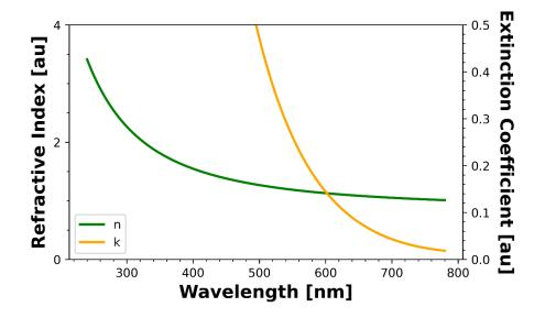
Figure 9.8: Real (green) and imaginary (orange) components of the complex refractive index of a sputter deposited ITO thin film with 1% oxygen flow concentration.
