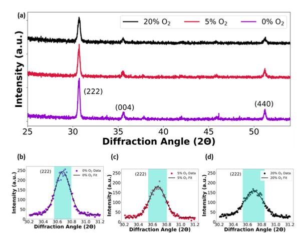
Figure 4.11: (a) XRD data for annealed ITO films of 0%, 5%, and 20% oxygen flow during deposition. (b), (c), and (d) show exemplar FWHM extractions for the respective (222) orientation for 0%, 5%, and 20% oxygen flow. The FWHM increases from 0.246° for 0% oxygen to 0.361° for 20% oxygen concentration.
