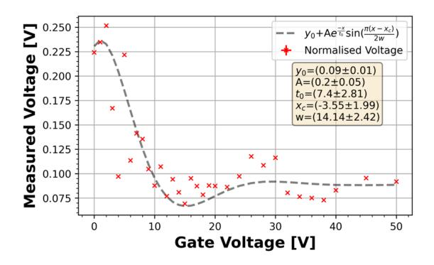
Figure 7.9: Oscilloscope measured voltage as a function of capacitor gate voltage for a 70  $\mu$ m single capacitor modulator.
