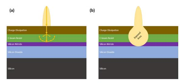
Figure 5.3: (a) Interaction of electrons with resist illustrating proximity effect and (b) the exposed area remaining.
