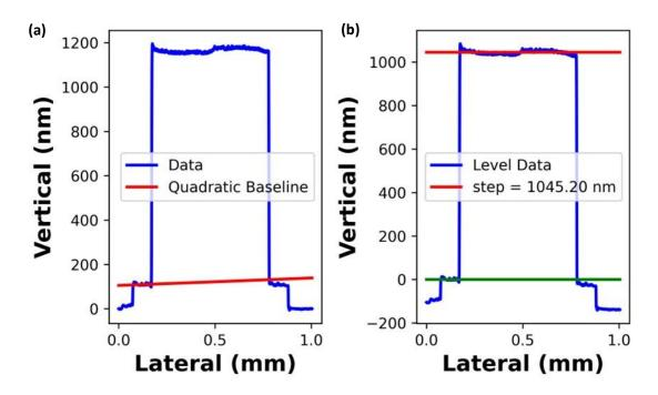
Figure 6.3: Surface profile analysis of SU-8 capacitor layer showing (a) distorted and (b) levelled surface profile.
