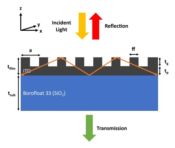
Figure 4.18: Guided mode resonance exhibited in an ITO grating, required simulation parameters labelled.
