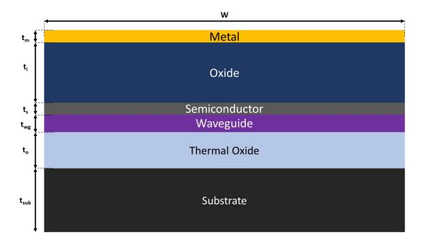
Figure 3.1: Schematic of proposed MOS EO Modulator where width (W) and thicknesses (t) are discussed in this chapter.
