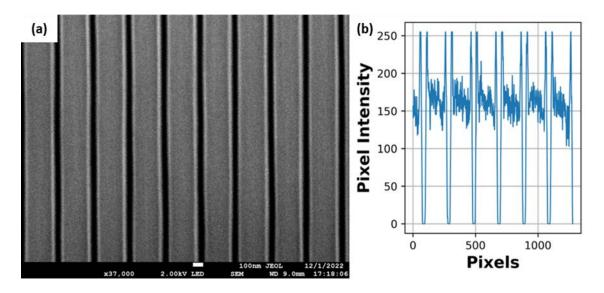
Figure 4.14: (a) Scanning electron micrograph of a 1D periodic structure in ITO, taken at 37,000x magnification, 9mm working distance, and 2kV beam power. (b) Raw pixel intensity across 1 row of an SEM image of a 1D periodic structure in ITO.
