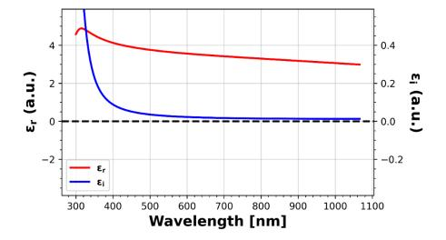
*Figure 9.10: Real (red) and imaginary (blue) components of the complex permittivity of a sputter deposited ITO thin film with 17% oxygen flow concentration.*
