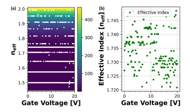
Figure 9.22: Effective index as a function of gate voltage for an ITO based modulator plotted as (a) a surface plot with the propagation constant and (b) the gate voltage.
