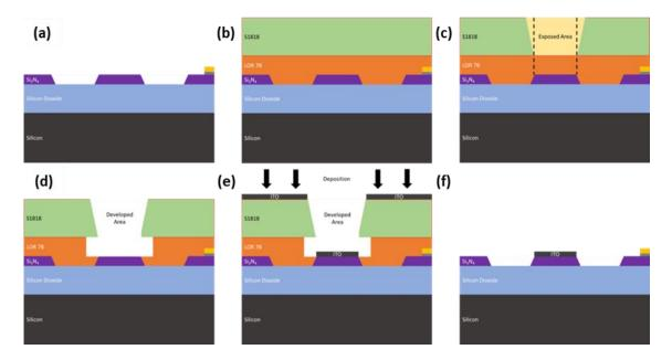
Figure 5.21: UVL and bilayer lift-off for ITO patterning.
