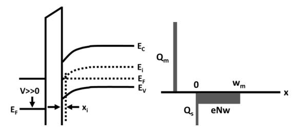
Figure 2.17: Energy band diagram and charge distribution of an ideal MOS capacitor in inversion.
