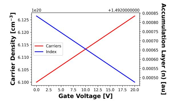
Figure 9.21: Predicted local carrier density (red) and refractive index (blue) within a 5nm accumulation layer of ITO. The letter has a linear relationship.
