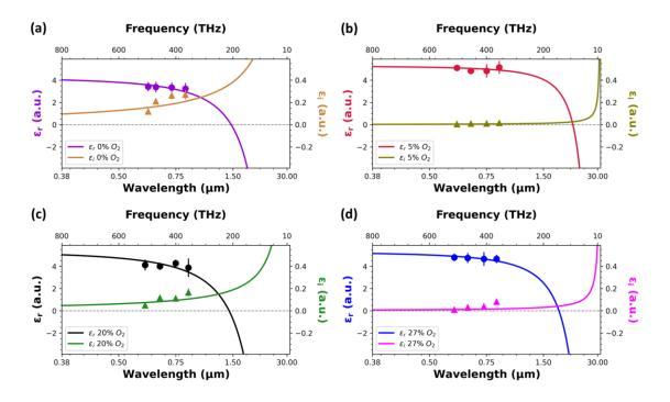
*Figure 4.21: Real and imaginary dielectric permittivity as a function of wavelength (frequency) for ITO films deposited with (a) 0%, (b) 5%, (c) 20%, and (d) 27% oxygen flow.*
