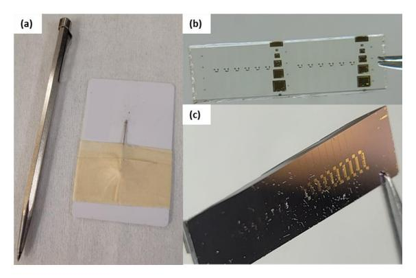
*Figure 5.26: (a) Cleaving tool and scribe, (b) cleaved silicon nitride on borofloat 33 sample, and (c) cleaved silicon nitride on thermal oxide on silicon sample.*
