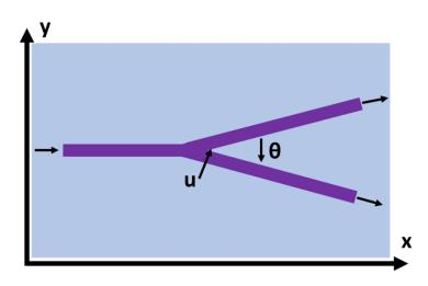
Figure 3.10: Optical power splitter with Y-junction waveguides.
