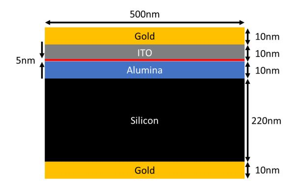
Figure 2.18: 2D schematic of the structure presented by Sorger et al.
