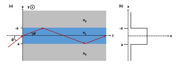
Figure 2.1: (a) Basic structure of the optical waveguide with indicated refractive indices and (b) refractive index profile of the optical waveguide. Light ray is indicated by the red arrow in (a), guided in the blue waveguide layer.
