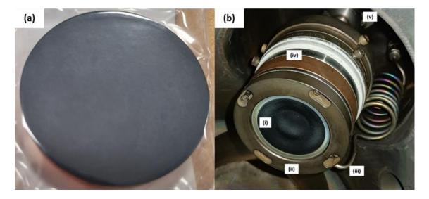
Figure 5.6: Indium tin oxide sputter target (a) new and (b) placed in the sputter gun, clamped into place, with dark space shield removed.
