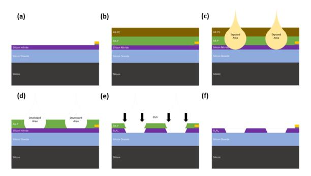
Figure 5.18: EBL and dry etching for waveguide patterning.
