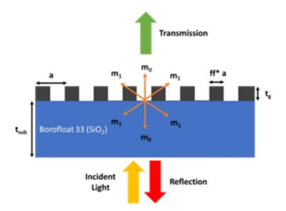
*Figure 2.5: Schematic of diffractive operating mode for a resonant structure.*
