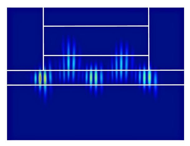
Figure 9.17: Fundamental waveguide mode in a 1.5  $\mu$ m gold, SU-8, ITO, silicon nitride on glass modulator side-profile. The waveguide mode profile is shown imposed on top of each other from 5 images. The ITO has a refractive index of 1.9.
