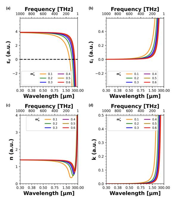
Figure 4.5: (a) Real and (b) imaginary components of the complex Drude permittivity and the corresponding (c) refractive index and (d) extinction coefficient of the complex refractive index as a function of the effective electron mass.
