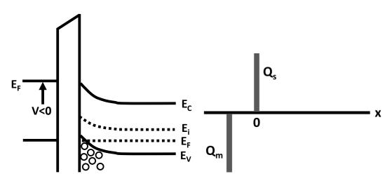
Figure 2.15: Energy band diagram and charge distribution of an ideal MOS capacitor in accumulation.
