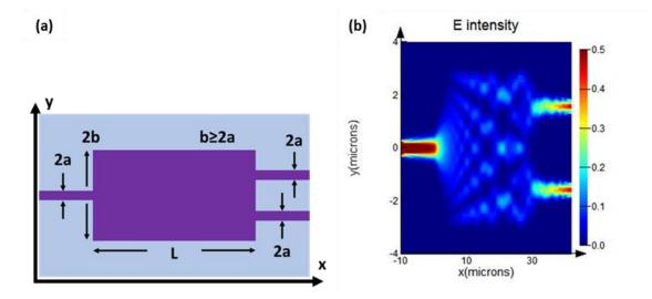
*Figure 3.9: (a) Schematic of a one-to-two multimode propagation splitter in solid-core waveguide technology. (b) Electric field profile of a one-to-two multimode propagation splitter [161].*
