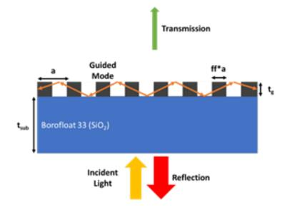
Figure 2.6: Schematic of near- $\lambda$  operating mode for a resonant structure.
