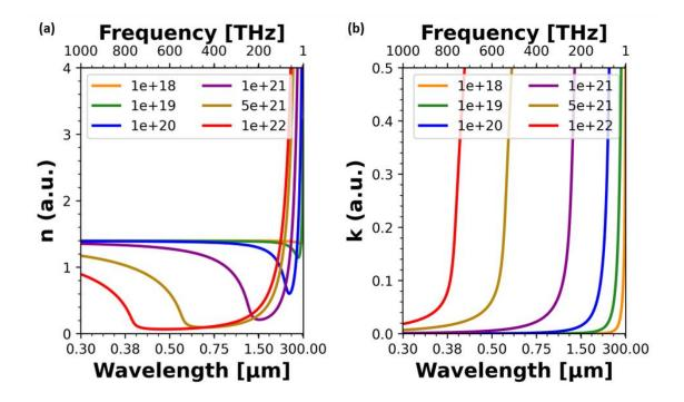
Figure 4.2: (a) Refractive index and (b) extinction coefficient components of the complex refractive index calculated from the Drude permittivity for literature values of free carrier density. Data taken from Sorger et al. [187] and replotted. Carrier densities are expressed in cm<sup>-3</sup> as is customary in the field.
