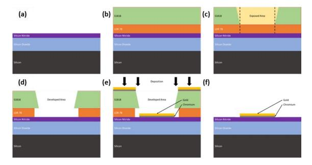
Figure 5.16: Bilayer lift-off for alignment mark patterning.
