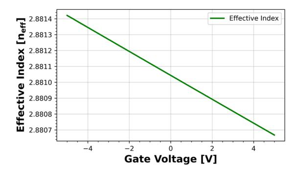
*Figure 2.20: Effective index as a function of gate voltage for ITO-based modulation in [77] plotted as a function of the gate voltage.*
