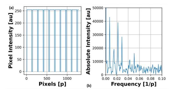
Figure 4.15: (a) Threshold treated data of 1 row of an SEM image of a 1D periodic structure in ITO and (b) the corresponding Fourier space frequencies.
