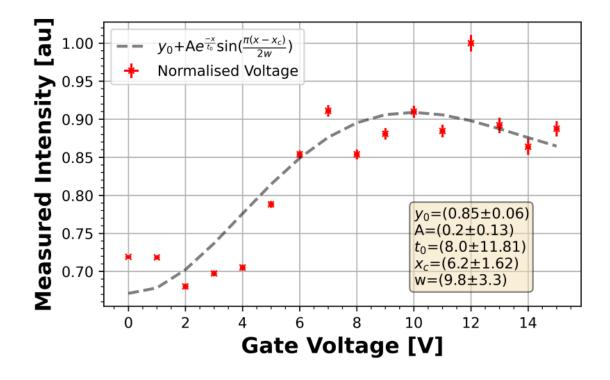
Figure 7.16: Normalised camera intensity at capacitor exit as a function of capacitor gate voltage for a 600  $\mu$ m single capacitor, single waveguide, modulator for a 520 nm input.
