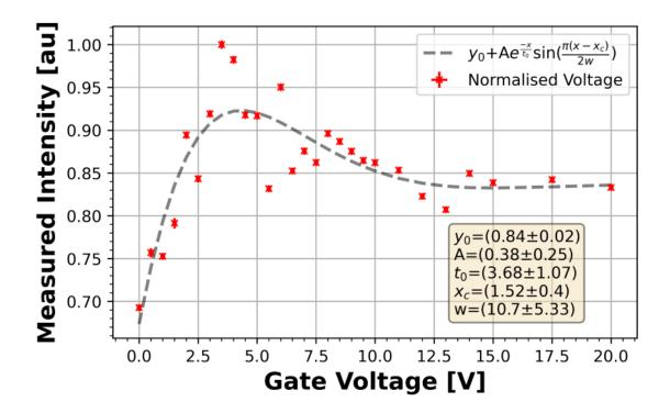
Figure 7.18: Normalised camera intensity at capacitor exit as a function of capacitor gate voltage for a 50  $\mu$ m single capacitor, single waveguide, modulator for a 635 nm input.
