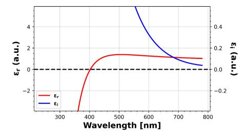
Figure 9.7: Real (red) and imaginary (blue) components of the complex permittivity of a sputter deposited ITO thin film with 1% oxygen flow concentration.
