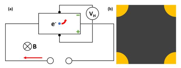
Figure 4.9: Schematic of (a) a Hall effect measurement setup and (b) Van de Pauw electrical contact configuration.
