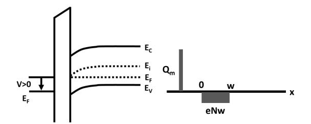
*Figure 2.16: Energy band diagram and charge distribution of an ideal MOS capacitor in depletion.*
