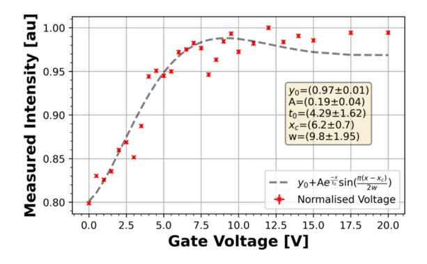
Figure 7.20: Normalised camera intensity at capacitor exit as a function of capacitor gate voltage for a 100  $\mu$ m single capacitor, single waveguide, modulator for a 785 nm input.
