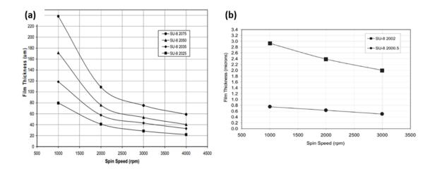
*Figure 9.13: Thickness as a function of spin speed for SU-8 2000 series [294] showing the (a) thicker and (b) thinner films in the range.*
