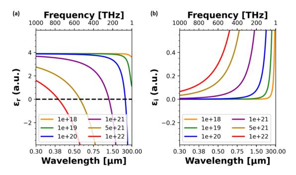
Figure 4.1: (a) Real and (b) imaginary components of the complex Drude permittivity for literature values of free carrier density. Data taken from Sorger et al. [187] and replotted. Note that carrier density is expressed in cm<sup>-3</sup> as is customary in the field.
