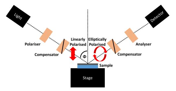
Figure 9.6: Optical elements required to determine the change in polarisation of the light upon reflection at the sample, (Spectroscopic Ellipsometer setup) [314].
