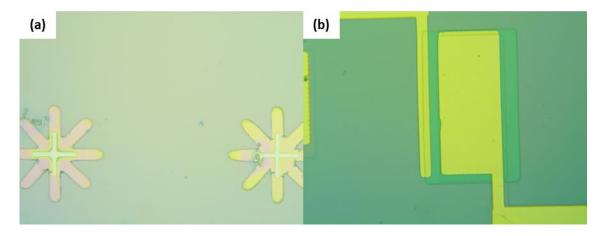
*Figure 5.14: Micrographs of (a) UV and electron beam lithography alignment marks, and (b) misaligned MOS capacitor components.*
