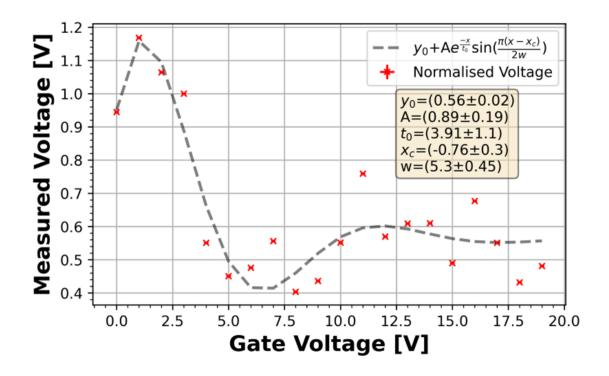
Figure 7.8: Oscilloscope measured voltage as a function of capacitor gate voltage for a 60  $\mu$ m single capacitor modulator.
