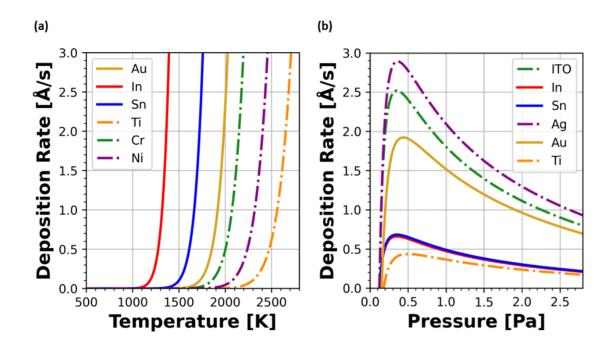
Figure 5.8: Approximation of deposition rate as a function of (a) evaporation temperature for electron beam evaporation of common materials, and (b) plasma pressure for pulsed DC reactive magnetron sputtering of common materials.
