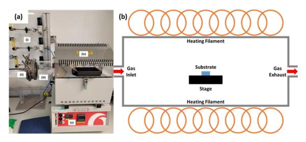
Figure 5.12: (a) Photograph and (b) schematic of the tube furnace available at York.
