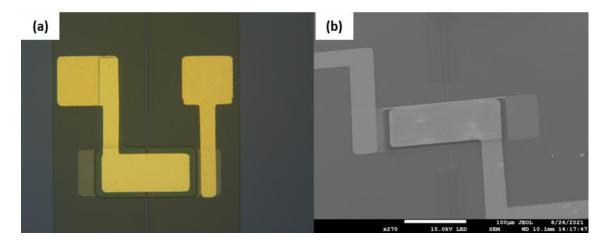
Figure 5.27: (a) Optical and (b) electron microscope image of fabricated MOS EO modulator showing waveguide, ITO, SU-8, and electrical contact layers.
