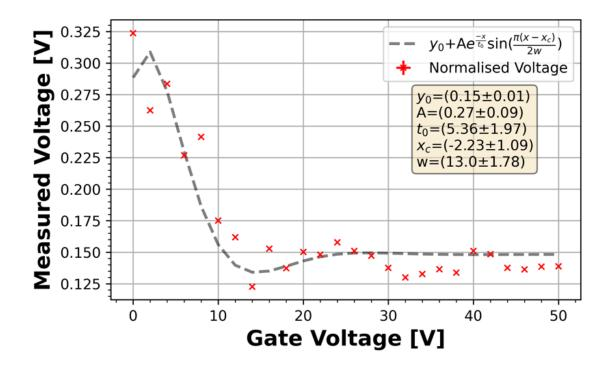
Figure 7.10: Oscilloscope measured voltage as a function of capacitor gate voltage for a 100 μm double capacitor modulator.
