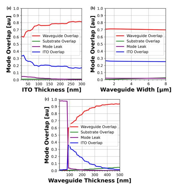
Figure 9.3: Mode overlap as a function of (a) indium tin oxide layer thickness, (b) waveguide width, and (c) waveguide layer thickness for a slab structure.
