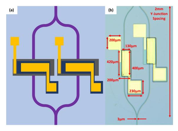
Figure 3.12: (a) Illustrate diagram and (b) micrograph of the phase modulator with a capacitor on each arm of the Mach-Zehnder architecture.
