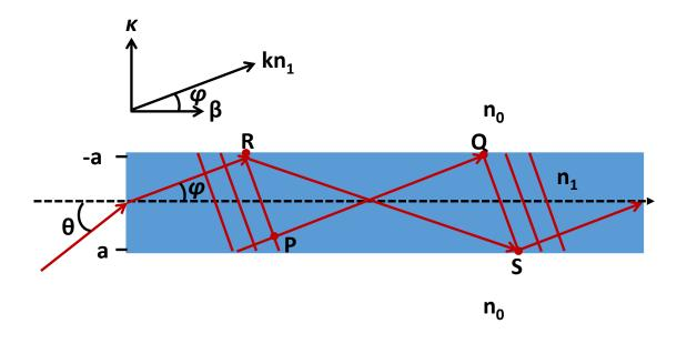
Figure 2.2: Light rays and their phase fronts in an optical waveguide.
