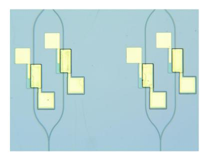
*Figure 5.28: Micrograph of phase modulators with double capacitors, showing only the waveguide, ITO, SU-8, and gold layers.*
