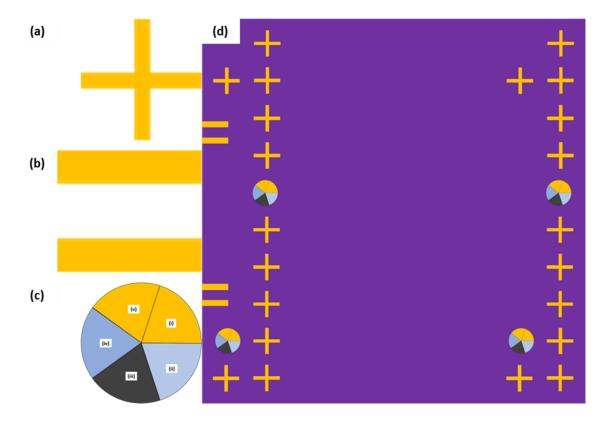
Figure 5.15: Alignment mark designs, showing (a) individual cross marker, (b) cleave marker, (c) layer alignment marker, and (d) sample layout (not to scale).
