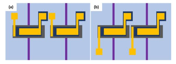
Figure 3.8: Top-down illustration of the (a) same level and (b) staggered top and bottom electrical contacts with arrayed modulators.
