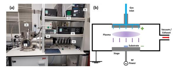
Figure 5.9: (a) Photograph and (b) schematic of the bespoke reactive ion etcher at York.
