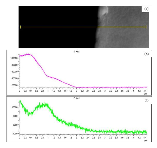
Figure 6.9: (a) Scanning electron micrograph of the region of interest and the corresponding elemental counts per second as a function of the distance across the cross-section of the region of interest for (b) silicon and (c) oxygen.
