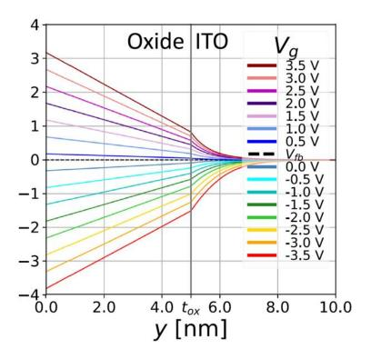
Figure 9.1: The potential profile across the oxide and ITO layers from numerical simulations of [312].
