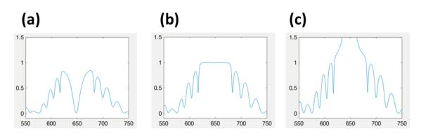
Figure 8.2: Reflectivity spectrum for a distributed Bragg reflector showing a (a) dip in reflection, (b) a flatband response, and (c) a peak in reflection.
