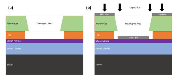
Figure 5.11: (a) Post UV exposure development with bilayer photoresist and (b) targeted thin film deposition.
