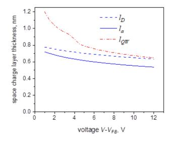
Figure 9.2: Effective space-charge region width, estimated using different analytical methods [311].
