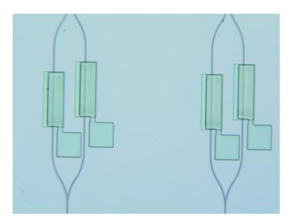
*Figure 5.24: Micrograph of phase modulators with double capacitors, showing only the waveguide, ITO, and SU-8 layers.*
