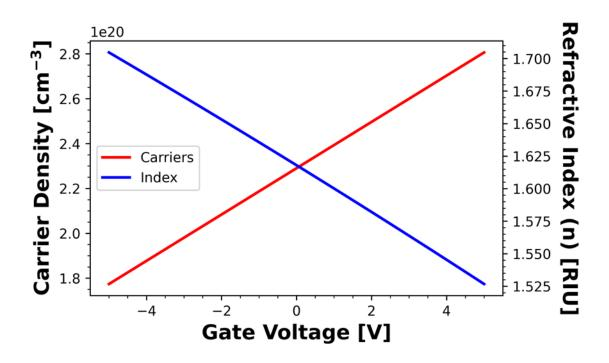
Figure 2.19: Local carrier density and refractive index within 5nm accumulation layer of ITO in [77].
