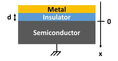
Figure 2.14: Cross-section of a metal-oxide-semiconductor structure.
