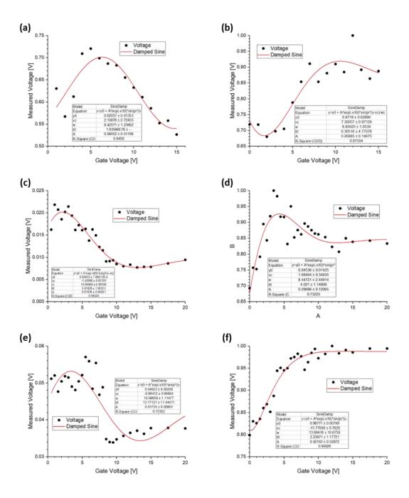
Figure 9.19: Oscilloscope measured voltage as a function of capacitor gate voltage for (a)(b) 600  $\mu$ m, (c)(d) 50  $\mu$ m, and (e)(f) 100  $\mu$ m straight-through modulator at (a)(b) 520 nm, (c)(d) 635 nm, and (e)(f) 785 nm input wavelength.
