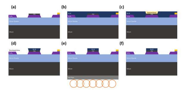
Figure 5.23: UVL and hard baking for SU-8 patterning.
