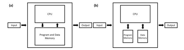
Figure 1.2: (a) Von Neumann and (b) Harvard computing architecture.
