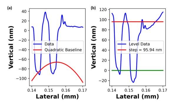
*Figure 5.19: A (a) distorted and (b) levelled surface profile data for the silicon nitride waveguide. Data line marked in blue, quadratic line marked in red, zero marked in green.*
