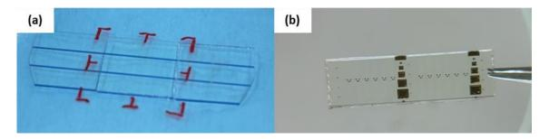
Figure 5.13: (a) Partially diced silicon nitride on borofloat 33 samples, and (b) cleaved chip from partially diced sample.
