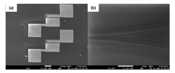
Figure 5.29: Scanning electron micrographs of (a) Y-junction splitter and (b) phase modulator with two capacitors.
