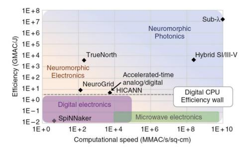
Figure 1.3: Computational efficiency and the digital efficiency wall. Figure taken from neuromorphic photonics [10] under CC-BY. Hybrid Si/III-V is a silicon and group III-V semiconductor simulated neural network PIC, sub- $\lambda$  refers to subwavelength photonics, and the neuromorphic electronics platforms are discussed in later sections.
