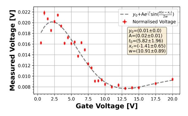
Figure 7.17: Oscilloscope measured voltage as a function of capacitor gate voltage for a 50  $\mu$ m single capacitor, single waveguide, modulator for a 635 nm input.
