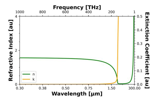
*Figure 5.33: Refractive index (green) and extinction coefficient (orange) components of the complex refractive index of sputter deposited ITO with a 27% oxygen flow concentration during deposition.*
