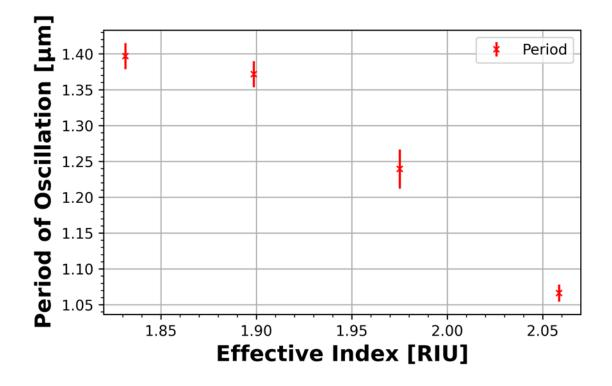
Figure 7.14: Period of transmittance oscillation as a function of waveguide mode effective index.
