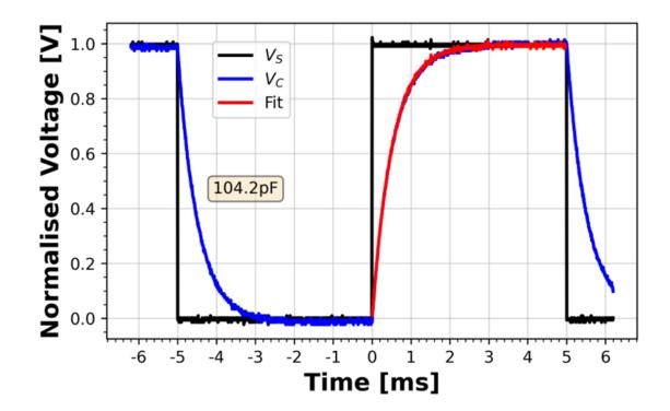
Figure 6.6: Capacitance measurement for 32 parallel capacitors in an RC charging circuit. Input voltage alternates between -0.5 and 0.5 V, normalised to 0-1 V, and is shown in black. The voltage across the capacitor is shown in blue, with the charging region between 0 and 0.005 s. The exponential fit using the calculated capacitance is shown in red.
