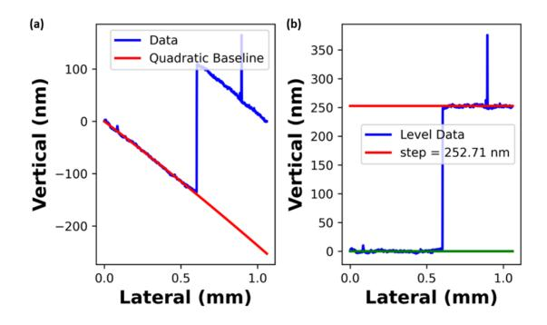
Figure 4.7: A (a) distorted and (b) levelled surface profile data for the same sputter deposited ITO film. Data line marked in blue, quadratic line marked in red, zero marked in green.
