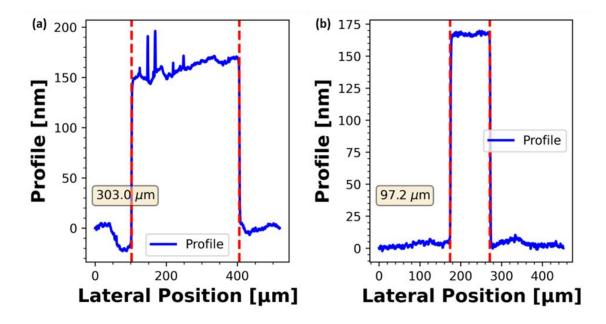
Figure 6.2: Surface profile analysis of indium tin oxide contact measuring (a) length and (b) width of the surface profile.
