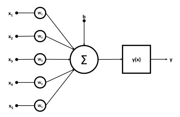
Figure 1.4: Nonlinear model of an artificial neuron.
