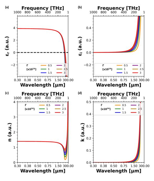
Figure 4.4: (a) Real and (b) imaginary components of the complex Drude permittivity and the corresponding (c) refractive index and (d) extinction coefficient of the complex refractive index as a function of the collision frequency.
