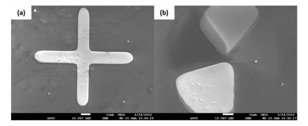
Figure 5.17: (a) individual alignment mark and (b) layer alignment marks.
