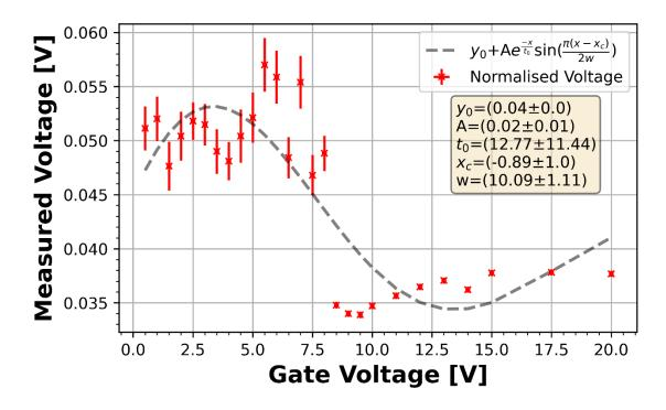
Figure 7.19: Oscilloscope measured voltage as a function of capacitor gate voltage for a 100  $\mu$ m single capacitor, single waveguide, modulator for a 785 nm input.
