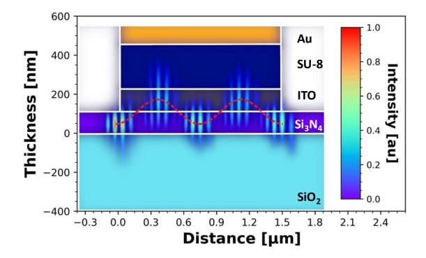
Figure 7.11: Fundamental waveguide mode in a  $1.5\mu$ m gold, SU-8, ITO, silicon nitride on glass modulator side-profile. The waveguide mode profile is imposed onto an illustration of the modulator with thicknesses and lengths shown. Intensity is shown by the colour scale on the right of the figure. The ITO has a refractive index of 1.9.
