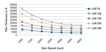
Figure 9.12: Photoresist thickness as a function of spin speed for lift-off resist (LOR) series [293].
