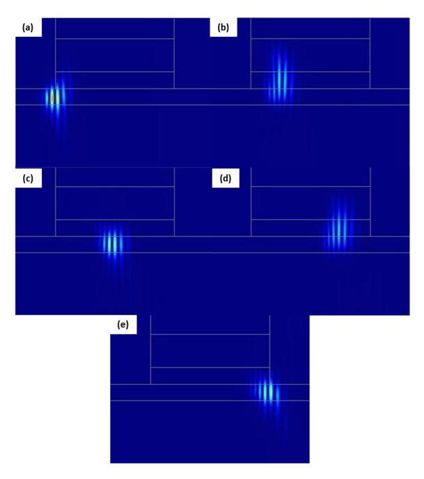
Figure 9.16: Fundamental waveguide mode in a  $1.5\mu m$  gold, SU-8, ITO, silicon nitride on glass modulator side-profile. The waveguide mode profile is shown at (a) the waveguide entry (b)-(c) travelling through the waveguide, and (e) exiting the waveguide. The ITO has a refractive index of 1.9.
