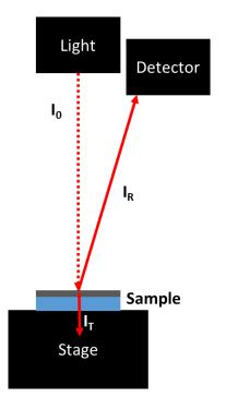
Figure 9.9: Illustration of a spectroscopic reflectometer.:
