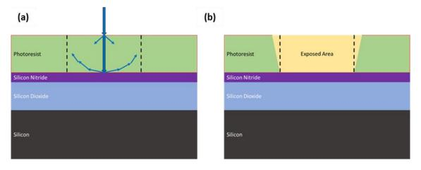
*Figure 5.4: (a) Interaction of UV with resist illustrating proximity effect and (b) the exposed area remaining.*
