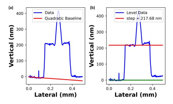
Figure 9.14: Surface profile analysis of SU-8 layer showing (a) distorted and (b) levelled surface profile.
