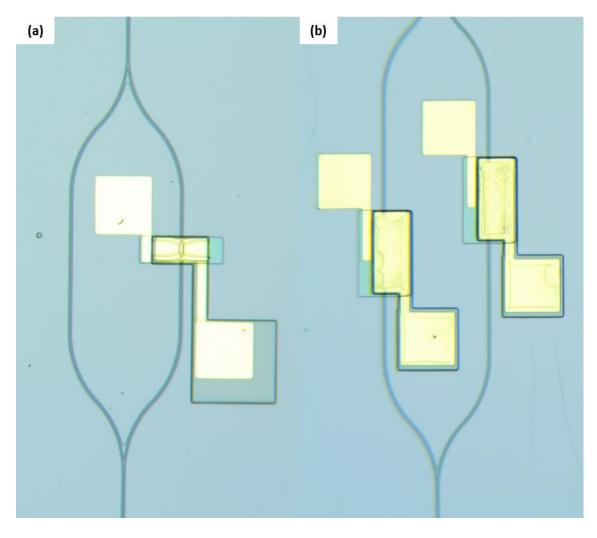
Figure 7.7: (a) Single and (b) double capacitor phase modulators.
