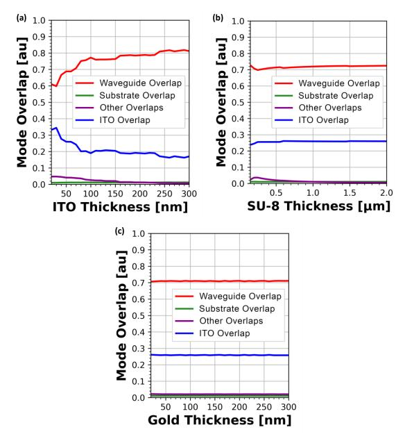
Figure 3.5: Mode overlap as a function of (a) indium tin oxide layer, (b) SU-8 layer, and (c) gold layer thickness.
