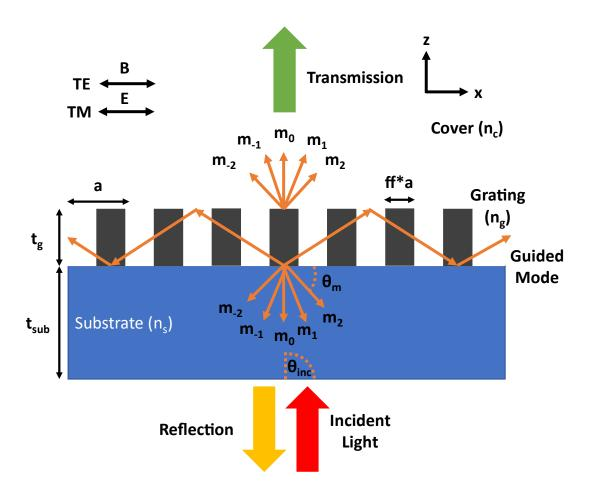
*Figure 2.3: Illustration of a typical 1D periodic structure used in this work, with guided and diffracted modes indicated.*
