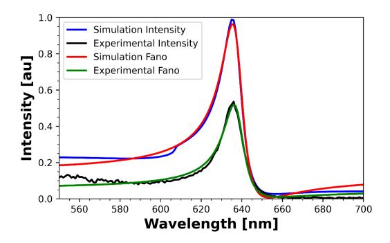
Figure 4.20: Comparison between simulated and experimental resonances for an ITO grating with fitted Fano resonances, found using minimising algorithm.
