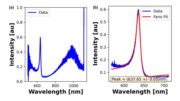
*Figure 4.17: (a) Raw spectrum from 1D periodic structure in ITO and (b) the fitted Fano resonance function with peak wavelength.*
