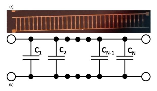
Figure 6.4: Metal-oxide-semiconductor capacitors in parallel, showing the (a) fabricated chip and (b) an illustration of the equivalent circuit.
