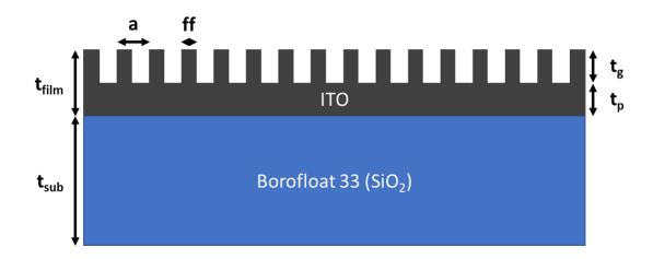
Figure 4.12: Schematic of 1D periodic structure in ITO showing some of the parameters that need to be known: substrate thickness ( $t_{sub}$ ), film thickness ( $t_{film}$ ), grating thickness ( $t_g$ ), waveguide thickness ( $t_{wg}$ ), grating period (a), and grating fill factor (ff).
