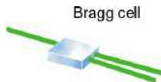
Figure 6.16 The Bragg cell used as a beam splitter[111]
