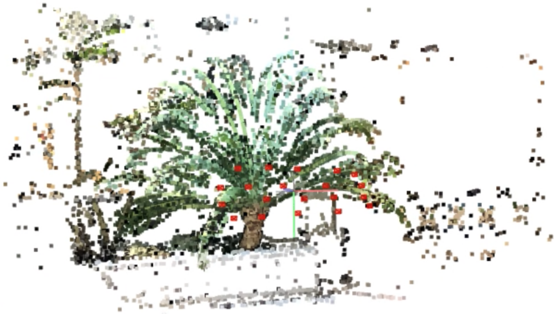
Figure 8.3: Generated point cloud and camera poses from COLMAP
