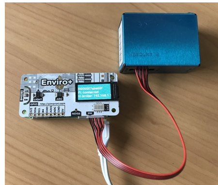
(B) Enviro+: A sample Indoor Air Quality Unit
