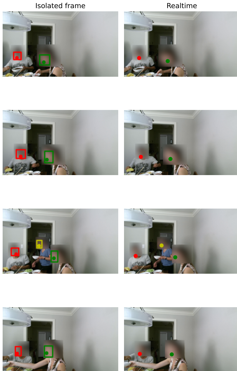
Fig. 3.7 The annotations on the left show bounding boxes and mouth positions annotated from the isolated frame tool. The annotations on the right show the corresponding frames in the real-time annotation tool. In the real-time tool, only mouth positions are annotated. The faces of the participants have been blurred to protect their privacy. When annotating the data, faces were visible.
