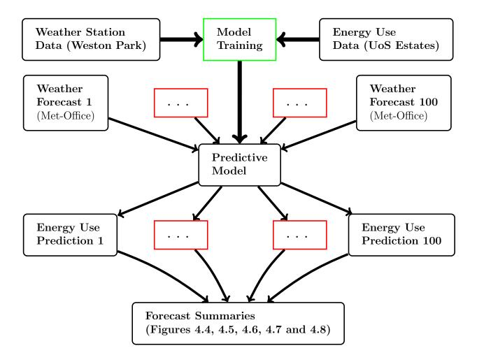
Figure 4.3: Work Flow Diagram: Sequentially the model i trained using the known energy use and recorded weather data, the resultant model is then used as predictive model for the weather forecasts to produce predictions, which are then summarised.
