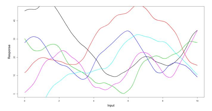
Figure 1.3: Samples from a Gaussian process prior distribution with squared exponential covariance functionplotted as lines as GP samples are continuous.. These are 'draws' from the prior distribution
