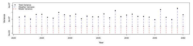
Figure 4.4: Predicted energy use for Chillers 1 and 2 combined. The 95% confidence plot has the international recognised baseline scenario for climate change Information Commons performance in light grey and the forecast energy use for 2021 to 2050 in black. The variance decomposition plot breaks down the sources of uncertainty into the variance from model performance, bottom, and weather uncertainty, top.
