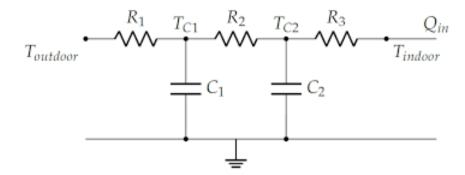
Figure 1.2: Formal capacitor network diagram representing a connection in figure 1.1 taken from Boodi et al. (2020), this case between indoor and outddor
