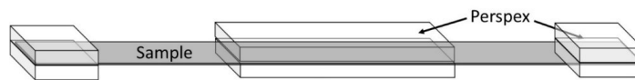
Figure 5.23: Illustration of four Perspex pieces securing the ends of the sample in the same manner as the two Perspex pieces in the middle. The Perspex pieces at the end of the sample are secured using a chemical adhesive.
