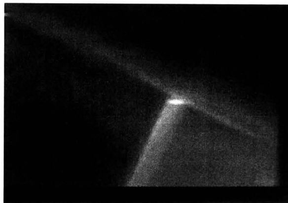
Figure 4.16: Experimental free surface and interface profiles for a 0.52 mm wide slot
