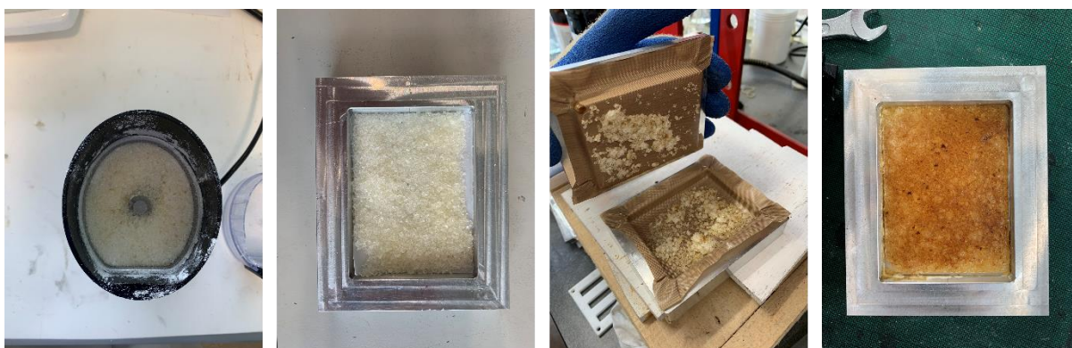
Figure 5-6 - Grinding and hot-press reforming of A1/HEMA/MMA networks.
