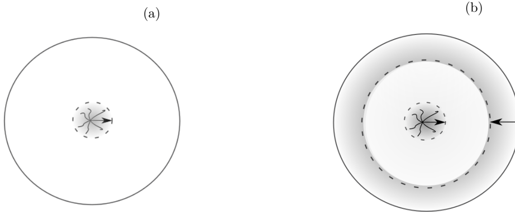
Figure 5.2: Propagation of radial and circumferential crack in the uniformly distributed loaded plate; (a) radial fracture initiated from the centre, (b) circumferential fracture initiated from the boundary and radial fracture initiated from the centre at later times
