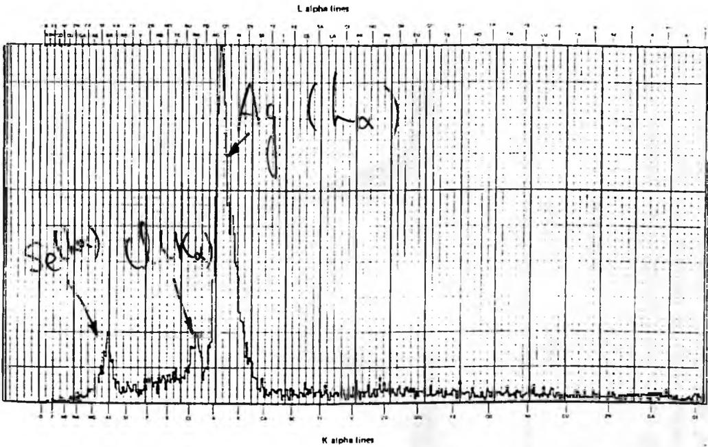
Figure 3.88 EDXA analysis reveals the formation of silver on  $\text{Ag}_2\text{Se}$  electrodes after cathodic polarisation for 5 minutes.
