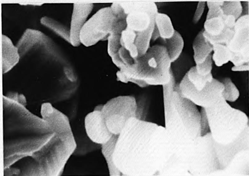
Figure 2.8 Scanning electron microscope (SEM) photographs of synthetic silver selenide ( $\text{Ag}_2\text{Se}$ ). Silver selenide crystals can be observed at relatively low magnifications. Magnifications: (a) 6500 x (b) 15000 x
