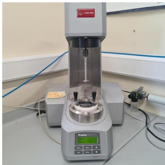
Figure 3-13 Anton Paar MCR301 rotational rheometer used for sample analysis.
