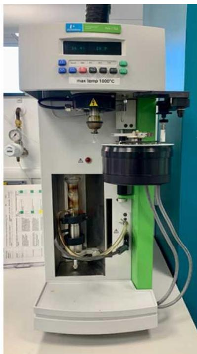
Figure 3-11 Perkin Elmer Pyris-1 TGA Instrument used for samples analysis.
