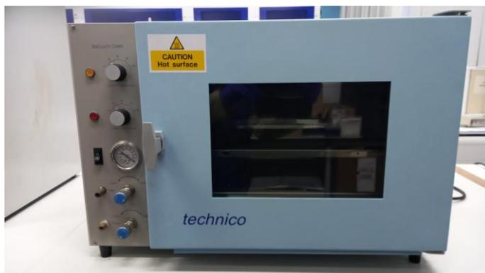
Figure 3-3 Technico™ Vacuum Oven used for drying samples.
