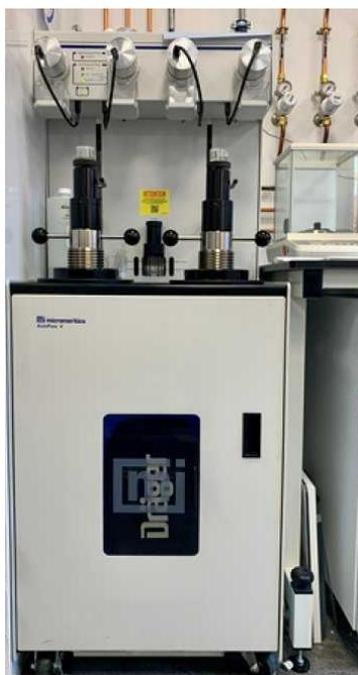
Figure 3-7 AutoPore 9620 porosimeter which was used for measuring the samples porosity based on the mercury porosimetry technique.
