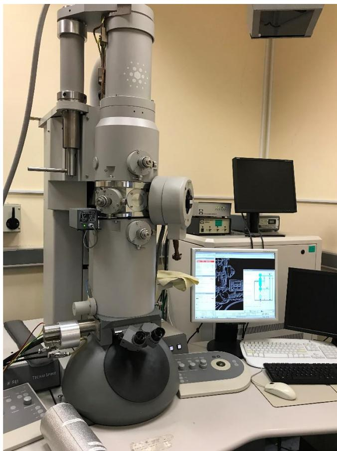
Figure 3-6 Transmission electron Microscopy unit used for imaging samples. (FEI Tecnai Spirit BioTWIN).
