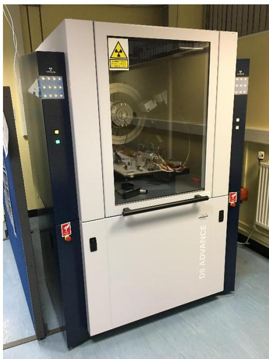
Figure 3-9 Bruker AXS D8 Discover X-ray Diffractometer (XRD) used for sample analysis (Bruker AXS GmbH, Karlsruhe, Germany).
