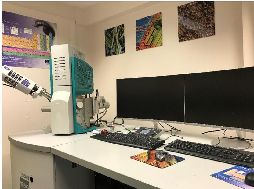
Figure 3-5 Scanning electron Microscopy unit used for imaging samples. (TESCAN VEGA3 LMU).
