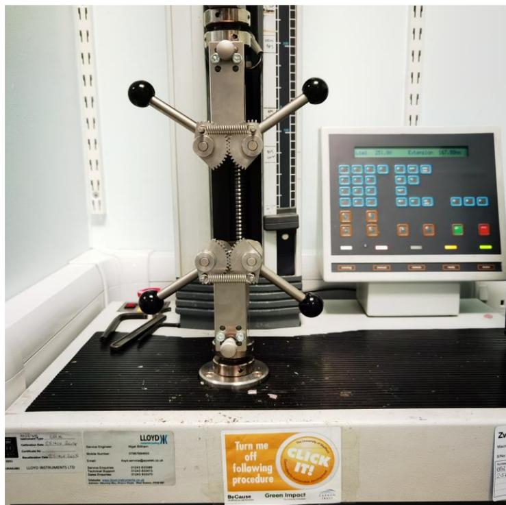
Figure 3-14 The universal testing machine used for measuring samples tensile properties.
