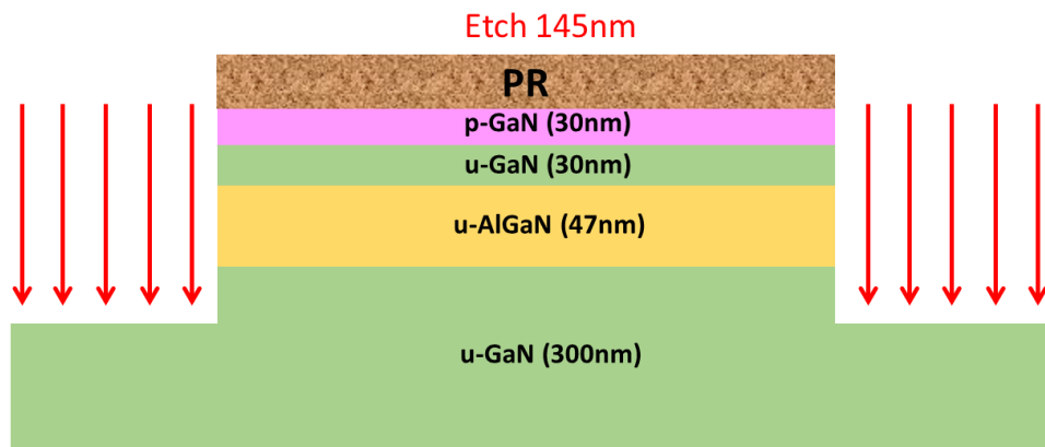
Figure 0.5 The schematic cross-section of devices after device Isolation etching.
