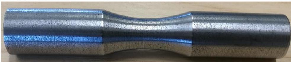
Figure 4-18 Example of the specimen used for the torsion experiments.
