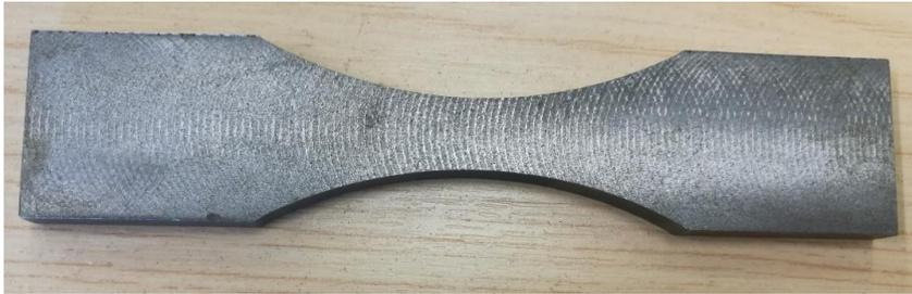
Figure 4-1 Example of plain specimen used for the static and fatigue test.
