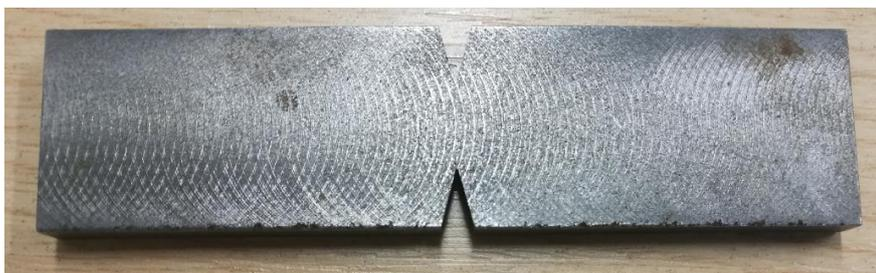
Figure 4-4 Example of the notched specimen used for fatigue test.
