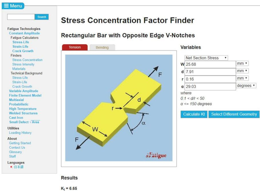
Figure C2 Calculation of the stress concentration factor at the notch tip of the material 40060.
