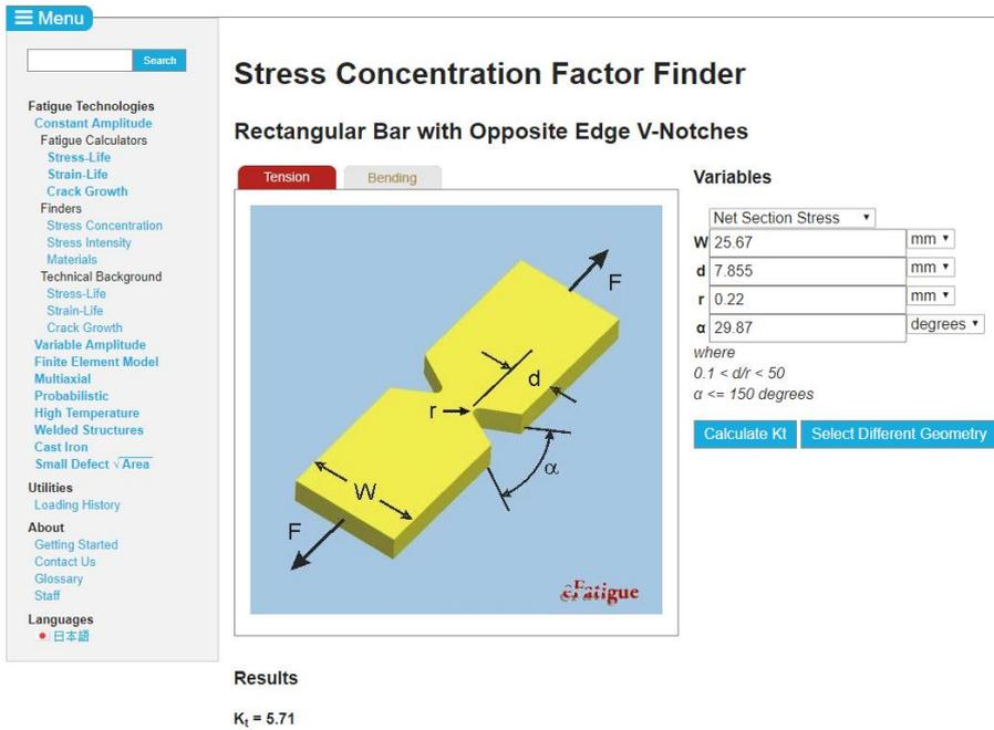
Figure C1 Calculation of the stress concentration factor at the notch tip of the material 40054.
