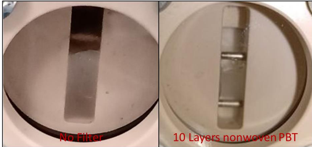
Figure 3.3 Images of the conductivity-controlled extractor with no filters present (left) compared to 10 layers of polybutylene terephthalate filter used (right).
