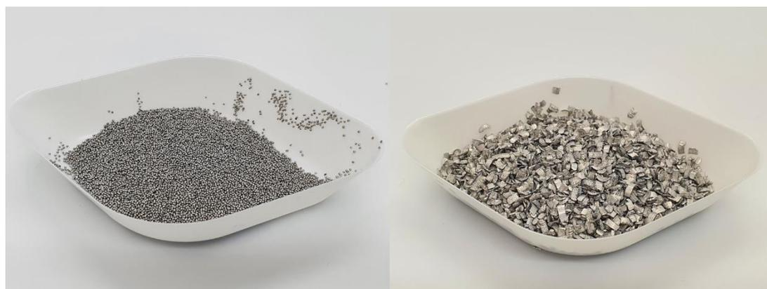
**Figure 6.1** Photograph showing a representative sample of Mg powder (left) and raspings (right) used to synthesise cement samples.
