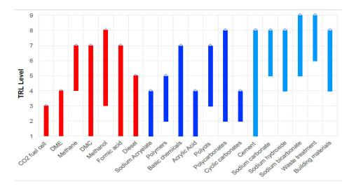
Figure 2.4 Technology readiness of various CO<sub>2</sub> utilisation products (Wilson et al., 2015a). Fuels are coloured red, chemicals and polymers dark blue and carbonates light blue.
