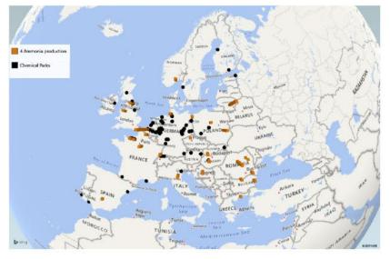
Figure 3.9 Locations of emissions of CO<sub>2</sub> from ammonia production facilities in Europe. Adapted from E-PRTR.
