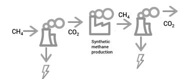
Figure 3.14 Following the carbon atom in producing synthetic methane from fossil methane
