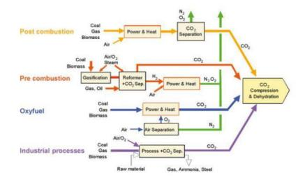
Figure 3.2. CO<sub>2</sub> capture technologies (Moazzem et al., 2012).
