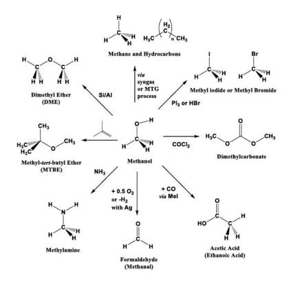
Figure 2.3 A selection of synthetic uses for methanol. Dowson and Styring (2014)
