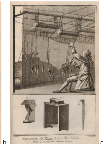
Fig. 4) The weaving looms and the manipulation of “haute-lisse” (perpendicular) warp threads in the royal Gobelin manufactory as illustrated in the Encyclopédie (1751-1772), vol. 26, respectively plates I, VI, IX.
