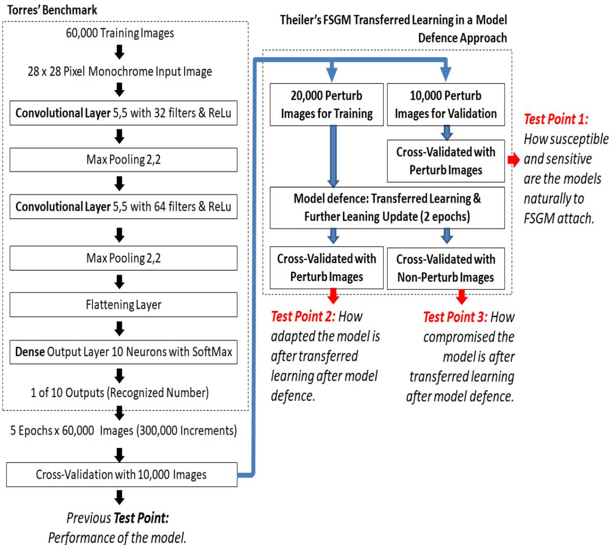
FIGURE 39 EXPERIMENT MODEL FOR AN ANALYTICAL METHOD WITH FSGM [J1]
