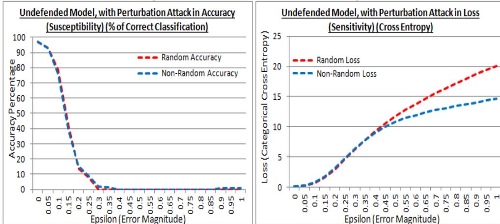
FIGURE 41 TEST POINT 1: ACCURACY AND LOSS WITHOUT TRANSFERRED LEARNING [J1]
