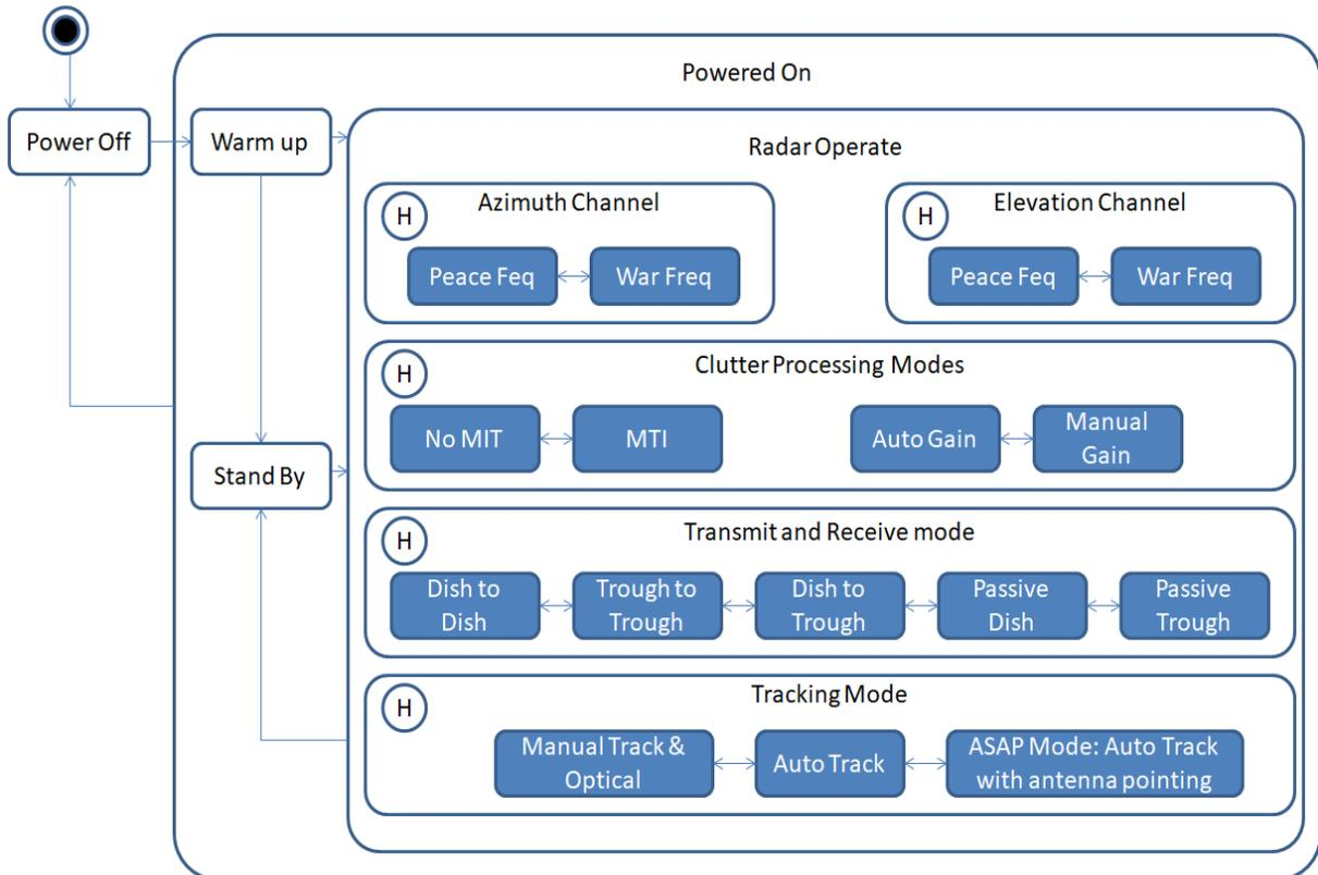
FIGURE 15 UML S-75 STATE DIAGRAM [J5]
