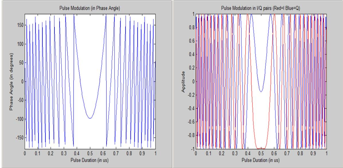
FIGURE 60 WAVEFORM MODULATION LINEAR CHIRP EXAMPLE (TEST MODULE)
