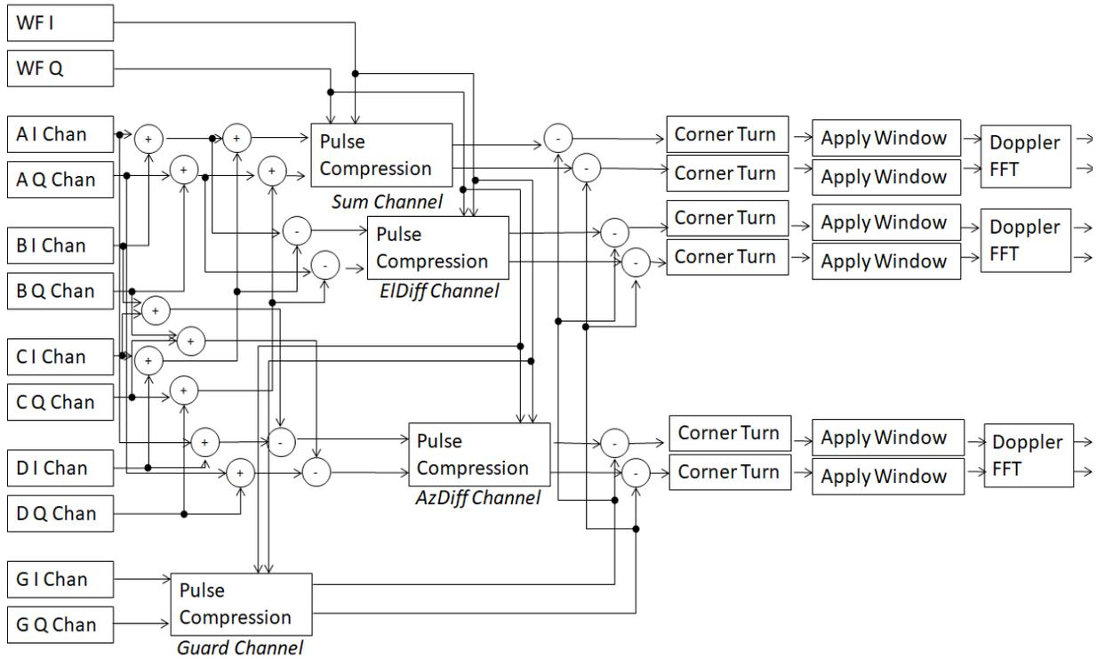
FIGURE 14 SIGNAL AND PROCESSING BLOCK DIAGRAM [J5]
