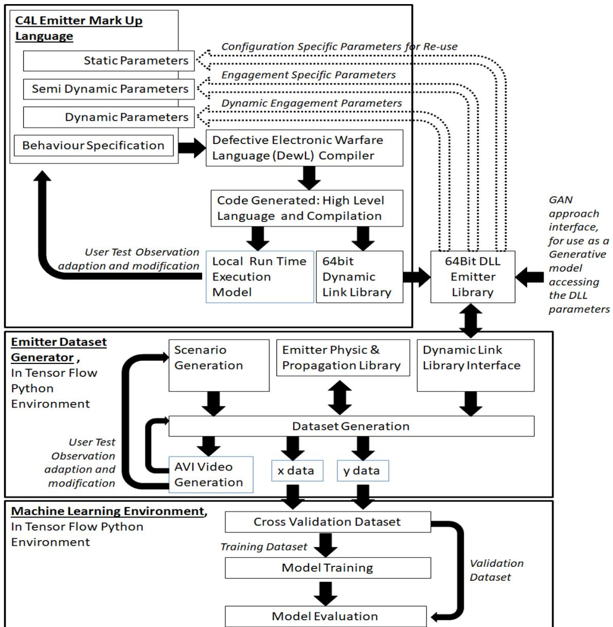
FIGURE 46 SYNTHETIC EMITTER DATASET GENERATOR ARCHITECTURE
