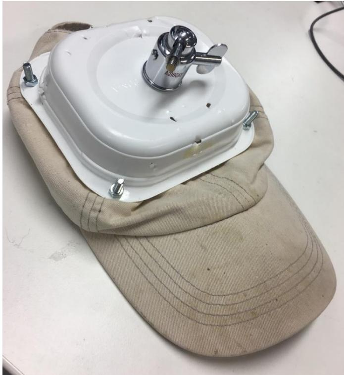
*Figure 17: A modification of the pole-mounted camera modifying an old baseball cap with a camera mount.*
