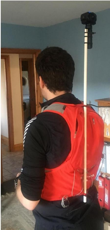
**Figure 16:** Pole-mounted camera attached to a running bag with cable ties used for the second trial method.
