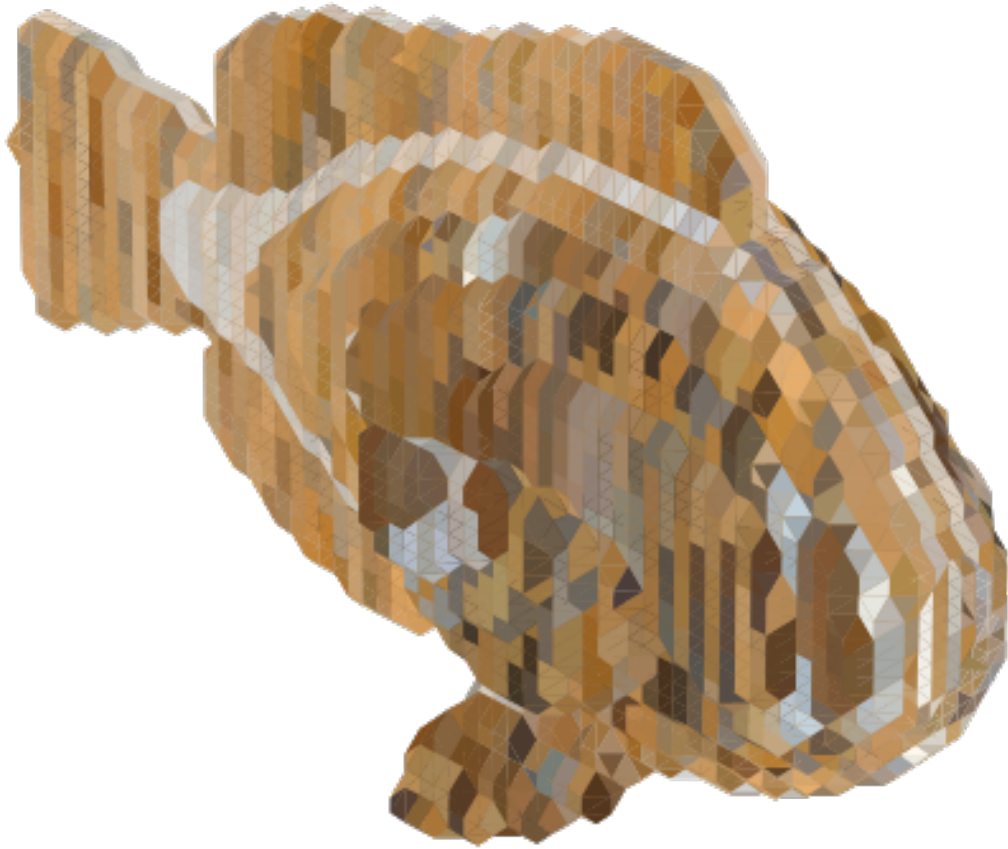
Figure 7.6: Low resolution mesh conversion using marching cubes with extrapolated face colours from a network generation.
