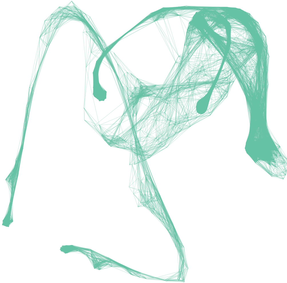
Figure 7.2: A 1.0 scale point cloud from human mesh, represented in a connected non directional graph of closest points N where N < 0.1 . The vague outline of a non euclidean human form can be made out within the graph.
