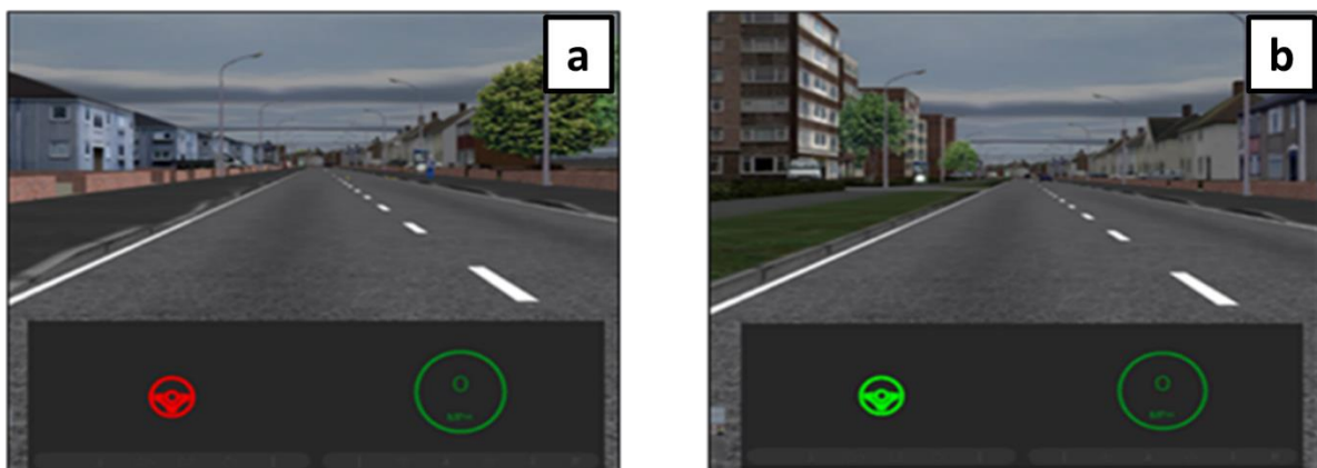
Figure 5.1. HMI Interface on the dashboard: (a) when automation was disengaged; (b) Automation was engaged.
