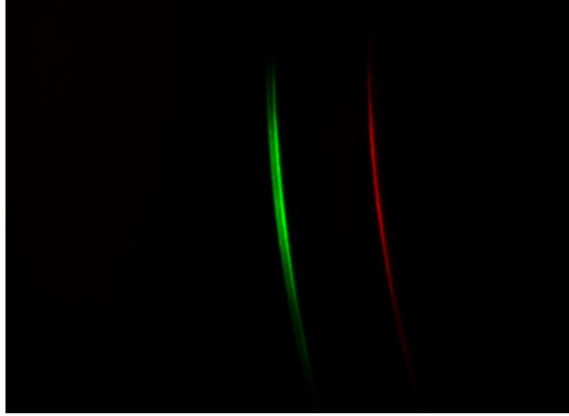
Figure 2.9. Distorted spectral lines. Note, the curve of the spectral peaks. This can create complications within the calibration process due to the shifting linear location of the spectral peaks.
