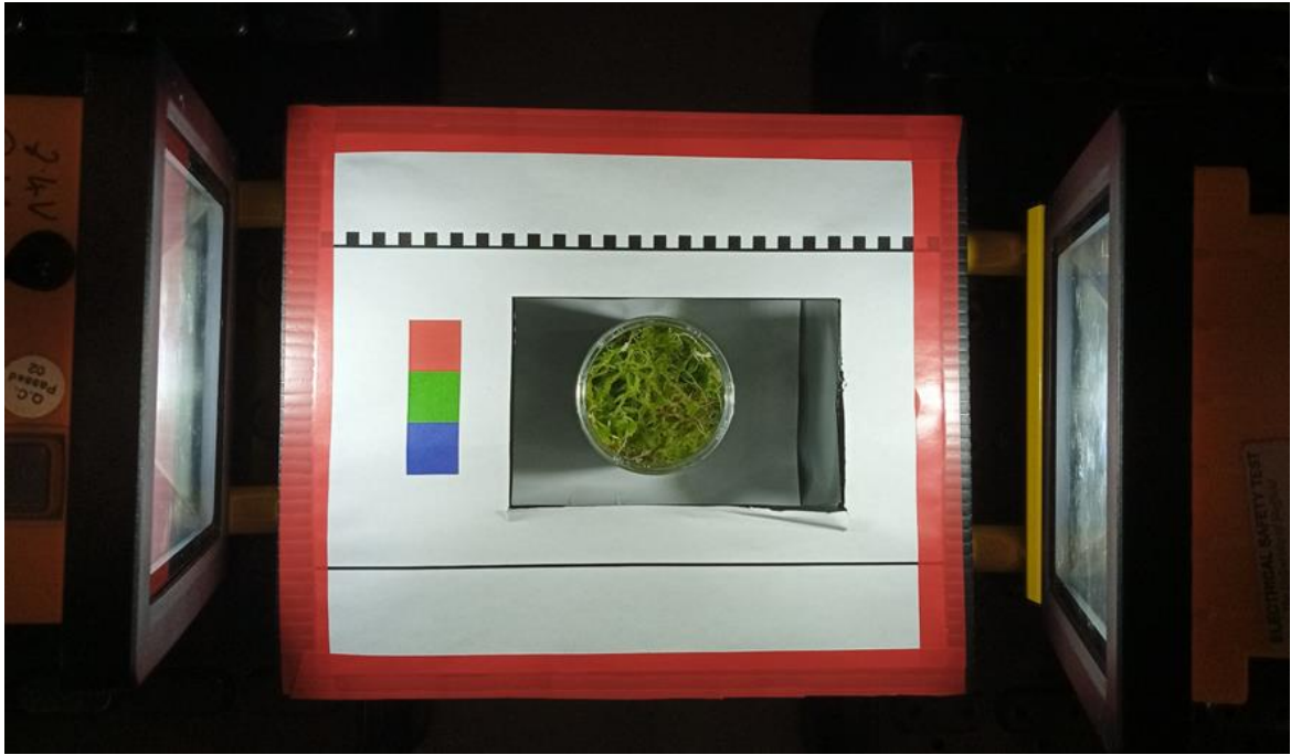
Figure 4.22 A sample of Sphagnum moss ready for image capture using the hand-held Hyperspectral Smartphone and the in-scene reference card. Illumination is provided by two 20 W LED lamps.
