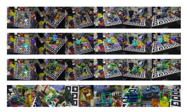
Figure 4.9: Qualitative results on Occluded LINEMOD. First row: the original images. Second row: the predicted object class, 2D bounding box and instance segmentation (different color means different class). Third row: 6D pose represented by 2D projection contour which green is the ground truth and the other color is estimated. Fourth row: Area screenshot, the first three columns is success cases and the last three columns is fail cases.
