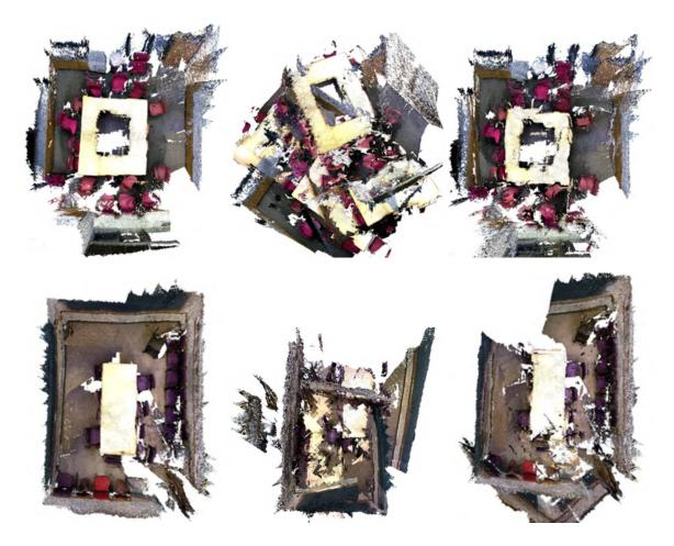
Figure 3.10: Reconstruction of scenes from the SUN3D Dataset. First column: ground truth. Second column: pose graph method [11]. Third column: proposed approach
