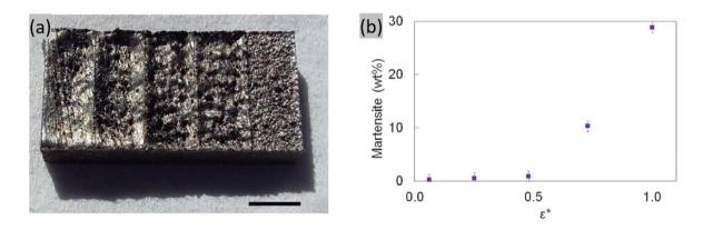
Figure 6.8: (a) Spatially graded 17-4PH showing rough surface in the high thermal strain region (austenite + martensite) and smooth surface in low thermal strain region (fully austenitic) (b)Relationship between the weight percent of martensite and the process driven thermal strain term [50].
