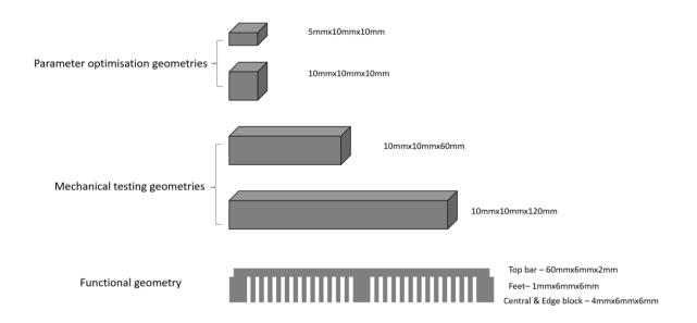
Figure 3.1: Geometries utilised in this study. Cuboids were mostly used for design of experiment purpose and can be further cut-off for microscopy investigations. Tensile bars were extracted from bar structures. The presence of as-built residual stress was revealed by the cantilever structure.
