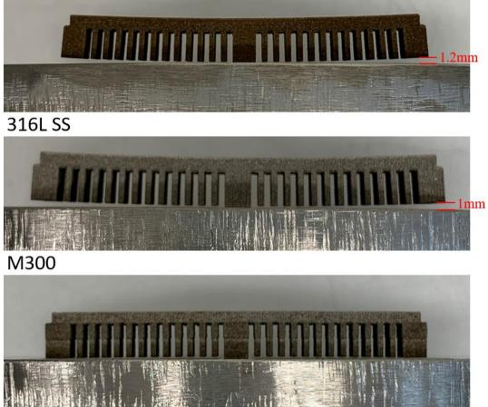
Figure 6.3: By measuring the gap of distortion, it can be seen that Fe-Mn TWIP steel displays the highest magnitude of distortion after cut-off. This is closely followed by 316L SS which shows a similar level of angular distortion. Meanwhile, the M300 shows no distortion.
