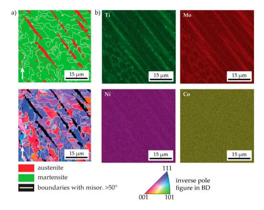
Figure 5.12:a) EBSD phase map and IPF map of LMD-built M300 maraging steel, FCC austenite is coloured in red and BCC martensite is coloured in green. b) Elemental segregation maps showing clear segregation of Ti, Mo and Ni at cell boundaries. The location of the segregation site matches to the location where austenite phase is indexed in a) [90].
