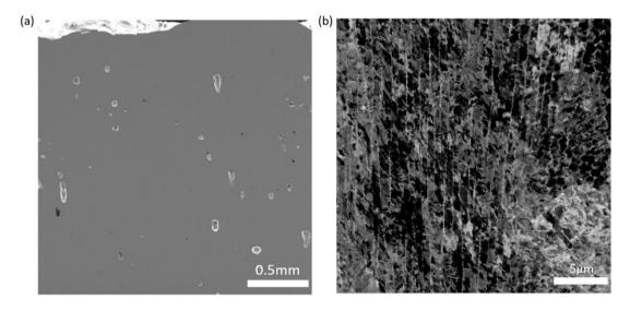
Figure 5.1: (a)Secondary electron micrograph showing the distribution of keyhole type defects in as-built M300. (b)Backscattered electron micrograph of as-built M300 showing solidification cell structures. Cell boundaries are highlighted due to the presence of retained austenite.
