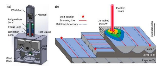
Figure 2.2: Schematic graph of an Arcam EBM device, a set of magnetic lenses guides the electron beam through to the build chamber. b: Typical build scenario with EBM. The overlap of melt pools are illustrated with dashed lines [2].
