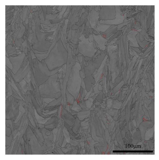
Appendix Figure 10: EBSD boundary characteristic map of additively manufactured 316L SS.  $\Sigma$ 3 boundaries are coloured in red.
