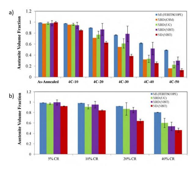
Figure 5.16: Remaining volume fraction of austenite in a deformed/rolled metastable austenitic steel obtained with magnetic induction, X-ray diffraction and neutron diffraction. a)shows the results of samples deformed to different engineering strain at 4°C. The results obtained in samples rolled to different levels of thickness reduction is illustrated in b) [94].
