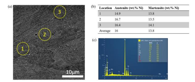
Figure 5.6: (a) Backscattered micrograph of the site of EDS point analysis. (b) Nickel content in grey (austenite) and black (martensite) islands, a clear enrichment of nickel in austenite can be seen. (c) Typical EDS spectrum of the point index, high carbon content is caused by the deposition during EBSD mapping.
