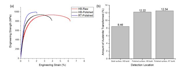
Figure 5.9: (a)Engineering stress/strain curve of room temperature and HB built M300 steel. Lower yield and tensile strengths are registered by the HB built specimens. (b) Transformation of austenite during tensile testing.
