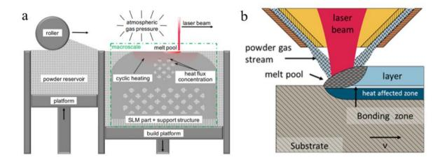
Figure 2.1: a typical setup of a powder bed fusion system with indication of melt region and operating environment [10]. b: Experimental set up of a laser powder deposition System [3].
