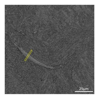
Figure 7.3: EBSD band contrast figure showing the location of the austenite crescent. FIB lift out position is highlighted in yellow.
