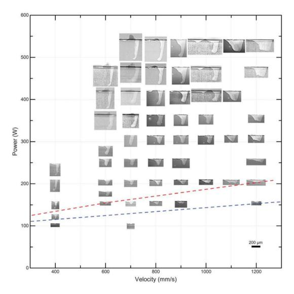
Figure 2.9: Plot showing how power and scan speed of the laser affects the shape of the keyhole. Note the conduction mode melt pool below the blue line [10].
