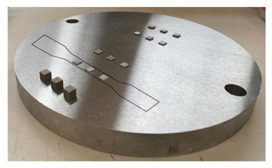
Figure 7.5: The M300 cladding deposited in Aconity Mini and the proposed shape of tensile specimen for sensor testing.
