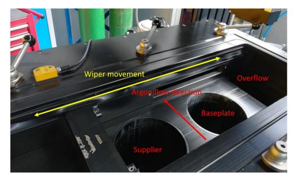
Figure 3.2: Processing chamber of the Aconity Mini. The supplier sits in front of the baseplate column. Each layer the wiper blade brings new power from raised supplier platform to the lowered baseplate platform. Excess powders are swept to the overflow.
