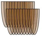
Figure 5.14: Schematic drawing of the effect of keyhole type melt pool. Not only does the melt pool penetrate further into the previous layer, the effect of  $30\mu m$  hatch spacing is further magnified.
