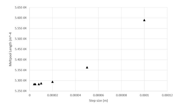
Appendix Figure 8: Sensitivity test of the MATLAB script utilised in this study. A step size of 0.000005 is chosen.
