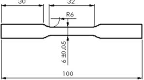
Appendix Figure 2: Dimensions of the larger tensile bar tested in Chapter 4 and 5.
