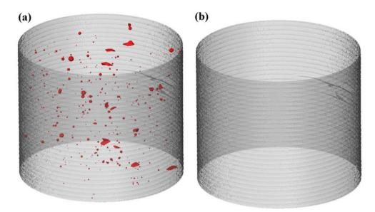
Figure 7.1: Effect of hot isostatic pressing on the defect volume of an additively manufactured part [13].
