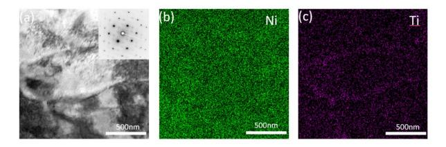
Figure 5.4: (a) BF-STEM micrograph showing the outline of a dislocation cell. Insert SAD shows the [110] BCC zone axis with weak response of precipitates and largely confident fully martensitic matrix. (b) and (c) STEM EDS maps showing the segregation profile of Ni and Ti, respectively.
