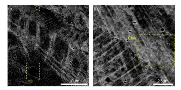
Figure 4.17: Backscattered electron micrographs showing cavities and remaining dislocation cells in L-PBF built TWIP steel strained to 25%.
