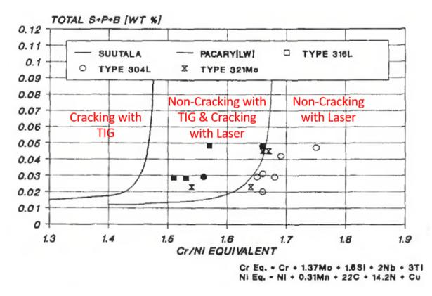
Figure 2.11: Modified Suutala diagram of pulsed laser welding. Note the shift in trend line between the laser welding result and TIG welding condition [22].
