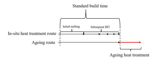
Figure 5.15: Two methods of obtaining additional austenite in additively manufactured M300. In-situ heat treatment route involves heat treating the sample through subsequent layers, whereas the aging route revert austenite after the AM process.
