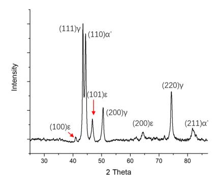
Figure 4.6: XRD spectrum of as-rolled TWIP steel sheet. Both transformation products ( $\epsilon$  and  $\alpha$ ') can be seen.
