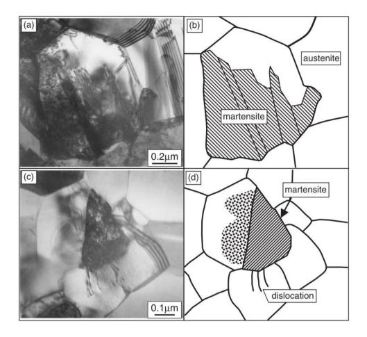
Figure 4.19: Transmission electron micrographs and corresponding drawings of the morphology of martensite inside (a)fine and(c)ultrafine austenite grains. With approximately 1  $\mu$ m grain size, multiple laths with similar orientation are formed. When the grain size is further refined below 1 $\mu$ m, a single lath of martensite is formed [82].
