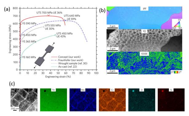
Figure 2.17: (a): Mechanical properties of additively manufactured 316L compared to conventionally processed counterparts. (b): Precession electron diffraction images showing large grains and sub-micro dislocation network in as-built 316L SS. (c): STEM EDS segregation map showing Mo and Cr segregation at low angle grain boundaries [16].
