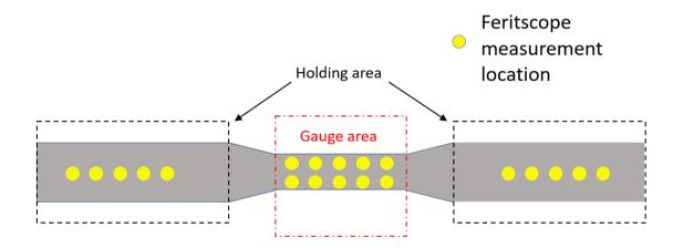
Appendix Figure 4: Schematics of the Feritscope testing procedure of M300 tensile specimen.
