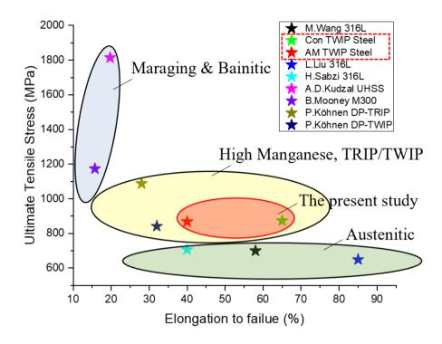
Figure 4.21: Performance comparison between the known studies of L-PBF built steels and the present study. The steels designed in the present study shows improved ultimate tensile strength when compared to legacy austenitic stainless steels and superior ductility in comparison to previously reported additively manufactured high manganese steels [16][33][84][46].
