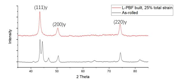
Figure 4.15: XRD spectrum comparison between strained L-PBF built tensile bar and severely deformed TWIP steel. Absence of transformation product can be seen in the L-PBF built steel. Peaks in the as-rolls sample are labelled in Fig 4.6.
