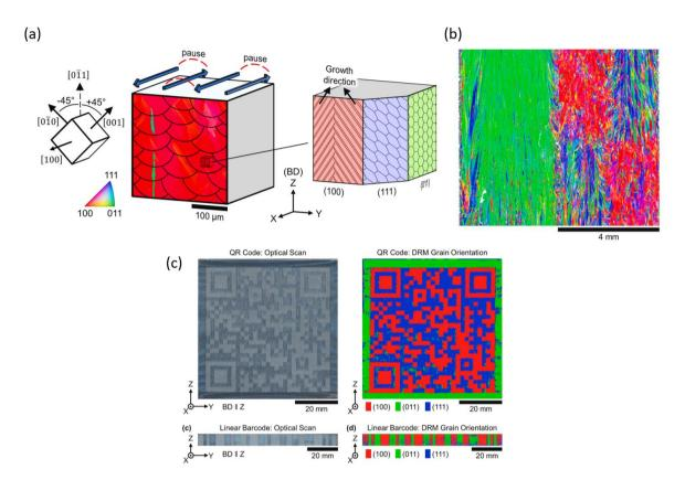
Figure 2.19: (a) Crystal orientation and supposed melt-pool morphology of additively manufactured 316LSS under texture control. (b)EBSD IPF map of texture controlled 316LSS. Large blocks of grains are successfully grown in the same orientation. (c) Optical and directional reflectance microscopy micrograph of etched surface showing a QR code [37].
