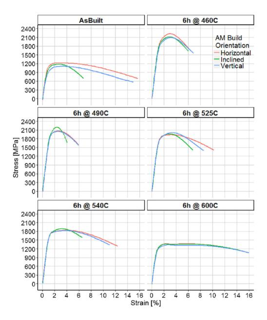
Figure 2.22: Engineering stress-strain curves of as-built and heat treated M300 samples. A trade-off between peak strength and elongation to failure can be clearly seen between as-built and aged samples. Inclined samples (coloured in green) exhibit overall inferior mechanical performance [46].
