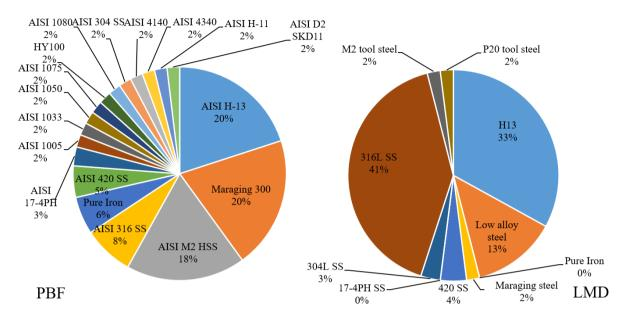
Figure 2.16: Two pie charts showing the grades of steels studied with powder bed fusion and laser metal deposition, despite the similarity in composition. Reproduced from [4].
