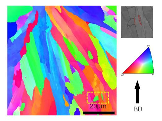
Figure 4.9: EBSD IPF-Z of as-built TWIP steel. Large aspect ratio grains contain neighbouring elongated cells with low misorientation angles. A site in the bottom right corner of the IPF containing  $\Sigma$ 3 boundaries highlighted in red is shown in the top right corner.
