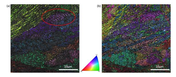
Appendix Figure 3: IPF of (a) austenite and (b) combined phases in aged M300 sample. Area circled in red shows near-single variant transformation.
