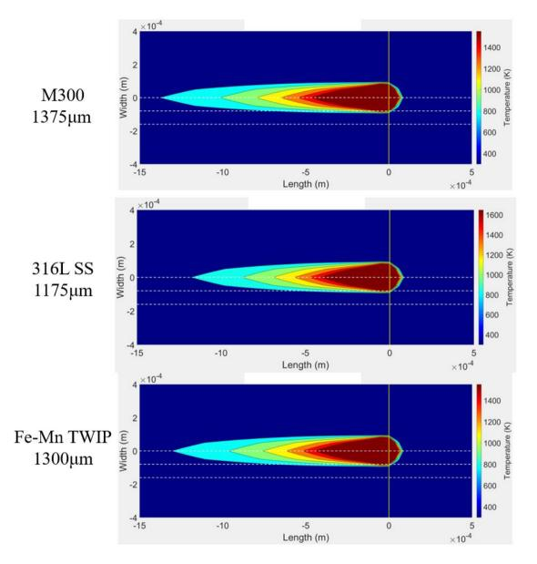
Figure 6.6: Melt pool length simulated with the Matlab script. Overall similar melt pool lengths are observed in all three steels.
