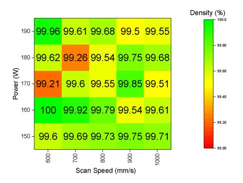
Figure 4.7: Density measured from cubes built in the DoE. All samples registered above 99% density indicate that the proposed TWIP steel exhibits good printability.
