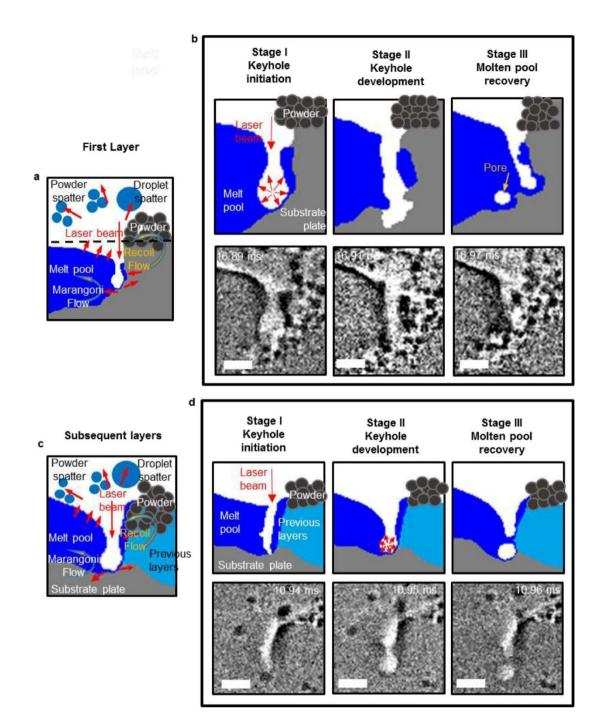
Figure 2.8: In-situ observation of keyhole melt pool in L-PBF built Ti-6Al-4V. The evaluation of the melt pool was separated into three stages. The first stage mainly involves the establishment of the keyhole melt pool [11].
