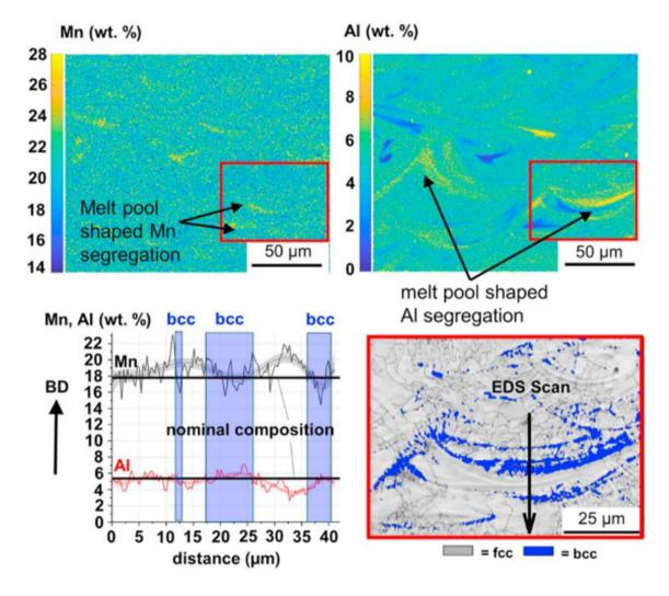
Figure 5.13: EDS maps of additively manufactured Fe-Mn-Al-C steel showing clear presence of band-like structures. EDS Line analysis shows coupled depletion of Mn and enrichment of Al in BCC phase areas, with corresponding EBSD phase map showing the location of measurement area [81].
