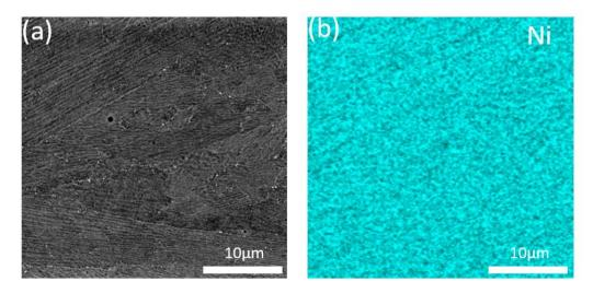
Figure 5.7: (a) Backscattered electron micrograph of aged sample. High contrast particles are precipitates. (b) SEM EDS map of Ni.
