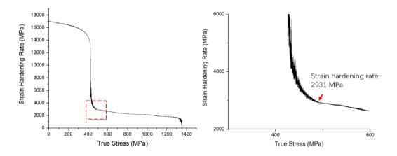
Figure 4.4: Kocks-Mecking analysis of conventionally manufactured TWIP steel.
