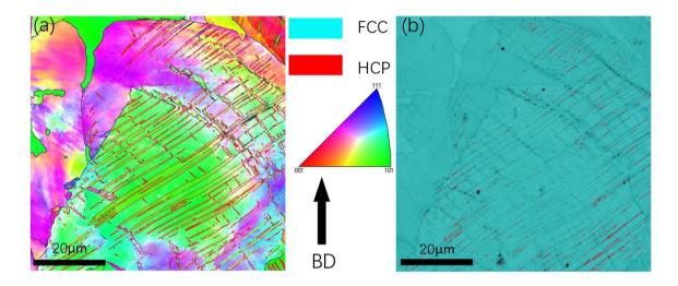
Figure 4.14: (a) EBSD IPF with  $\Sigma 3$  grain boundaries highlighted in red showing the distribution of deformation twins in the TWIP steel sample strained to 25%. (b) Phase map of L-PBF built TWIP steel showing the presence of  $\varepsilon$ -martensite formed in twin bands.
