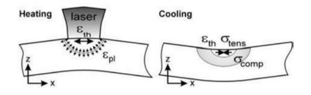
Figure 2.12: Modes of residual stress in relation to the rapid heating and cooling during the L-PBF process [26].
