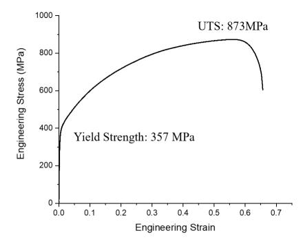
Figure 4.3: Engineering stress-strain curve of cold-rolled & annealed TWIP steel.
