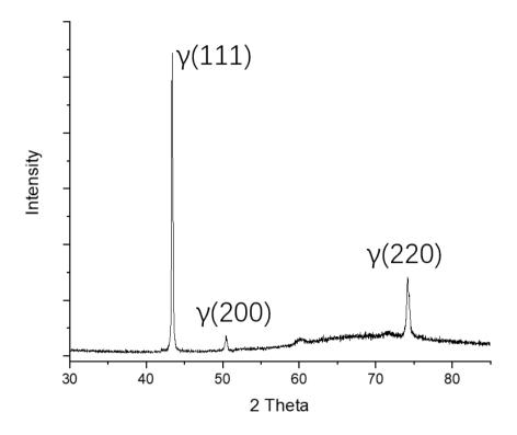
Figure 4.10: XRD spectrum taken from as-built TWIP steel. Note the higher intensity in (220) FCC peak.
