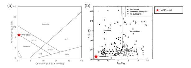
Figure 4.1: (a) Schaeffler diagram prediction based on the composition proposed for this study, the present composition is predicted to yield austenite and martensite in the weld region. (b) Original Suutala diagram showing that the present TWIP steel is susceptible.
