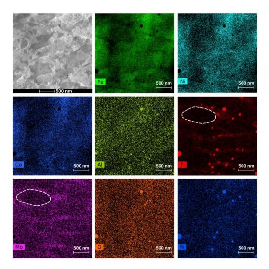
Figure 2.21: STEM EDS segregation maps of additively manufactured MS1 maraging steel. By comparing with the bright field STEM image at the top left corner, strong Mo cell-boundary segregation can be observed in bottom left map of Molybdenum. High density of Ti-Al nanoparticles is also observed in corresponding segregation maps [44]. The outline of a cell is circled in white.
