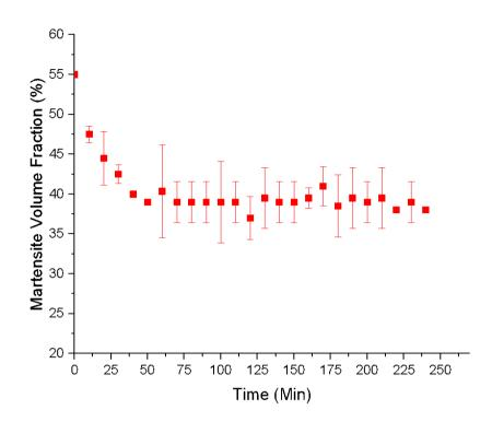
Figure 5.8: Recovery in austenite during the ageing heat treatment of M300 Rapid recovery of austenite can be seen in the first 40 minutes of ageing. The recovery process terminates after 50 minutes of ageing as the maximum austenite stability is reached. Further holding led to homogenisation and dissolution of cell boundaries which caused the fluctuation in readings.
