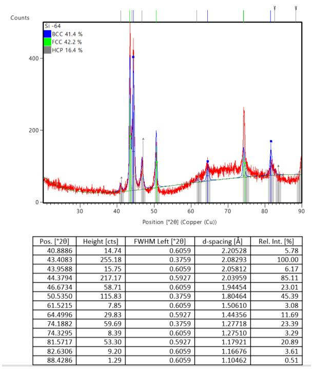
**Appendix Figure 9: Rietveld refinement calculation results and the peaks used in the calculation.**
