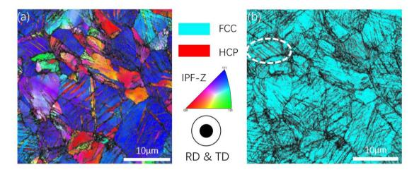
Figure 4.5: (a) EBSD IPF-Z of fractured TWIP steel. High density of deformation bands can be seen in the microstructure. (b)EBSD phase map of fracture sample, red deformation bands circled in white in the top left corner of (b) are indexed as  $\varepsilon$ -martensite.
