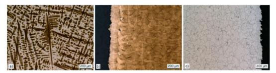
Figure 7.2: Microstructure of as-cast, additively manufactured and AM+HIP CoCrMo alloy [101].
