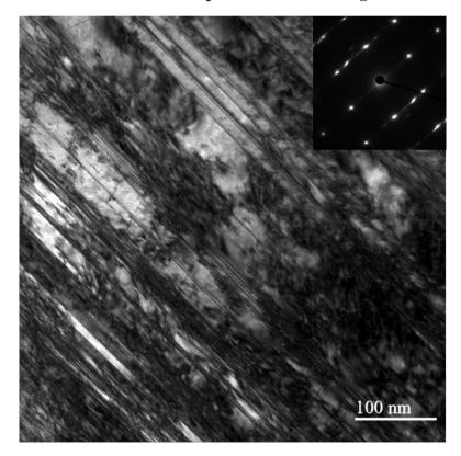
Figure 4.16: Bright field TEM micrograph showing high density of deformation twinning and dislocation forests. SAD insert shows diffraction spots of the FCC matrix and twin. Image taken in [110] zone axis.
