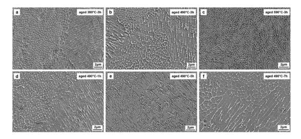
Figure 2.23: Secondary electron micrographs showing the partially dissolved dislocation network in M300 after substantial ageing heat treatment [49].
