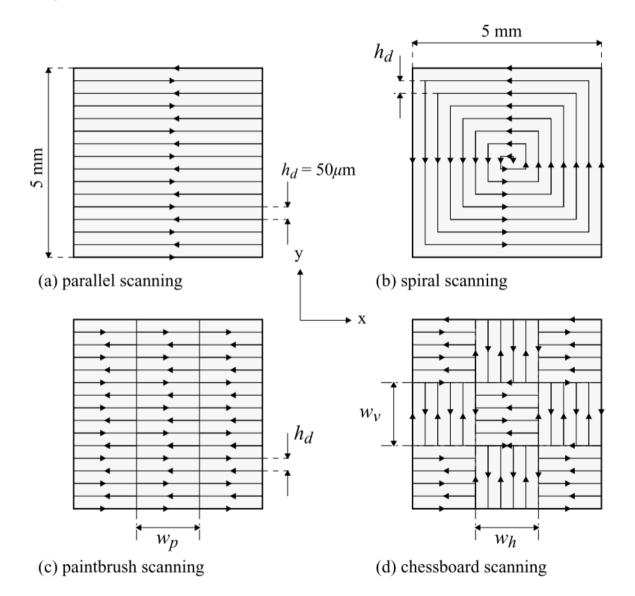
Figure 2.3: Visualisation of scanning strategies. Poor overlap or miss-alignment of islands in the strategy shown in (c) and (d) can lead to severe cracking [6].
