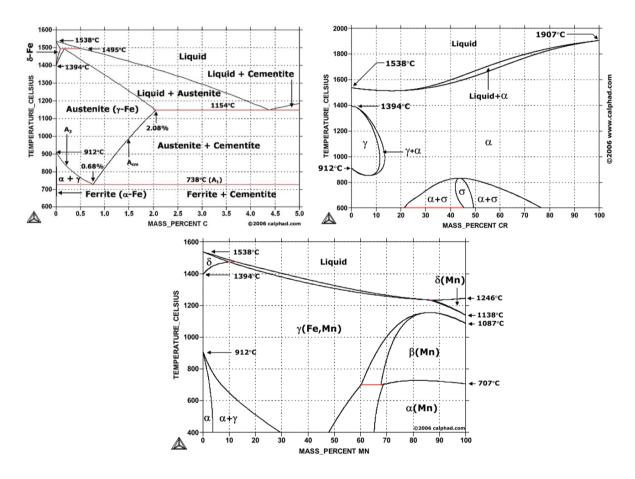
Figure 2.14: Typical Fe-C, Fe-Cr and Fr-Mn phase diagrams [28][29][30].
