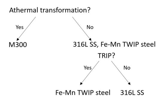
Figure 6.1: Alloy selection in the study based on where a steel can undergo athermal or deformation driven transformation.
