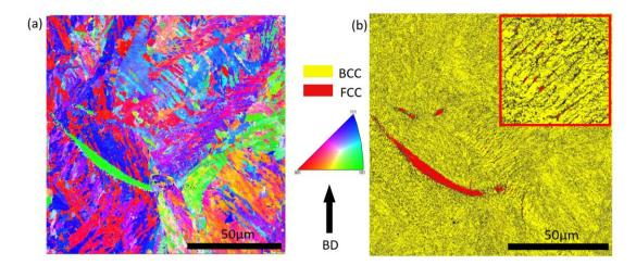
Figure 5.2: (a) EBSD IPF and (b) phase map of as-built M300. Insert in (b) shows a magnified region where distribution of retained austenite can be seen. The colouring of phases is shown in the legend. ImageJ calculation shows around 6.9% of austenite is present in b).
