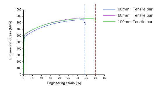
Figure 4.18: Engineering stress strain curves showing the size effect in L-PBF built TWIP steel.
