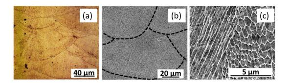
Figure 2.20: (a) 2% nitric acid etched optical micrograph of as-built M300 maraging steel. (b) SEM micrograph showing the melt pool boundaries. (c) Close up SEM micrograph showing dislocation cells [43].
