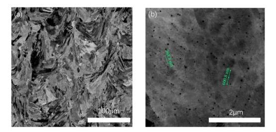
Figure 4.8: (a) Back scattered electron micrograph of as-built TWIP steels taken in the build direction. (b) Dislocation cell structure in the as-built TWIP steel. Nanometre sized gas pores can be seen in (b).
