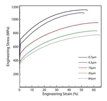
Figure 2.25: Engineering stress strain curve of TWIP steels with different grain sizes. Smaller grains lead to higher yield strength and slight reduction in plastic strain [54].
