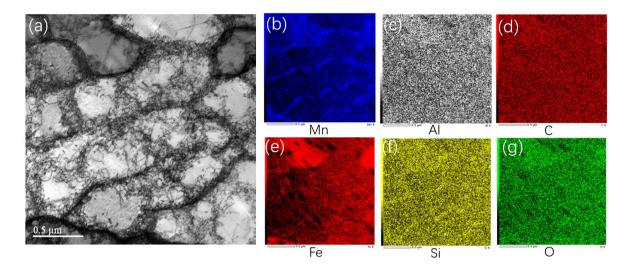
Figure 4.12: Bright field STEM image and EDS maps of the as-built TWIP steel. Strong segregation of Mn can be observed in (b).
