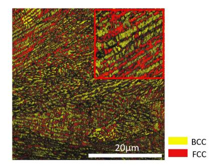
Figure 5.5: EBSD phase map of M300 heat treated at  $600^{\circ}$ C for 24hrs. Insert shows partial dissolution of cell boundaries. Map acquired at a step size of  $0.1\mu$ m. ImageJ calculation shows 13% of austenite is present.
