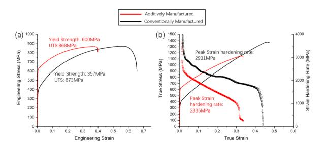
Figure 4.13: (a)Engineering and true stress strain curves of conventionally and additively manufactured TWIP steel, the trade-off between ultimate tensile strength and ductility can be seen in the AM built TWIP steel. (b) True stress-strain curve combined with strain hardening rate analysis showing the lower peak strain hardening rate of additively manufactured TWIP steel, as well as the steep decline in strain hardening rate.
