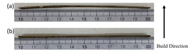
Figure 6.4: EDM sectioned M300 tensile bars. Significant distortion can be seen in (a) which is the top surface of the build part. Meanwhile, the tensile bar (b) sectioned below the build surface shows no distortion.
