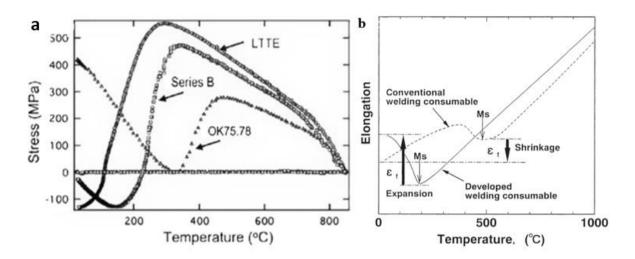
Figure 2.29: a: Comparison of welding electrodes with different Ms and its influence on the residual stress [66]. b: Schematic diagram showing the improvement made by reducing Ms [67].
