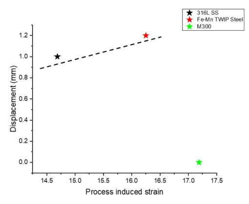
Figure 6.7: Relationship between thermal strain term and the cut-off distortion observed in cantilevers. While the austenitic steels exhibit large displacement due to the thermal strain, M300 shows no distortion due to its self stress-relief capability.
