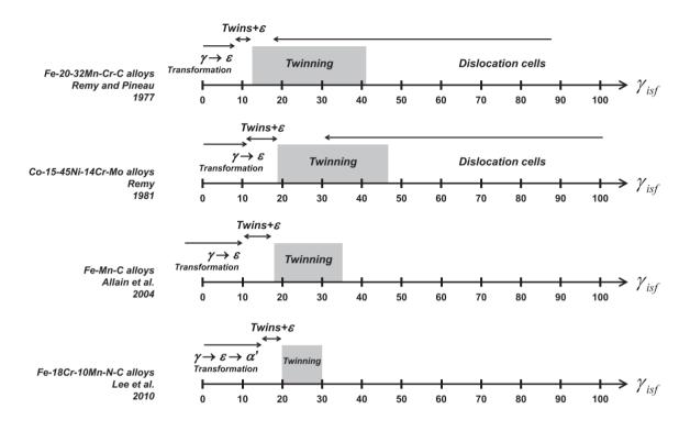
Figure 2.24: A series of studies showing how changing the chemistry can alter the deformation mechanism [57].
