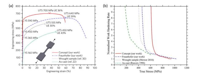
Figure 4.20: (a) Engineering stress strain curves of additively manufactured 316LSS. (b)Kocks-Mecking analysis of data presented in (a) showing a different strain hardening behaviour. Peak strain hardening rates were obtained after yielding and a steady decrease can be observed [16].
