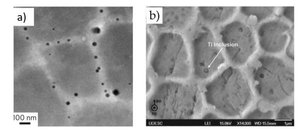
Figure 2.10: a) SiO inclusion observed in as-built 316LSS. b) TiO inclusion in aged M300 maraging steel [16][17].
