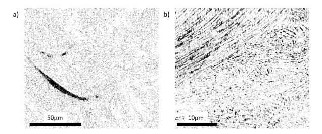
Appendix Figure 7: 8-bit processed EBSD phase maps of a) as-built and b) 24hrs aged M300 maraging steel for ImageJ area fraction analysis.
