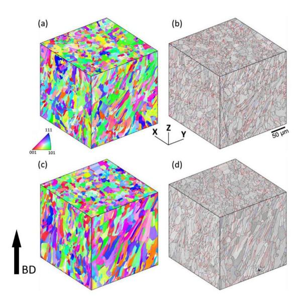
Figure 2.18: EBSD IPF showing the distribution of  $\Sigma 3$ (red) and  $\Sigma 9$ (blue) boundaries in (a)(b) as built and (c)(d) annealed status of 316L SS [34]. The build direction is annotated as BD.
