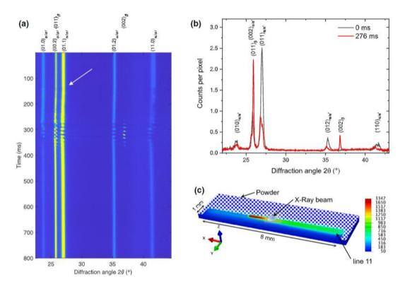
Figure 7.4: (a) variation of phase fraction shown in stacked intensities spectrum taken from the fabrication process of Ti-6Al-4V. (b) Individual spectrums taken before and after a laser hatch being laid. (c) Schematic diagram showing the relative positions of the melt pool, heat affected zone and the Synchrotron X-ray beam [102].
