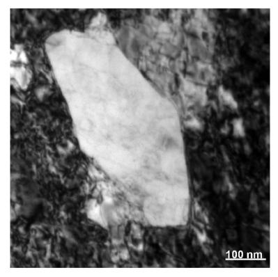
Figure 5.3: Off-axis imaged dislocation cell in additively manufactured M300.
