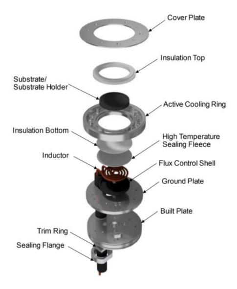
Figure 3.3: Inductive heating element installed in Aconity Lab. The baseplate can be kept at a constant temperature during the build and slowly cooled back down to room temperature after the build.
