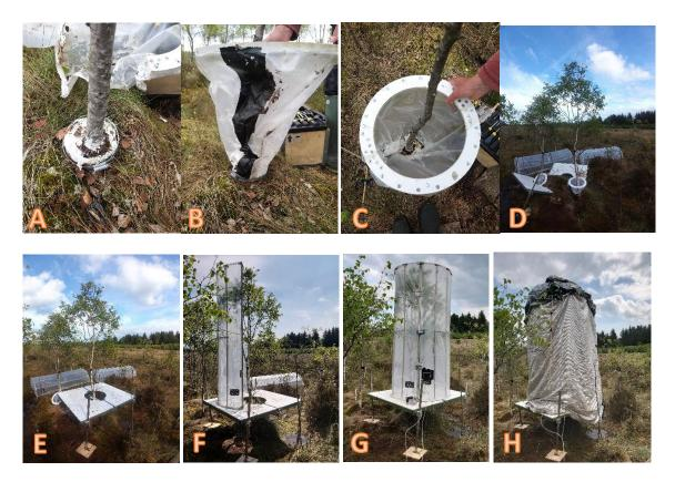
*Figure 5.1*: *a-h*) *Images illustrating the tree chamber systems components and how they assemble.*
