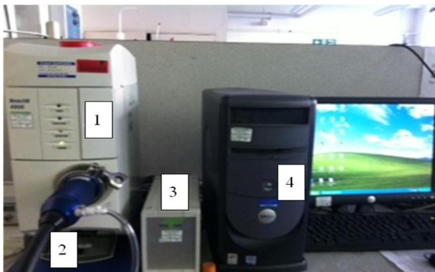
Figure 4.5: The ATR-FTIR instrument ReactIR spectroscopy: 1.MTC-detector; 2.insertion probe; 3. detector module; 4. PC
