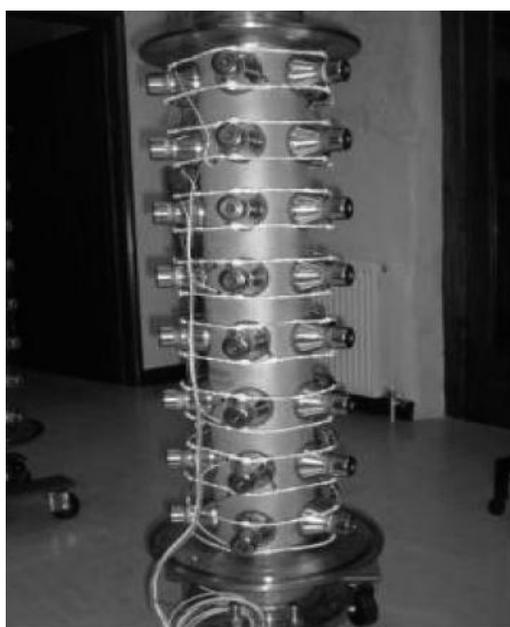
Figure 3.8 20L flow cell fabricated in hard chrome-plated stainless steel with multi-transducers for use in the alumina industry shown with acoustic shield removed for clarity (Ruecroft et al., 2005)
