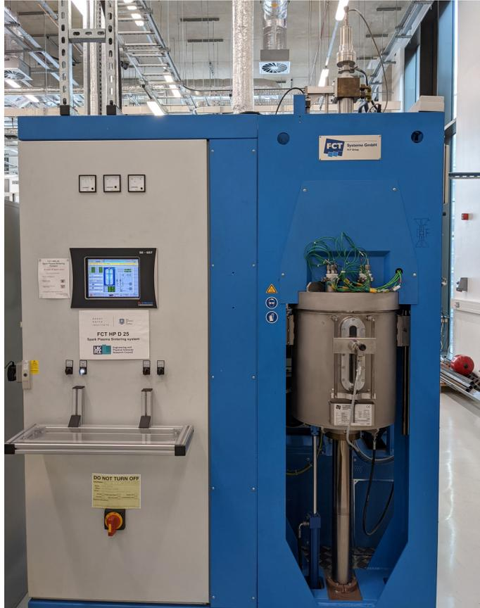
FIGURE 3.2: Photograph of the FCT Systeme GmbH type HP D25 furnace used for all FAST processing.
