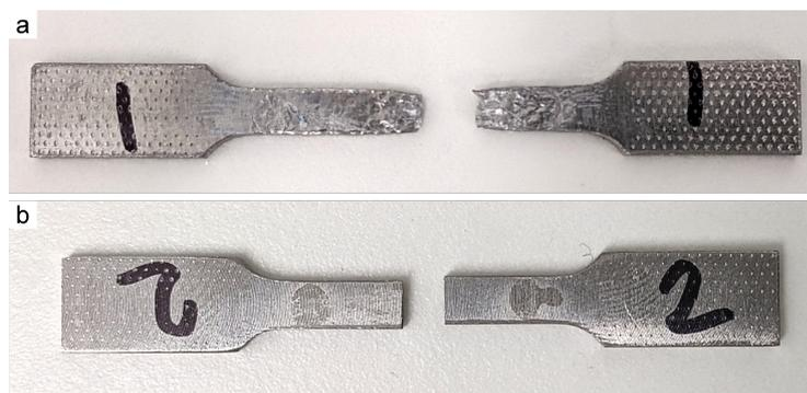
FIGURE 5.22: Photograph of fractured tensile specimens: a) Example of a Beta-C specimen, b) example of a 5.56 wt.% Fe specimen.
