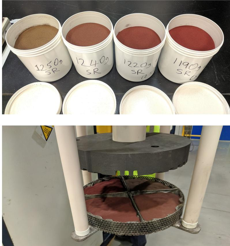
FIGURE 5.14: Top: photograph of SR +  $\text{Fe}_2\text{O}_3$  oxide mixtures after mixing, with increasing red colouration due to higher  $\text{Fe}_2\text{O}_3$  content. Bottom: photograph of oxide mixtures placed in quadrants of steel basket before being placed into reduction cell.
