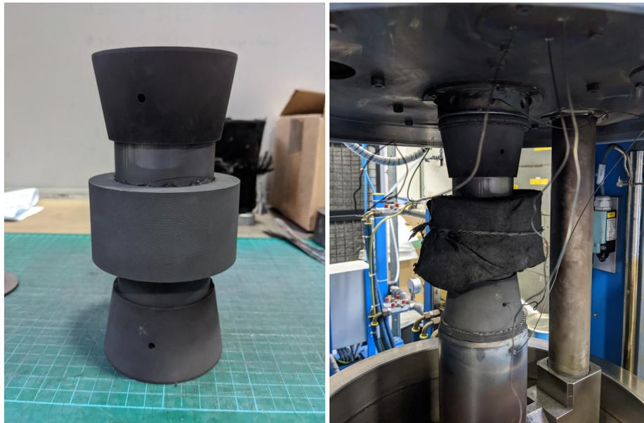
FIGURE 3.4: Left: photograph of assembled tooling (60 mm internal diameter) with supports, right: photograph of assembled tooling placed into the FAST vacuum vessel and covered with a graphite felt jacket.
