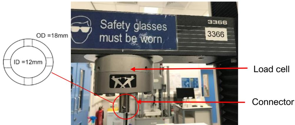
**Figure 6.11 - Attachment mechanism for Instron® 3366 universal testing machine; also showing cross section of connector**
