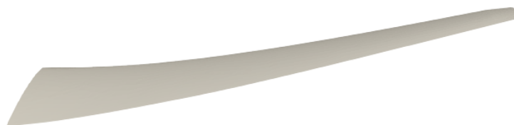
Fig. 1 The converged shape of the LANN wing at a flow condition of Mach 0.73 and a 2° angle of attack.
