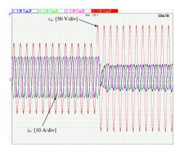
(b) Three-phase instantaneous inverter currents  $(i_{abc})$  and PCC voltage  $(v_a)$  waveforms when the grid fault is cleared
