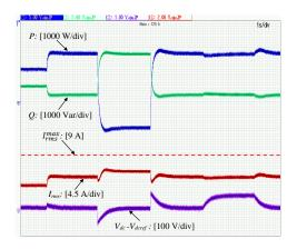
(b) Time response of P, Q,  $I_{rms}$  and  $V_{dc}$  in case of grid frequency swell
