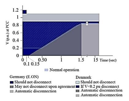
Figure 2.6: FRT curves required by German and Danish grid codes [77].
