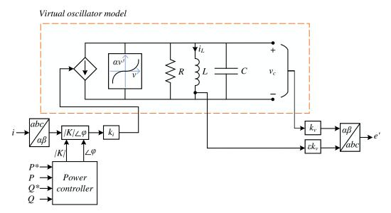
Figure 2.12: Van der Pol oscillator based VOC with active and reactive power regulation capability.
