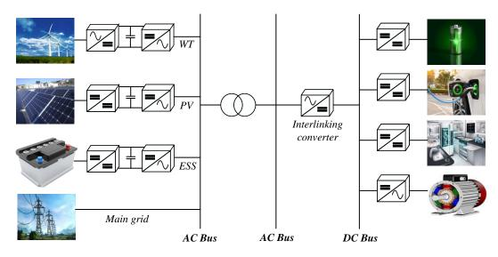
Figure 1.2: A typical example of a microgrid.
