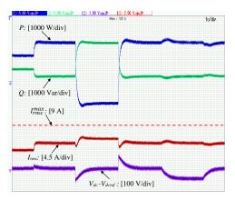
(a) Time response of P, Q,  $I_{rms}$  and  $V_{dc}$  in case of grid frequency drop
