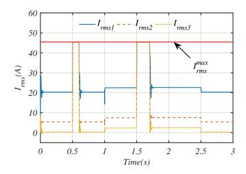
Figure 5.5: RMS currents of three parallel-connected three-phase inverters
