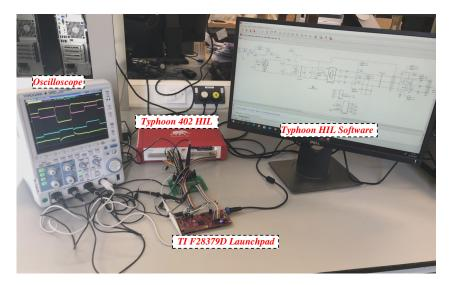
Figure 4.13: HIL experimental setup.
