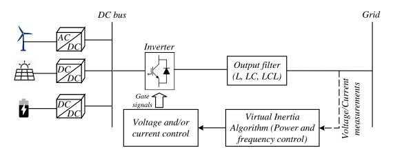
Figure 2.8: Basic virtual inertia concept.
