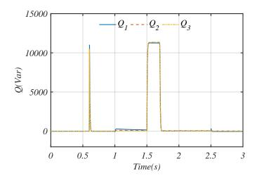
Figure 5.4: Reactive power outputs of three parallel-connected three-phase inverters
