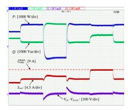
(b) Time response of  $P, Q, I_{rms}$  and  $V_{dc}$  when  $K_D = 3000$  Nms
