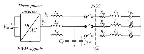
Figure 3.15: Grid-connected three-phase inverter.
