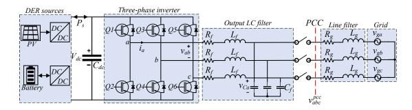
Figure 4.1: DER-sourced grid-connected VSC system
