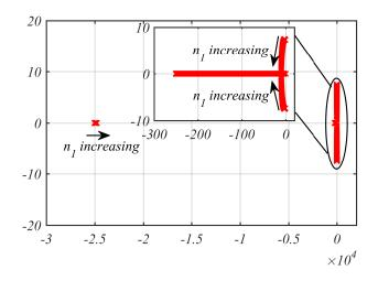
Figure 5.2: Closed-loop eigenvalue spectrum of inverter 1 as a function of active power droop coefficient  $n_1: \frac{0.01\sqrt{2}E^*}{S_{max}} \leq n_1 \leq \frac{0.3\sqrt{2}E^*}{S_{max}}$
