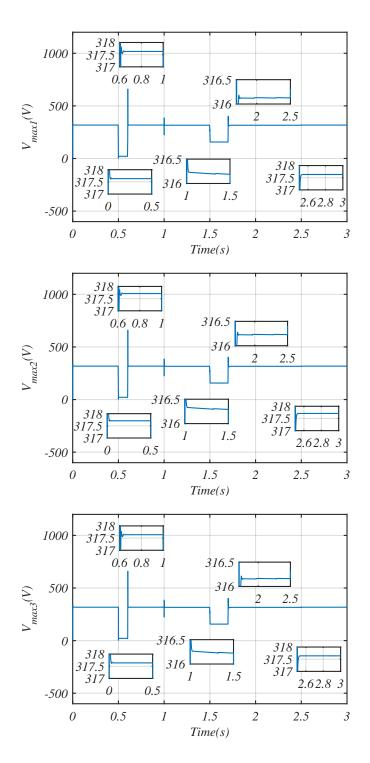
Figure 5.9: The maximum value of the PCC voltages of three parallel-connected three-phase inverters
