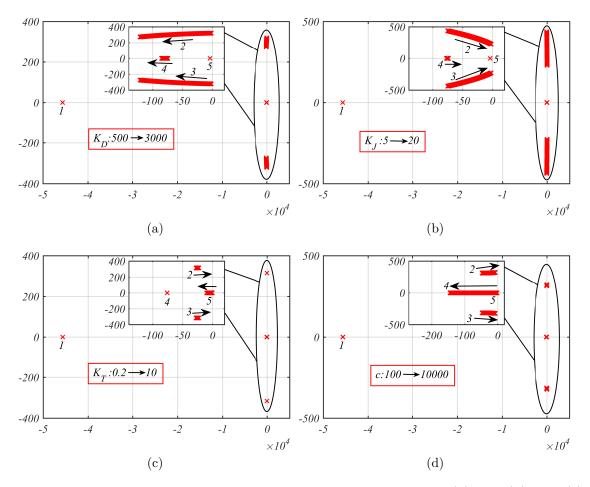
Figure 4.4: Closed-loop eigenvalue spectrum as a function of  $K_D$  (a),  $K_J$  (b),  $K_T$  (c), and c (d).
