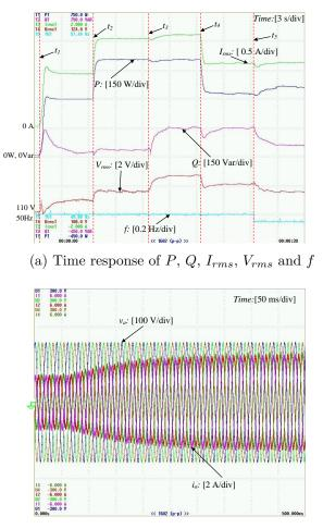
(b) Current transient when  $P_{set}$  is increased from  $300\,W$  to  $750\,W$
