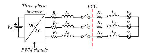
Figure 3.7: Three-phase grid-connected inverter with an L filter.
