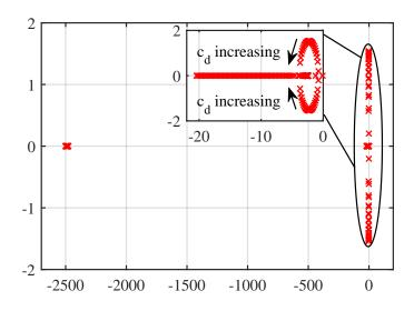
Figure 3.10: Closed-loop system eigenvalues as a function of controller gain  $c_d$  with  $0.1 \le c_d \le 50$
