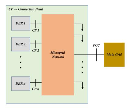
Figure 2.1: A microgrid with several DERs.
