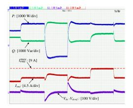
(c) Time response of  $P, Q, I_{rms}$  and  $V_{dc}$  when  $K_D = 5000$  Nms
