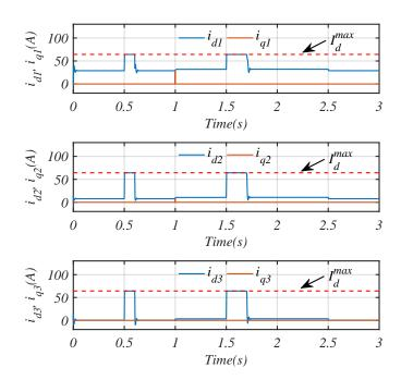
Figure 5.6: dq frame currents of three parallel-connected three-phase inverters
