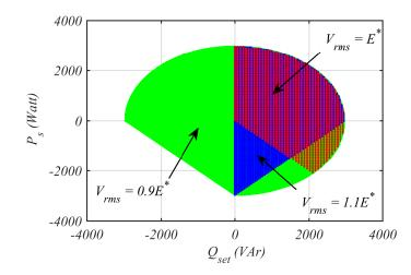
Figure 4.9: Regions for selecting  $P_s$  and  $Q_{set}$  to ensure closed-loop stability.
