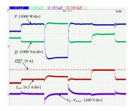
(b) Time response of  $P,\,Q,\,I_{rms}$  and  $V_{dc}$  when  $K_T=4~{\rm Nm}/{\rm V}^2$  and  $K_J=50~{\rm kgm}^2$
