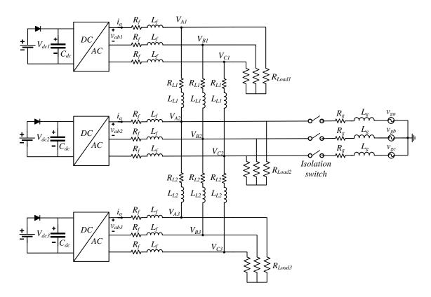
Figure 5.1: The microgrid system under consideration.
