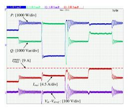
(a) Time response of  $P, Q, I_{rms}$  and  $V_{dc}$  when  $K_D = 3000$  Nms,  $K_J = 200$  kgm<sup>2</sup>, and  $K_T = 10$  Nm/V<sup>2</sup>
