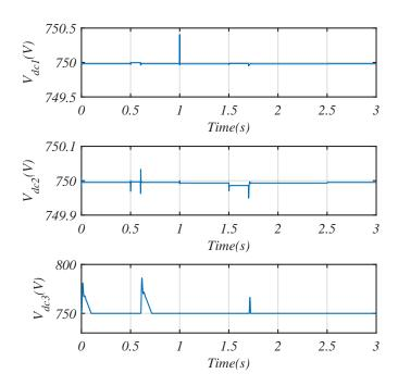
Figure 5.8: DC voltages of three parallel-connected three-phase inverters
