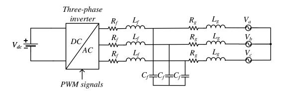
Figure 3.1: Grid-connected three-phase inverter with an LCL filter.
