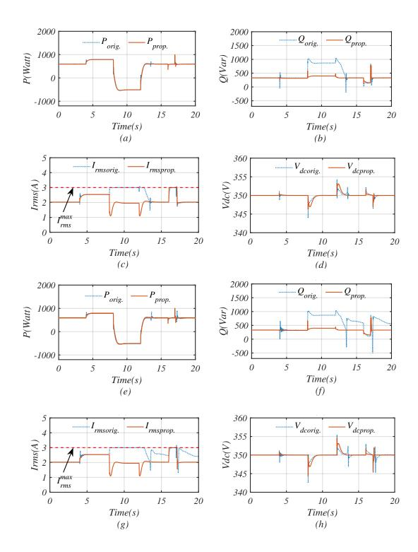
Figure 4.10: Performance comparison of the original [116] and the proposed controller. (a), (b), (c), and (d) with  $K_J = 10 \text{ kgm}^2$ , (e), (f), (g), and (h) with  $K_J = 50 \text{ kgm}^2$ , while  $K_T = 4 \text{ Nm/V}^2$  and  $K_D = 2500 \text{ Nms}$ .
