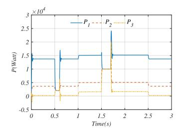
Figure 5.3: Active power outputs of three parallel-connected three-phase inverters
