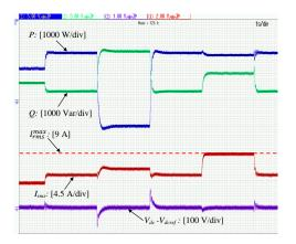
(c) Time response of  $P,\,Q,\,I_{rms}$  and  $V_{dc}$  when  $K_T=10~{\rm Nm/V^2}$  and  $K_J=30~{\rm kgm^2}$
