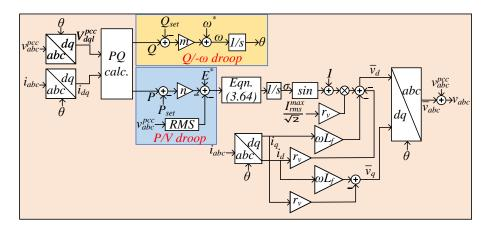
Figure 3.16: Implementation diagram of the proposed controller.
