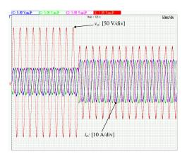
(a) Three-phase instantaneous inverter currents  $(i_{abc})$  and PCC voltage  $(v_a)$  waveforms when the grid fault occurs
