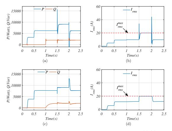
Figure 3.19: Performance comparison between the Benchmark Ctrl 2 (a)-(b) and the Proposed controller (c)-(d) under a 30% balanced grid voltage sag.
