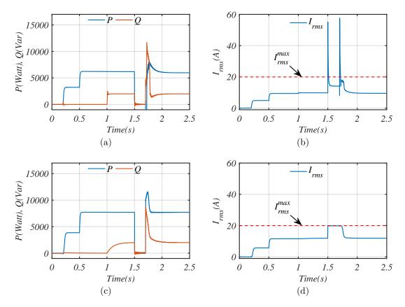
Figure 3.18: Performance comparison between the Benchmark Ctrl 1 (a)-(b) and the Proposed controller (c)-(d) under a three-phase short-circuit fault.
