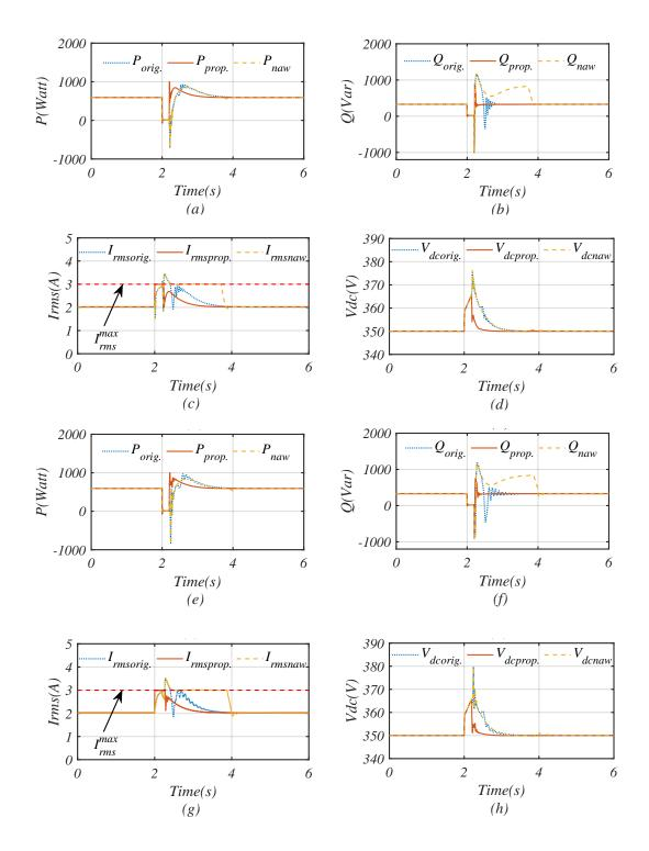
Figure 4.11: Performance comparison of the original [116], with (orig.) and without (naw) anti-windup techniques, and the proposed controller in case of a short-circuit (a), (b), (c), and (d) with  $K_J = 10 \text{ kgm}^2$ , (e), (f), (g), and (h) with  $K_J = 50 \text{ kgm}^2$ , while  $K_T = 4 \text{ Nm/V}^2$  and  $K_D = 2500 \text{ Nms}$ .
