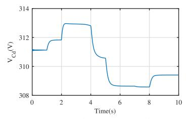
Figure 3.4: *d*-axis capacitor voltage.
