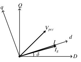
Figure 4.2: Vector diagram of local (dq) and global (DQ) PCC frames.
