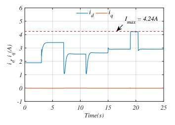
Figure 4.6: Inverter  $i_d$  and  $i_q$  currents.
