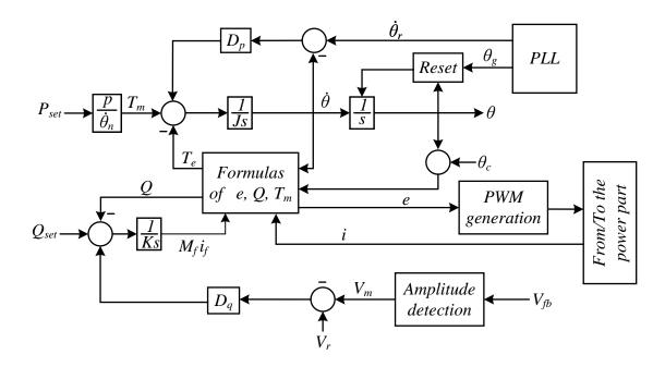
Figure 2.11: Controller stage of synchronverter.
