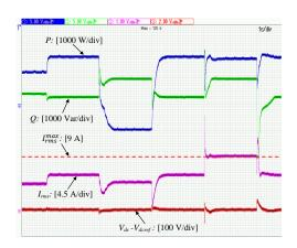
(c) Time response of P, Q,  $I_{rms}$  and  $V_{dc}$  when the reference current saturation method in [26] is used
