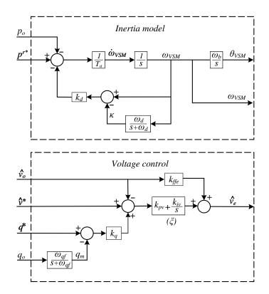
Figure 2.10: VSM inertia model, and voltage controller using reactive power droop.
