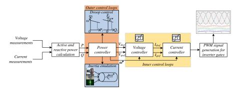
Figure 2.16: Commonly used cascaded inverter control scheme.
