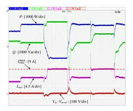
(b) Time response of P, Q,  $I_{rms}$  and  $V_{dc}$  when the d-axis priority based-current saturation algorithm in [123] is used
