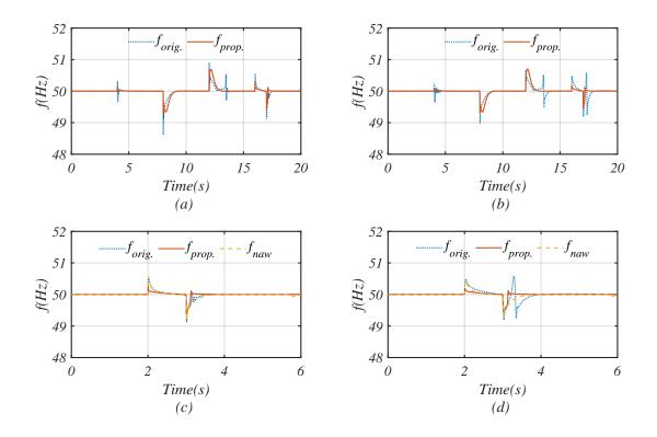
Figure 4.12: Frequency comparison of the original [116], with (orig.) and without (naw) anti-windup techniques, and the proposed controller in case of entire scenario (a) with  $K_J = 10 \text{ kgm}^2$  (b) with  $K_J = 50 \text{ kgm}^2$ , and in case of a 40% balanced grid fault (c) with  $K_J = 10 \text{ kgm}^2$  (d) with  $K_J = 50 \text{ kgm}^2$ , while  $K_T = 4 \text{ Nm/V}^2$  and  $K_D = 2500 \text{ Nms}$ .
