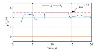
Figure 3.13: d- and q-axis currents.
