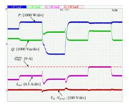
(a) Time response of P, Q,  $I_{rms}$  and  $V_{dc}$  when the proposed controller is used
