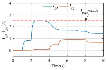
Figure 3.3: *d*- and *q*-axis grid currents.
