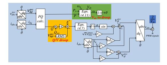
Figure 4.3: Implementation diagram of the proposed controller integrated with the ViSynC.
