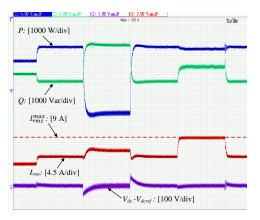
(a) Time response of  $P, Q, I_{rms}$  and  $V_{dc}$  when  $K_D = 2000$  Nms
