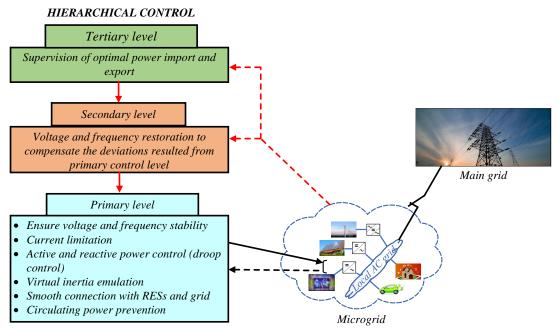
Figure 2.5: Hierarchical control layers in future power systems.
