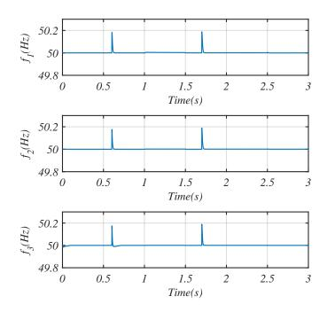
Figure 5.7: Frequencies of three parallel-connected three-phase inverters
