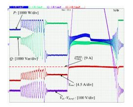
(b) Time response of  $P, Q, I_{rms}$  and  $V_{dc}$  when  $K_D = 3000$  Nms,  $K_J = 200$  kgm<sup>2</sup>, and  $K_T = 20$  Nm/V<sup>2</sup>
