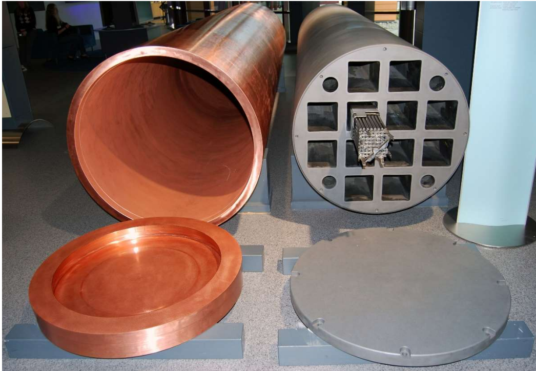
Figure 4: KBS-3 HLW GDF cask design, showing the multi-layer structure of the proposed cask. Zircaloy-clad spent fuel bundles are held within cast iron canisters (right), which are in turn encapsulated in copper canisters (right).
