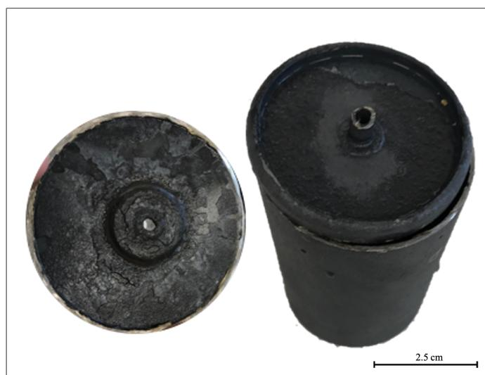
Figure 4.7: Scaling observed in 316 stainless steel canisters.
