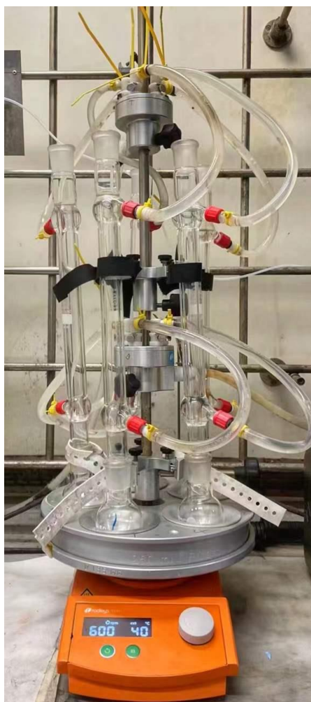
Fig. 2.2 The reactor apparatus for the test at atmospheric pressure with water reflux condenser open to air.
