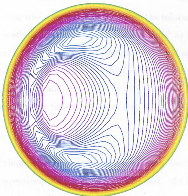
Figure 6.13: Film thickness contour at time t = 3.0 .
