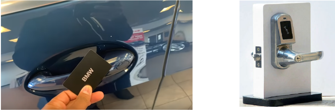
Figure 5.2: Some security applications of NFC technology. Commercial products like a security safe lock with an NFC system opening key. A BMW door opening and NFC house handle. The image was taken from a car shop in the United Kingdom and the web source [258].
