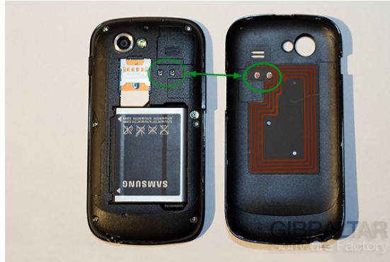
Figure 3.4: Samsung NEXUS S, the first NFC-enabled Android phone, open in the back where the NFC coil can be clearly noticed[155].
