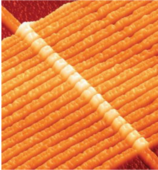
Figure 4.2: The memristor as seen via a scanning tunnelling microscope [225].
