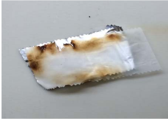
Figure 2.28: FOD to a chew-gum aluminium wrap which have begun to burn.
