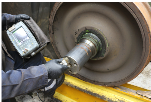
(a) Ultrasonic inspection
