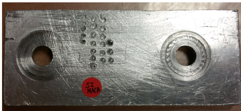
Figure 3.13: Test sample for replicating compounds, with a series of micro holes drilled into a section of scrap metal
