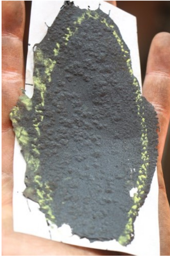
Figure 3.22: Example of a cast of a region of corrosion from a rail axle
