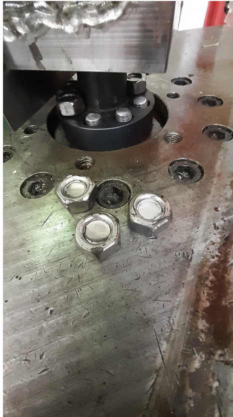
Figure 5.39: Fatigue failure of threaded bar machine assembly interface
