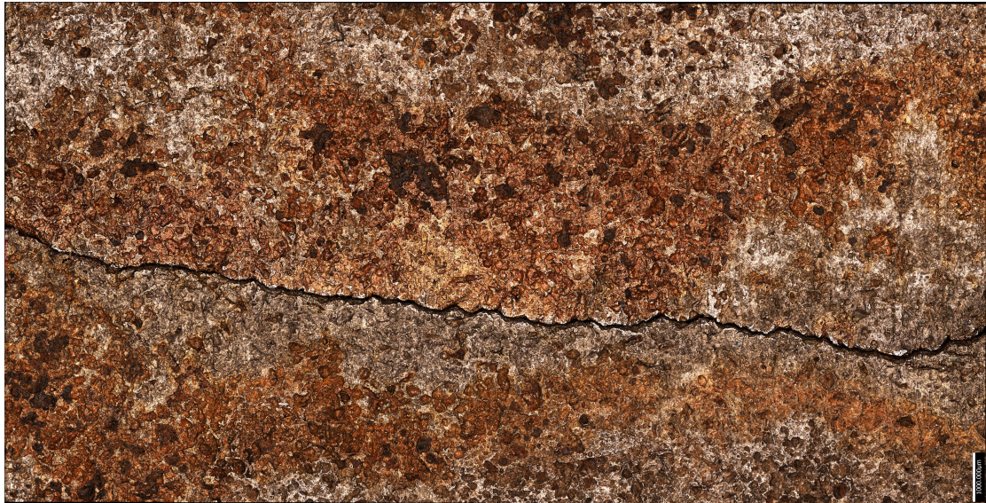
Figure 6.9: Optical image of the crack in the 12 month section of the sample. Taken using the Alicona Machine
