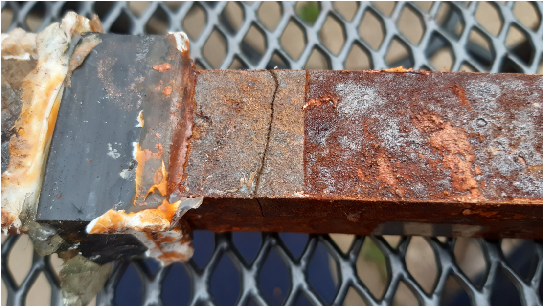
Figure 5.57: Crack that developed in one of the samples that contained the original axle surface
