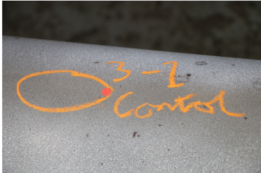
Figure 2.21: Example of an axle that has undergone shot blasting, but exhibits no other surface damage
