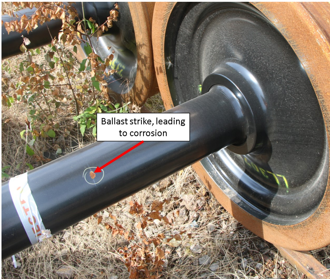
Figure 2.9: Damage to the paint layer of an axle due to a ballast strike. Corrosion has already taken place in the unprotected areas
