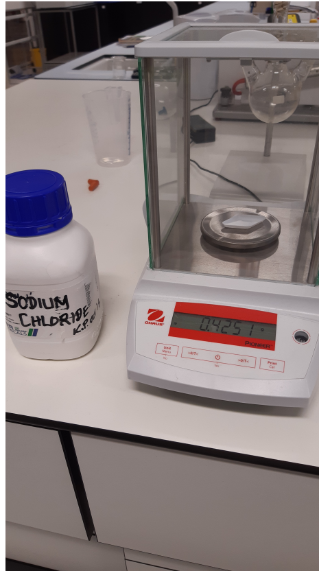
Figure 5.27: Equipment used to weigh out salts before being added to the artificial rainwater mixture
