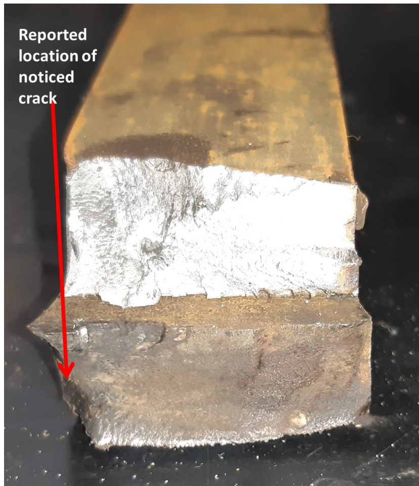
Figure 5.41: Close-up of upper fracture location
