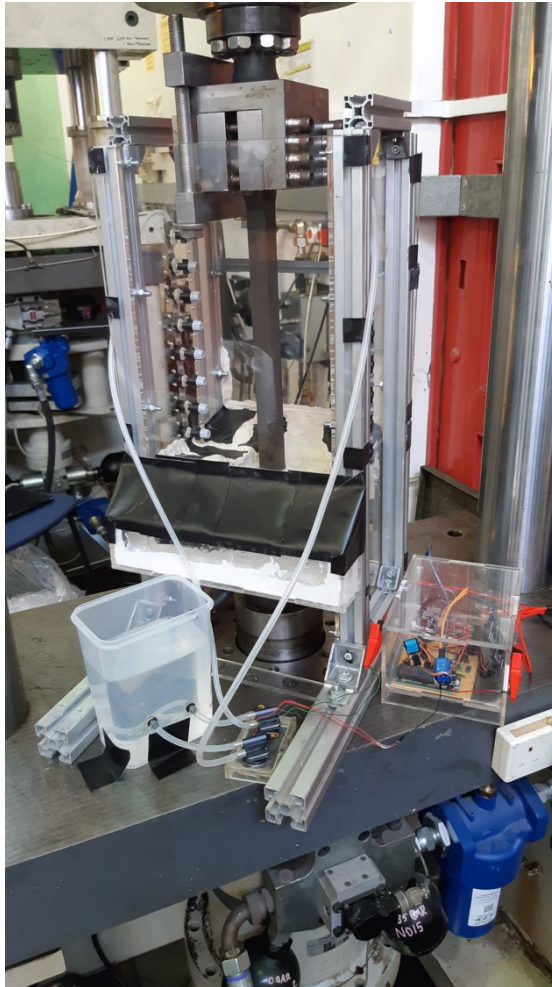
Figure 5.29: Image of the corrosion chamber used to contain the corrosive medium during the experiment. Corrosion chamber has been assembled within larger rig (white material removed before testing)
