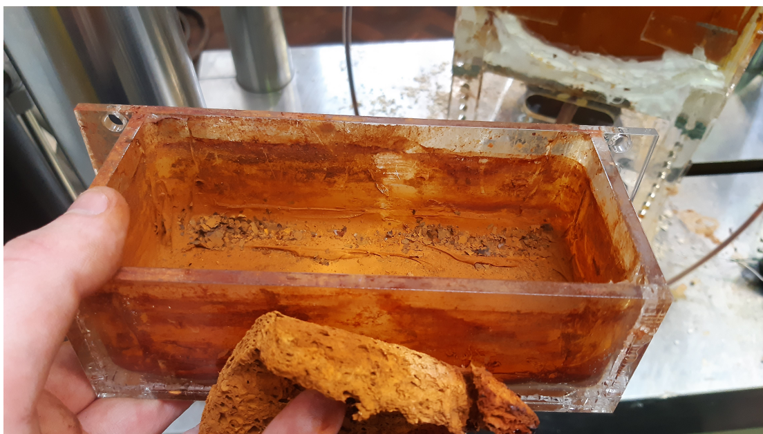
Figure 5.62: Larger sections of corrosion product that settled in the reservoirs, requiring the addition of a sponge to separate the outlets and inlets to prevent damaging the pumps
