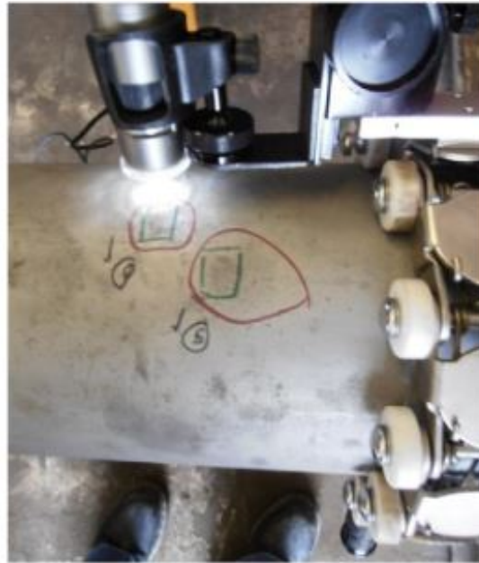
Figure 3.5: Optical approach for assessing corrosion pits [36]
