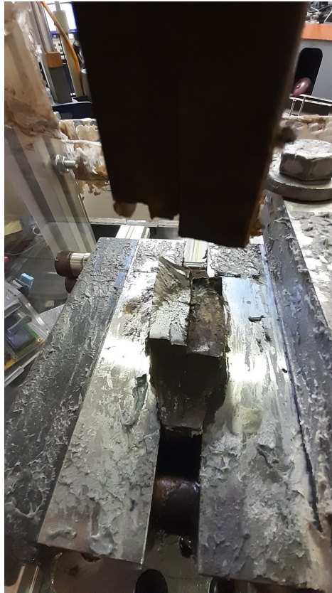
Figure 5.38: View of lower fracture surface showing debris in the dull fracture surface
