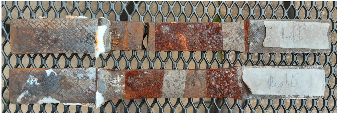
Figure 6.6: Image of the curved samples after having tape removed but before cleaning. Note the areas of reduced corrosion and the crack in the upper ("broken") sample.
