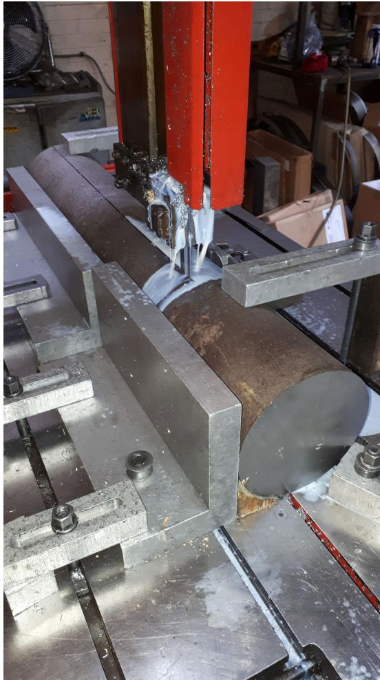
Figure 5.49: Cutting of the axle to produce the material used in the bright samples
