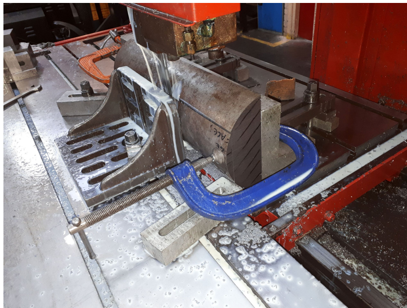
Figure 5.21: Cutting of the sample blanks from the original axle
