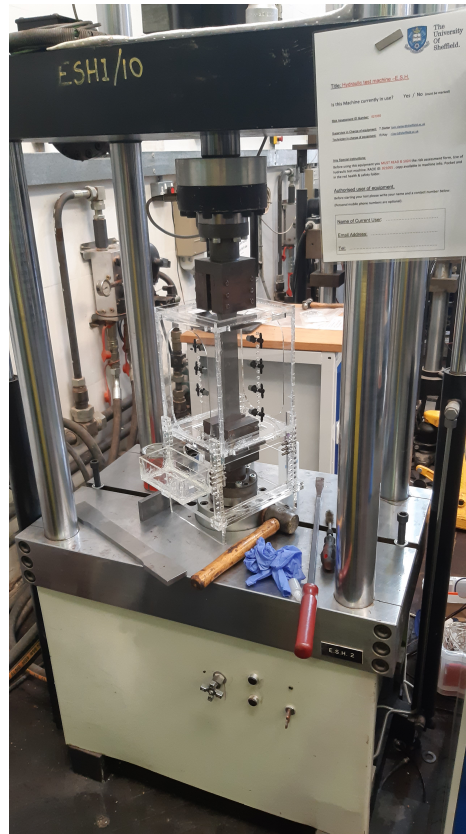
Figure 5.48: Image of the E.S.H. rig, with the jaws and sample fitted and the corrosion chamber under construction
