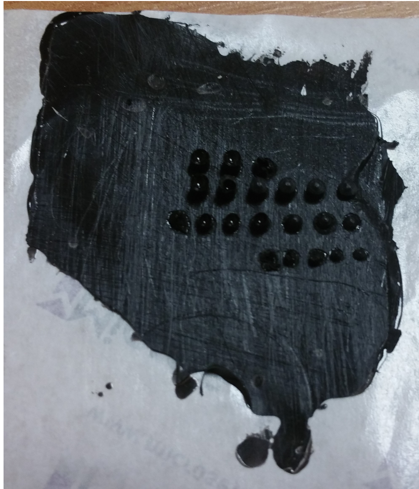
Figure 3.14: Example of a cast taken from the test sample using 101FF. Evidence of the air trapping issue can be seen at the tips of some of the columns
