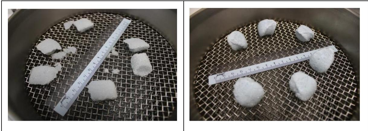
**Figure 5.8** Ballotini 10cSt pellets flattened/fragmented (left) and lactose 10cSt pellets elongated (right)
