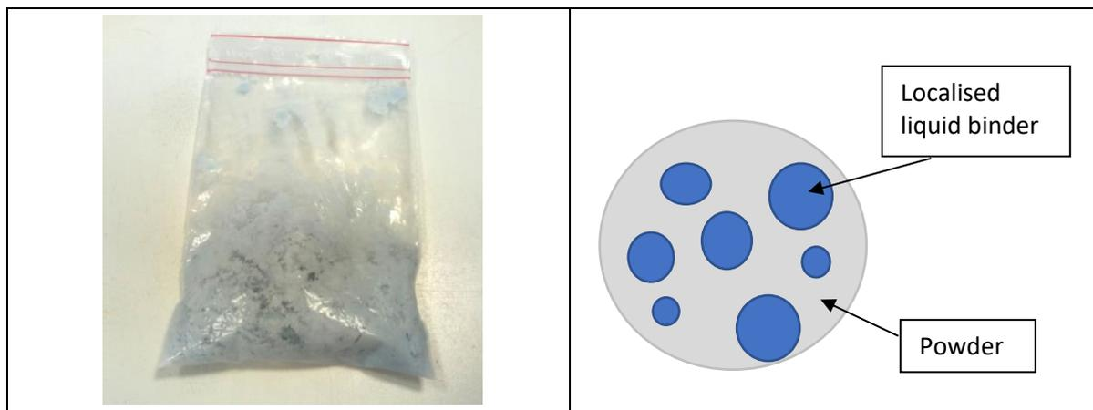
**Figure 3.10 Hand-kneading the mixture in a plastic bag (left) and localization of liquid binder within powders (right)**
