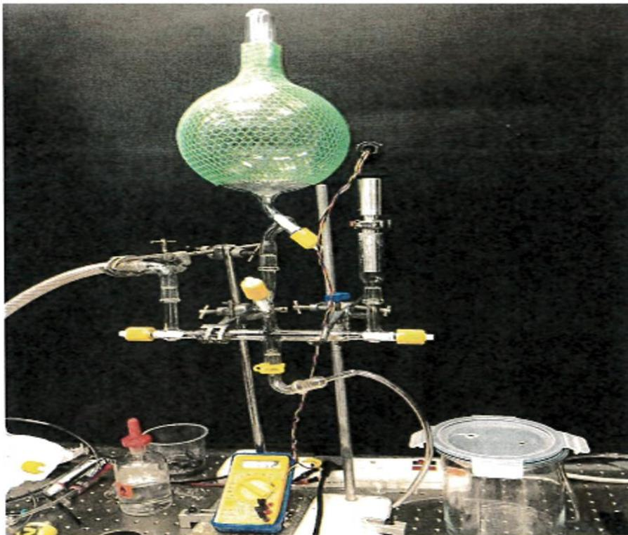
**Figure 2.10.** Experimental setup used to transfer  $C_2H_2$  into the White Cell for pathlength determination.
