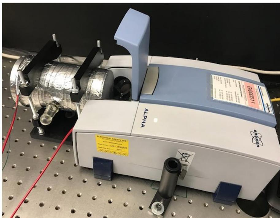
**Figure 2.11.** The commercial FTIR spectrometer attached to the home built White cell.
