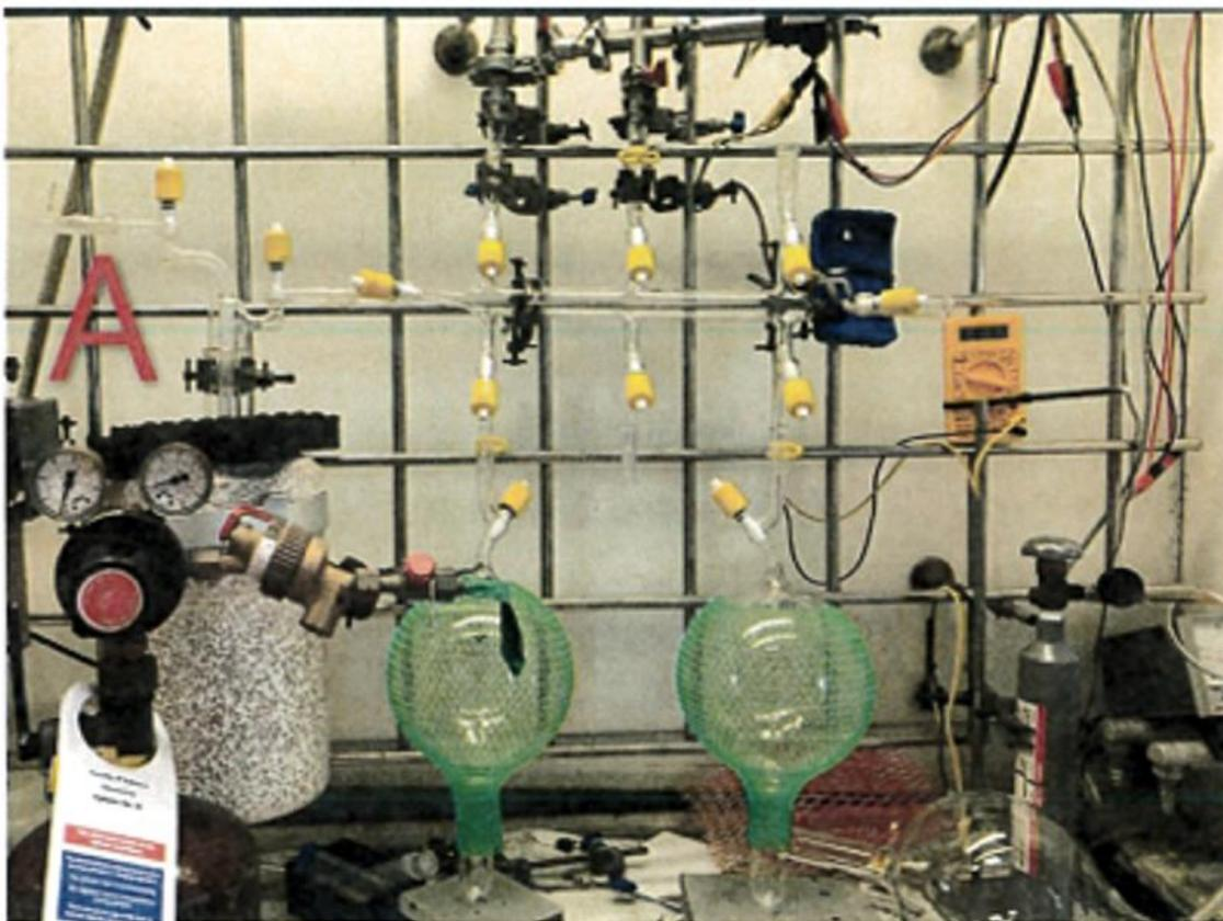
**Figure 2.8.** Gas handling line used to purify  $C_2H_2$  and introduce it with a defined pressure into the White Cell for pathlength determination.
