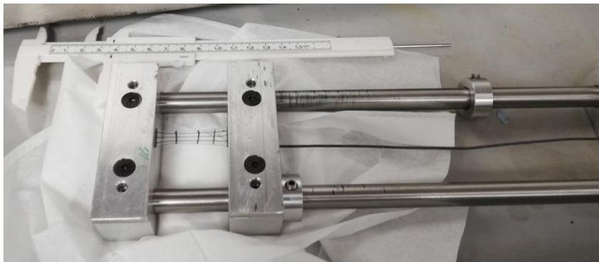
*Figure 2-1: Custom built stretching equipment for ellipsoid preparation.*
